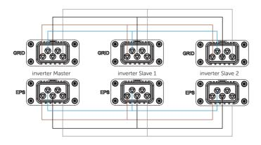
Figure 15-20 Power cable connection without X3-Parallel EPS BOX
