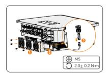
Figure 12-1 Disconnect the fans connectors
