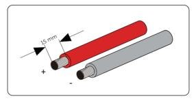
Figure 8-26 Striping the battery cable
