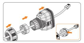
Figure 8-41 Threading the cables
