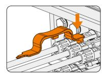
Figure 13-2 Releasing the PV connector
