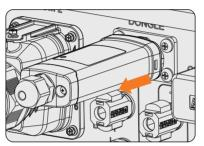
Figure 13-3 Removing the dongle
