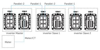
Figure 15-22 Communication connection without X3-Parallel EPS BOX
