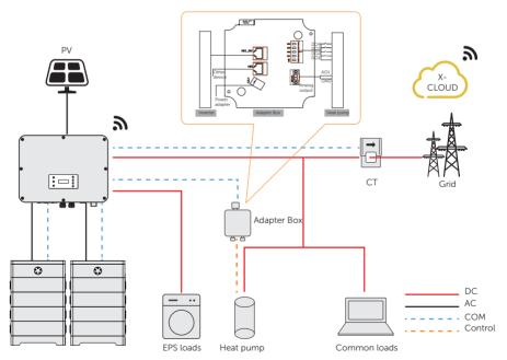
Figure 15-4 Adapter Box wiring diagram
