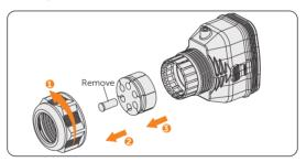
Figure 8-49 Disassembling the connector
