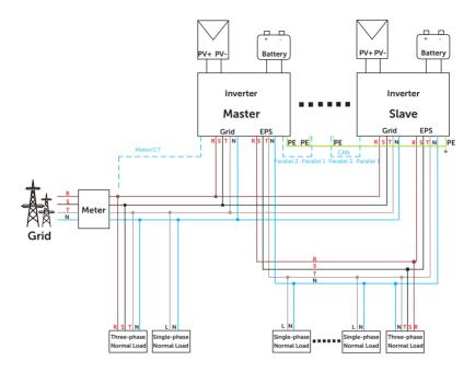
Figure 15-18 System diagram without SolaX X3-Parallel EPS BOX
