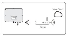
Figure 8-61 Wi-Fi mode connection diagram
