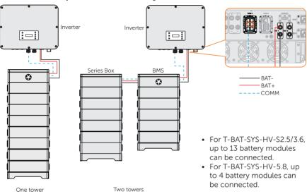
Figure 8-22 Battery connection in one string
