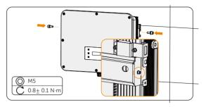
Figure 7-10 Securing the inverter
