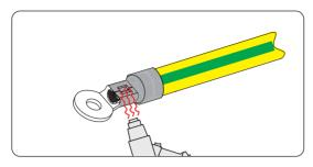
Figure 8-5 shrinking the tubing
