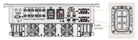
Figure 15-5 Connection terminal for Adapter Box
