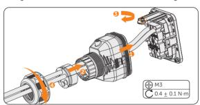
Figure 8-37 Securing the connector
