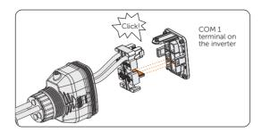
Figure 8-36 Inserting the connector to COM 1
