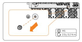
Figure 8-6 Uninstalling the screw
