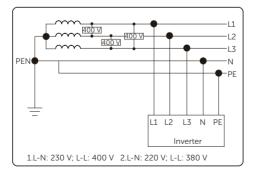
Figure 2-4 Supported power grid-TN-C-S
