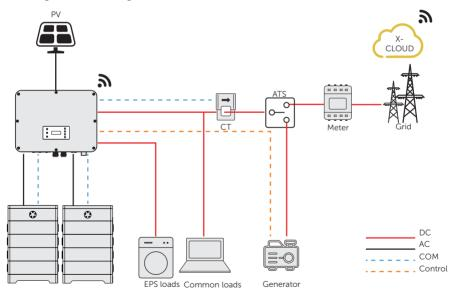
Figure 15-2 Dry contact wiring diagram
