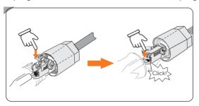
Figure 8-29 Press down on the Spring
