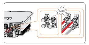
Figure 8-31 Connecting the battery connector
