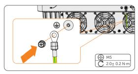
Figure 8-7 Securing the PE cable
