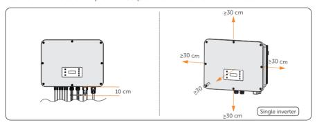
Figure 5-4 Clearance requirement for single inverter
