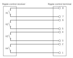
Figure 8-54 Connection diagram for ripple control
