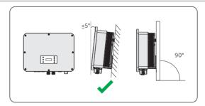
Figure 7-1 Correct installtion
