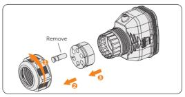
Figure 8-55 Disassembling the connector
