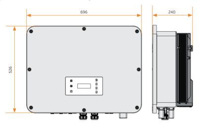
Figure 7-3 Dimensions 1 (Unit: mm)
