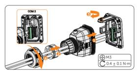
Figure 8-57 Connecting to the inverter
