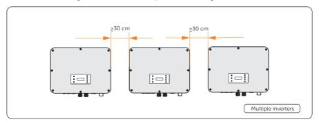
Figure 5-5 Clearance requirement for multiple inverter
