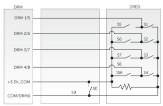
Figure 8-43 DRED wiring diagram
