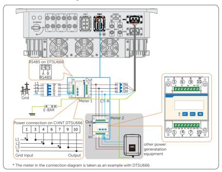
Figure 8-45 Meter connection diagram
