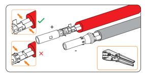
Figure 8-17 Crimping the terminal
