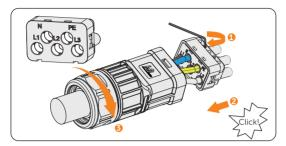
Figure 8-12 Assembling the AC connector
