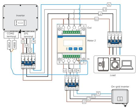
Figure 15-16 Connection diagram of Meter on EPS terminal
