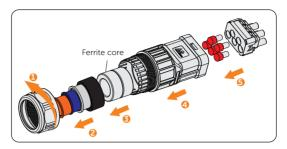
Figure 8-9 Disassembling the AC connector
