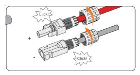
Figure 8-19 Securing the PV cable
