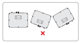
Figure 7-2 Incorrect installation
