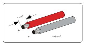
Figure 8-15 Striping the PV cable
