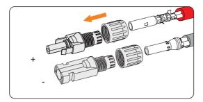
Figure 8-18 Threading the PV cable
