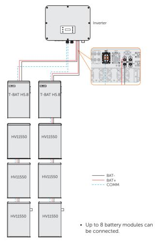
Figure 8-24 Battery connection in two strings (T-BAT-SYS-HV-5.8)
