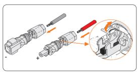
Figure 8-27 Opening the spring
