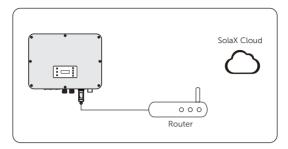
Figure 8-62 LAN mode connection diagram
