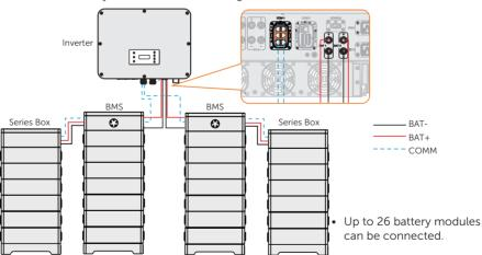
Figure 8-23 Battery connection in two strings (T-BAT-SYS-HV-S2.5/3.6)
