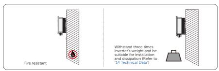
Figure 5-3 Installation carrier requirement
