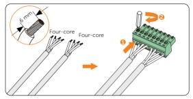
Figure 8-56 Connecting to 8-pin terminal block
