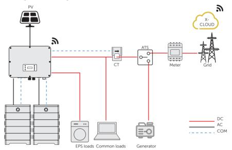
Figure 15-1 ATS control wiring diagram
