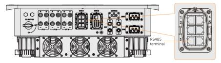
Figure 15-8 Connection terminal for EV-Charger
