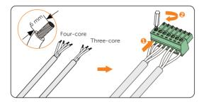
Figure 8-59 Connecting to 7-pin terminal block
