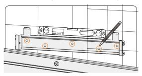
Figure 7-5 Marking the holes
