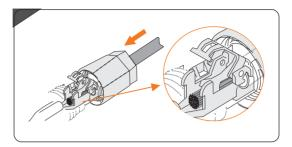
Figure 8-28 Threading the battery cable
