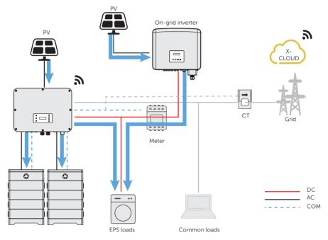
Figure 15-15 Power flowing when grid off
