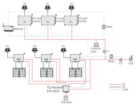
Figure 15-10 Datahub wiring diagram
