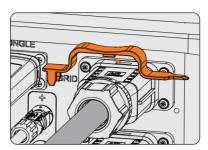
Figure 13-5 Removing AC connector
