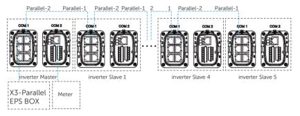
Figure 15-21 Communication connection with X3-Parallel EPS BOX
