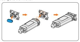
Figure 8-64 Wi-Fi connection procedure
