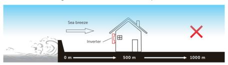
Figure 5-2 Incorrect installation position
