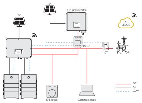
Figure 15-13 Micro-grid wiring connection
