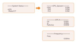
Meter/CT status: Information contains feed-in power of L1, L2 and L3 detected by the connected meter or CT. "+" represents feeding electricity to the grid, "-" represents drawing electricity from the grid (buying electricity).
