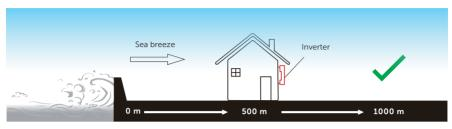
Figure 5-1 Recommended installation position
