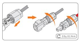
Figure 8-30 Tighten the cable gland
