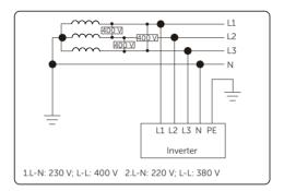
Figure 2-2 Supported power grid-TT
