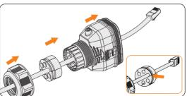
Figure 8-50 Threading the cables
