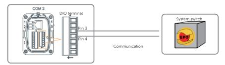
Figure 8-58 System switch connection diagram
