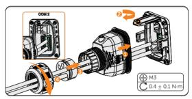
Figure 8-60 Connecting to the inverter
