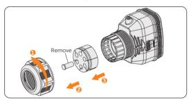
Figure 8-40 Disassembling the connector
