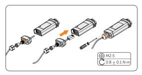
Figure 8-66 Assembling the dongle
