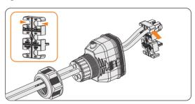
Figure 8-35 Installing RJ45 terminal to the cable fixture
