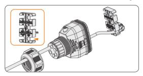
Figure 8-44 Installing RJ45 terminal to the cable fixture
