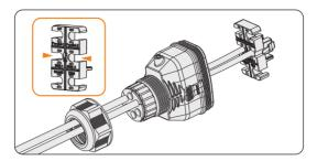
Figure 8-39 Installing RJ45 terminal to the cable fixture
