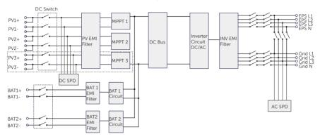
Figure 2-5 Circuit Diagram for X3-ULTRA series inverter
