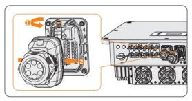
Figure 8-48 Disassembling the COM 2 terminal
