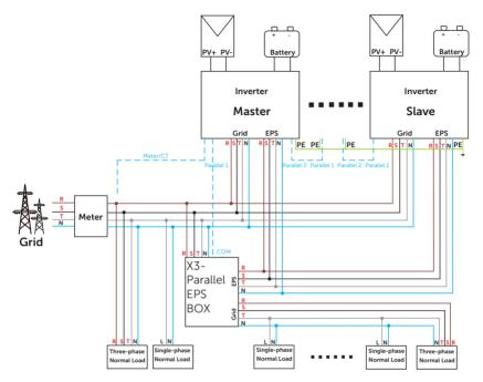
Figure 15-17 System diagram with SolaX X3-Parallel EPS BOX
