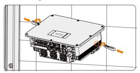
Figure 7-8 Install the handles
