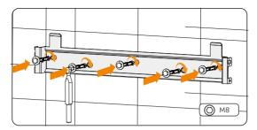
Figure 7-7 Inserting the screws
