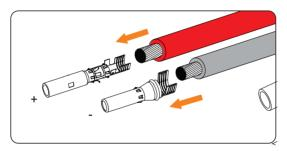
Figure 8-16 Inserting the PV pin contact
