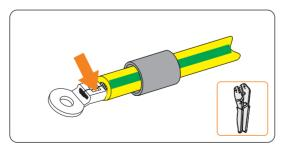
Figure 8-4 Crimping the cable
