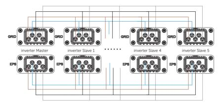
Figure 15-19 Power cable connection with X3-Parallel EPS BOX
