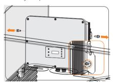
Figure 13-6 Unscrewing the M5 screws
