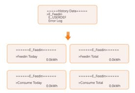
E\_USERDEF: The electricity of the connected on-grid inverter totay and the total.(detected by Meter 2) This function is only available when the meter 2 is connected.
