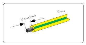
Figure 8-2 Striping the PE cable
