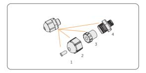
Figure 8-65 Disassembling the waterproof connector
