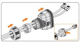
Figure 8-34 Threading the cables
