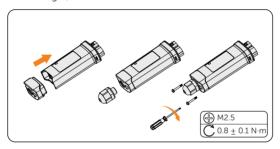
Figure 8-63 Assembling the dongle
