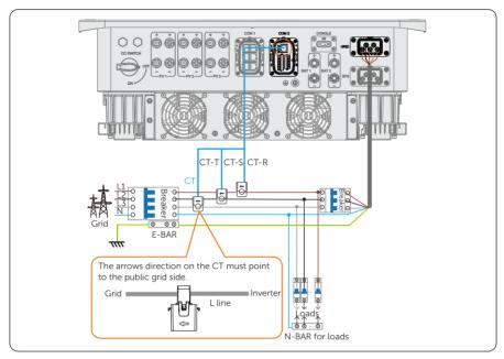
Figure 8-46 CT connection diagram
