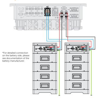
Figure 8-38 BMS connection diagram
