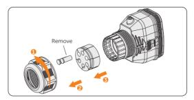
Figure 8-33 Disassembling the connector
