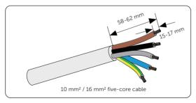
Figure 8-8 Striping the Grid cable
