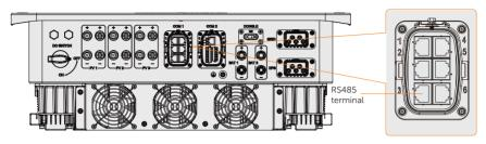
Figure 15-11 Connectiong terminal for Datahub
