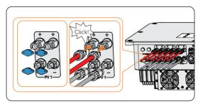
Figure 8-21 Connecting the PV cable
