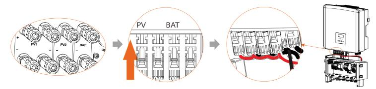
\*\*Note: 5.0 kw and 6.0 kw M series inverter have only two MPPT and two PV strings, so when connecting, you need to unplug ①/② of the PV in the X3-Matebox basic.
