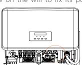
c) Use the inner hexagonal wrench to tighten the inner hexagonal screw on the right side of the inverter.
