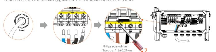
4) Pass the PV /Grid line through the PV port of the X3-MateBox basic, and then find PV (PV1+/PV1-/PV2+/PV2+) and Grid (N/R/S/T) port inside the X3-Matebox basic. Force the cable harness directly into the hole to jam, gently twist not to loosen.
