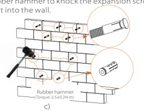
inner hexagonal wrench to screw the tapping screw until the expansion bolt "bang" is heard.
