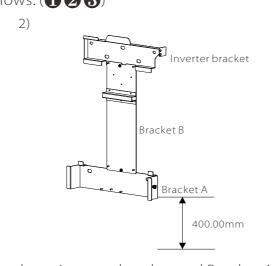
Note: When brackets are mounted, a spirit level is used to keep inverter bracket and Bracket A parallel to the ground.
