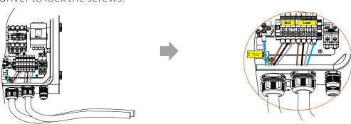
5) Pass the battery power wire through the BAT port of The X3-Matebox advanced, then find the BAT+ and BAT- ports in the X3-Matebox advanced, insert each wire accordingly, and use the screwdriver to lock the screws.
