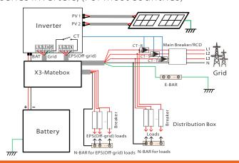
Diagram B: N line and PE line together, M series inverters: (Applicable to Australia)
