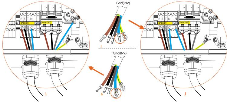
Note: According to the different N terminals of Grid(INV), select the corresponding connection position.(if need:(A + 6.4B) or (I + 6.4II))
