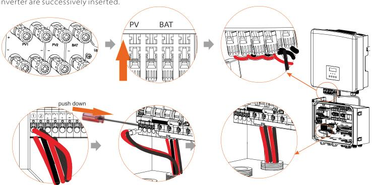
Note: 5.0 kw and 6.0kw M. series inverters have only two MPPT and two PV strings, so when connecting, you need to unplug 1/2 of the PV in the X3-Matebox advanced.
