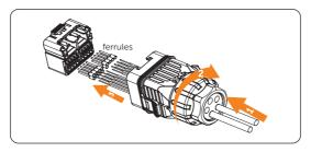
Figure 7-59 Inserting wires into ferrules
