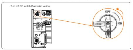
Figure 8-7 Turning off DC switch
