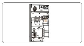
Figure 7-30 Removing the dustproof cover
