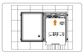
Figure 7-138 Reinstalling the plate
