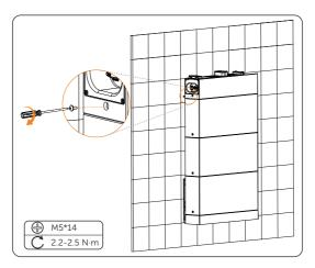
Figure 6-48 Tightening M5 screws
