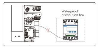
Figure 14-8 Connecting inverter to meter
