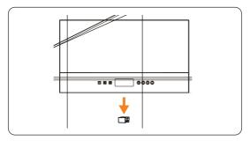
Figure 6-50 Removing the dustproof cover
