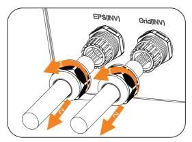
Figure 12-19 Disassembling EPS(INV) and Grid(INV) cables
