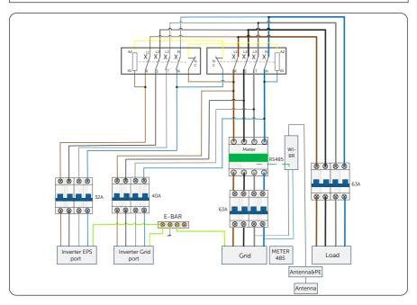
Figure 7-95 Matebox wiring diagram (with Wi-BR)
