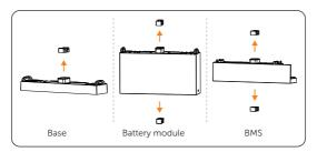
Figure 6-31 Removing dust covers
