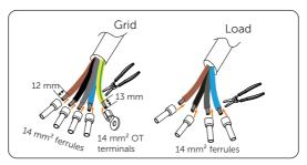
Figure 7-126 Assembling the Grid annd Load cable
