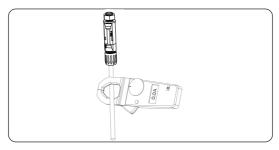
Figure 12-4 Detecting the current
