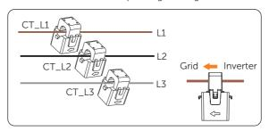
Figure 14-2 Clipping CTs to grid cables
