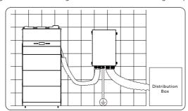
Figure 7-135 Connecting the Grid and Load cables
