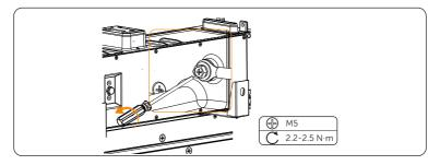
Figure 12-18 Disconnecting grounding cable
