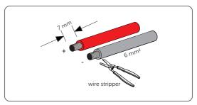
Figure 7-36 Stripping PV cables
