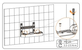
Figure 6-36 Securing the base
