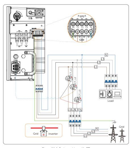
Figure 14-1 System wiring with CT
