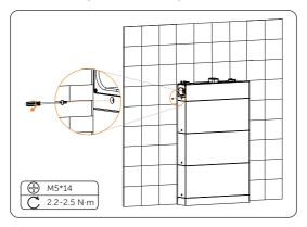
Figure 6-23 Tightening M5 screws
