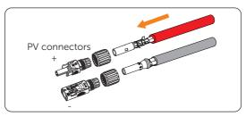
Figure 7-39 Threading PV cables with PV pin contacts connected
