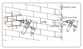
Figure 6-9 Drilling holes
