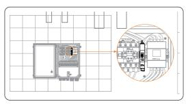
Figure 7-92 Installing the Wi-BR
