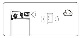
Figure 7-77 WiFi+4G connection diagram
