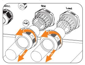
Figure 12-20 Disassembling Grid and Load cables
