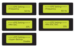
Figure 9-69 Setting data in EPS setting
