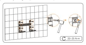
Figure 6-35 Tightening expansion screws
