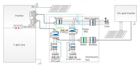
Figure 2-29 Micro grid system diagram
