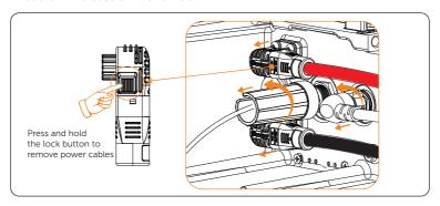
Figure 12-17 Disconnecting battery connectors
