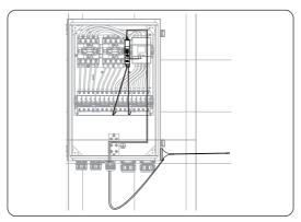
Figure 7-94 Connecting the Wi-BR and antenna
