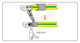
Figure 7-17 Crimping the cable
