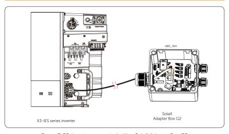
Figure 7-53 Inverter connected with a SolaX Adapter Box G2
