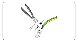
Figure 7-113 Stripping the PE cable
