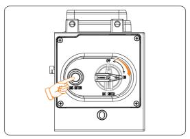
Figure 8-3 Turning on the battery
