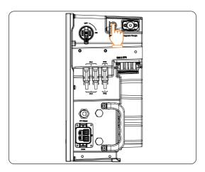
Figure 8-4 Pressing the inverter button
