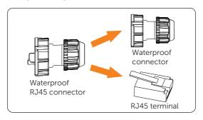
Figure 7-63 Disassembling the waterproof RJ45 connector
