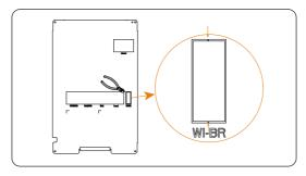
Figure 7-96 Cutting the baffle
