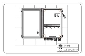
Figure 7-137 Securing the plate
