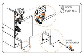
Figure 7-70 Locking the cable shielding board
