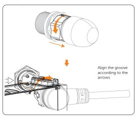
Figure 7-12 Locking heater cable
