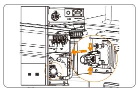
Figure 12-14 Disconnecting the communication connector
