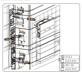
Figure 6-53 Locking the inverter brackets
