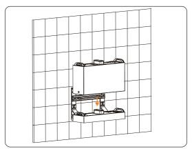
Figure 6-37 Placing battery module
