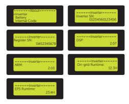
Figure 9-103 Displaying the inverter information
