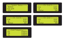
Figure 9-16 Displaying on-grid status
