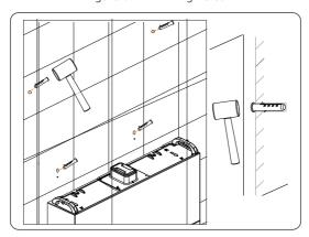
Figure 6-45 Knocking expansion tubes into the wall
