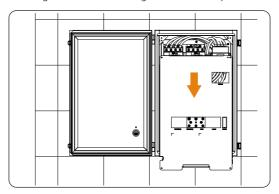
Figure 7-90 Removing the plate
