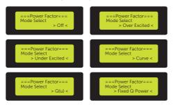
Figure 9-52 Selecting a mode in power factor
