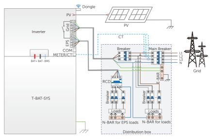
Figure 2-25 System diagram without X3-Matebox G2 for most countries
