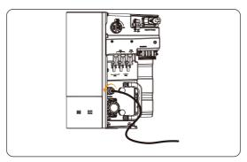
Figure 12-15 Disconnecting the CT/Meter cable
