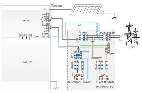
Figure 2-27 System diagram without X3-Matebox G2 for Australia
