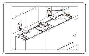
Figure 6-41 Marking the position of BMS
