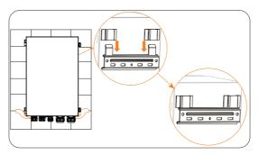
Figure 6-60 Hanging the matebox on the bracket
