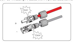
Figure 7-40 Securing PV cables
