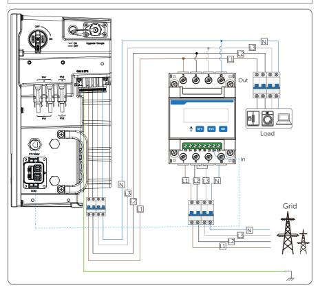
Figure 14-5 System wiring with direct-connected meter
