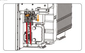
Figure 12-8 Pulling out PV dustproof buckles
