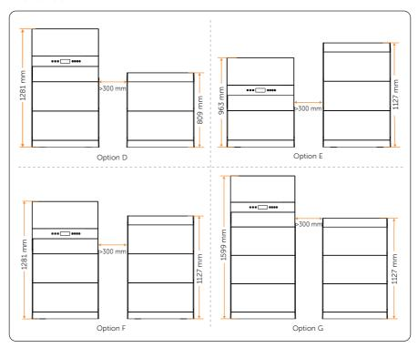
Figure 4-4 Installation options for two towers
