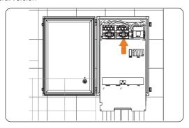
Figure 7-136 Reinstalling the plate
