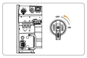
Figure 12-2 Turning off the DC switch
