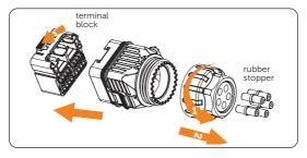
Figure 7-55 Disassembling the communication connector
