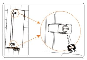
Figure 7-86 Unlocking the buckles
