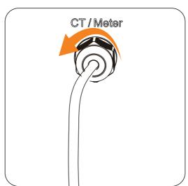
Step 22: Disassemble the CT/Meter cable in the X3-Matebox G2.
