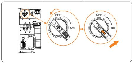
Figure 8-8 Locking DC switch
