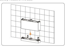
Figure 6-12 Placing the battery module
