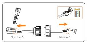
Figure 7-66 Crimping the communication cable for CT
