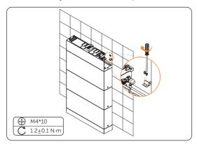
Figure 6-24 Install the anti-tamper bracket
