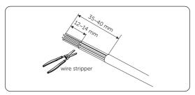
Figure 7-58 Stripping cables
