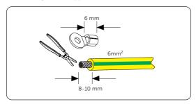
Figure 7-15 Striping the PE cable
