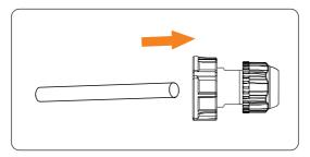
Figure 7-64 Threading the communication cable
