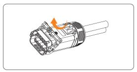
Figure 7-29 Pulling up the latch
