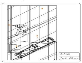
Figure 6-19 Drilling holes
