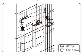
Figure 6-30 Placing the series box
