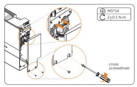
Figure 7-72 Locking the cable shielding board
