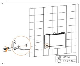
Figure 6-38 Tightening screws
