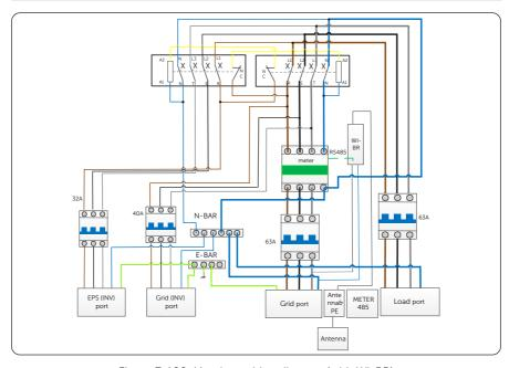
Figure 7-100 Matebox wiring diagram (with Wi-BR)
