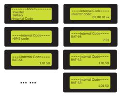
Figure 9-105 Displaying the internal code information
