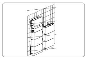
Figure 6-29 Installing two towers
