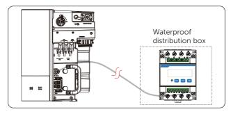
Figure 14-13 Connecting inverter to meter
