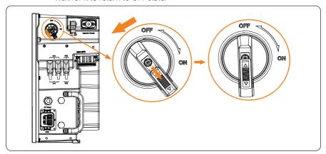
Figure 8-9 Unlocking DC switch
