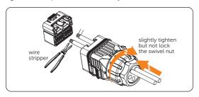
Figure 7-56 Stripping cables
