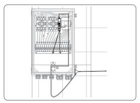
Figure 7-99 Connecting the Wi-BR and antenna
