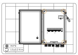
Figure 7-89 Loosening screws on the plate
