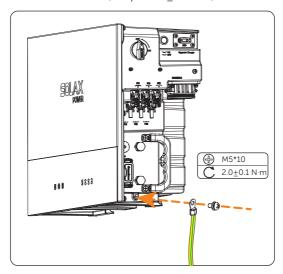
Figure 7-18 Securing the PE cable
