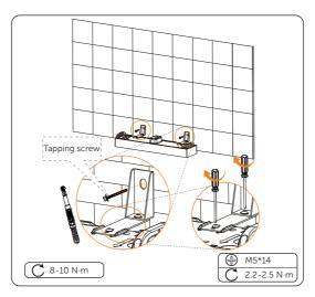
Figure 6-11 Securing the assembled bracket
