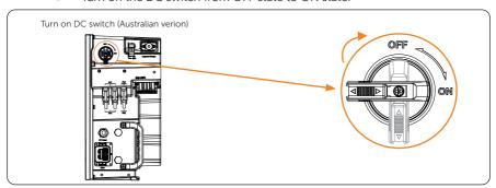
Figure 8-6 Turning on DC switch
