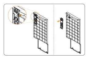
Figure 12-5 Remove the disassembling tool (only for pro version)
