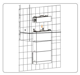
Figure 6-47 Placing the BMS
