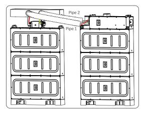
Figure 7-11 Inserting pipes into the cover
