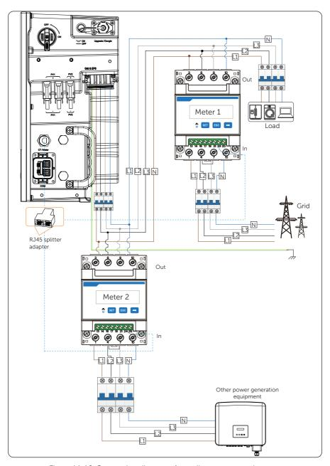
Figure 14-16 Connection diagram of two direct-connected meters
