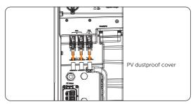
Figure 7-43 Removing the dustproof cover
