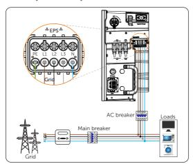
Figure 8-1 Turning on AC breaker
