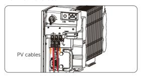
Figure 7-44 Connecting PV cables
