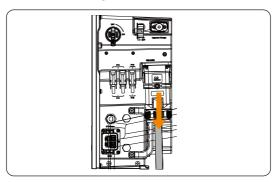
Figure 12-12 Unplugging the AC connector
