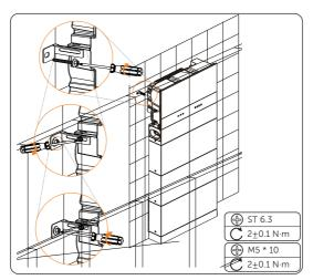
Figure 6-28 Locking the inverter brackets
