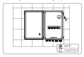
Figure 7-139 Securing the plate
