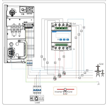
Figure 14-10 System wiring with CT-connected meter
