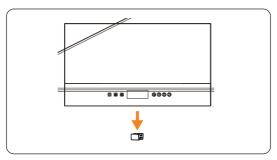
Figure 6-25 Removing the dustproof cover
