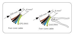
Figure 7-101 Stripping the EPS (INV) and Grid (INV) cable
