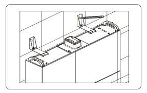
Figure 6-16 Marking the position of BMS
