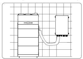
Figure 7-112 Well connected EPS and Grid cable
