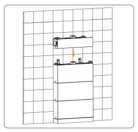
Figure 6-22 Placing the BMS
