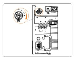
Figure 8-2 Turning on the DC switch
