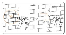
Figure 6-34 Drilling holes
