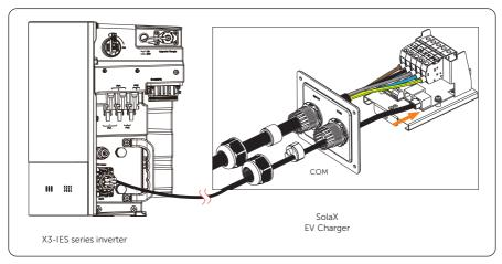
Figure 7-52 Inverter connected with a SolaX EV Charger
