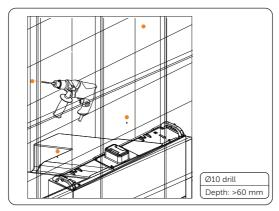
Figure 6-44 Drilling holes
