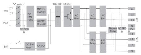
Figure 2-23 X3-IES system circuit diagram
