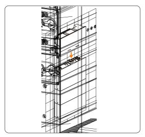
Figure 6-51 Installing the inverter
