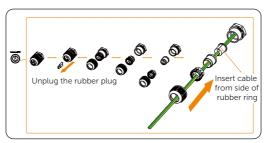
Figure 7-115 Threading the PE cable through Antenna&PE port
