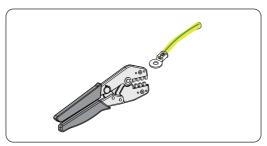
Figure 7-114 Crimping the PE cable
