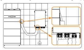
Figure 7-123 Well connected meter cable
