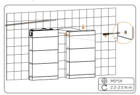
Figure 7-13 Tightening M5 screws
