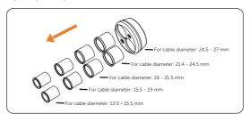
Figure 7-24 Taking out sealing plug
