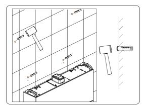
Figure 6-20 Knocking expansion tubes into the wall
