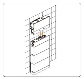
Figure 6-26 Installing the inverter
