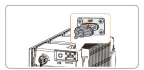
Figure 7-82 Installing the WiFi connecting cable
