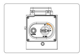
Figure 12-3 Turning off the BAT switch
