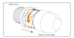
Figure 7-8 Closing short-circuit plug
