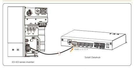
Figure 7-51 Inverter connected with a SolaX datahub
