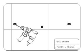
Figure 6-57 Drilling holes
