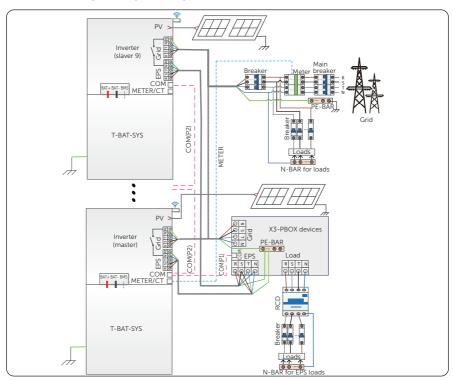
Figure 7-47 System diagram with SolaX X3-PBOX device
