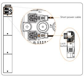
Figure 7-6 Removing short power cable
