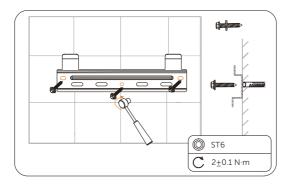
Figure 6-59 Securing the bracket
