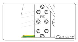
Figure 7-117 Threading the PE cable through Antenna&PE port
