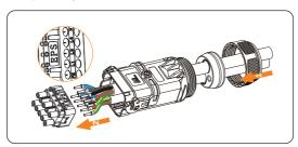
Figure 7-26 Inserting Grid and EPS cables into the AC connector
