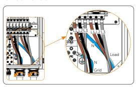
Figure 7-133 Connecting assembled Grid and Load cables to the matebox
