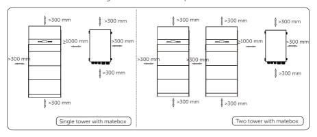
Figure 4-7 Clearance requirement with matebox
