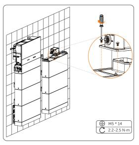
Figure 6-55 Placing the series box
