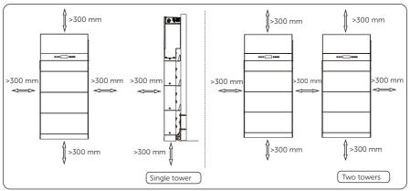
Figure 4-6 Clearance requirement
