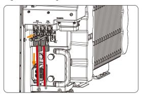
Figure 12-7 Pulling out PV connectors
