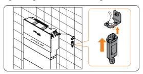
Figure 7-84 Plugging the dongle
