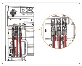
Figure 7-35 Well connected PV cables
