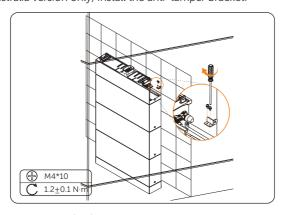
Figure 6-49 Install the anti-tamper bracket
