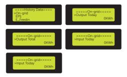
Figure 9-20 Displaying on-grid data
