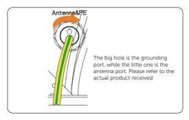
Figure 7-116 Tighting the waterproof connector
