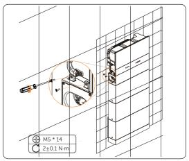
Figure 6-52 Locking the inverter with the BMS
