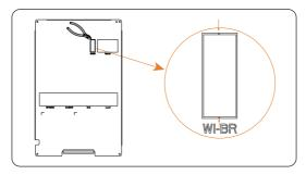
Figure 7-91 Cutting the baffle
