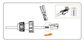
Figure 7-68 Crimping the communication cable for meter
