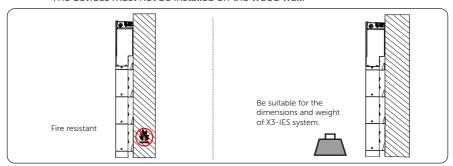
Figure 4-5 Installation carrier requirement
