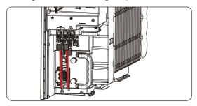
Figure 7-46 Well connected PV cables
