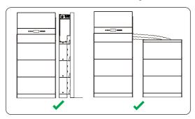
Figure 6-1 Correct installtion angle
