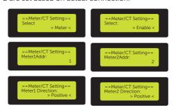
Figure 14-18 Selecting meter and set Meter 1 and Meter 2 data
