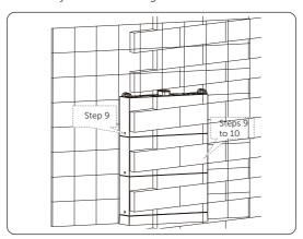
Figure 6-14 Placing battery modules
