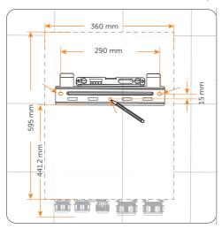
Figure 6-56 Positioning the matebox bracket
