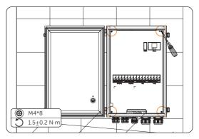
Figure 7-87 Loosening screws on the plate
