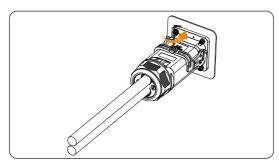
Figure 12-10 Loosening the AC connector
