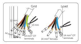
Figure 7-130 Assembling the Grid annd Load cable
