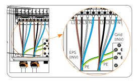
Figure 7-87 Connecting cables to the terminal block in the matebox
