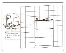
Figure 6-21 Tightening the BMS brackets
