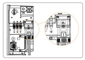
Figure 7-15 Well connected Grid & EPS cables
