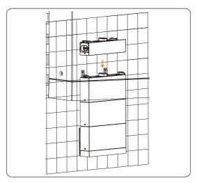
Figure 6-47 Placing the BMS
