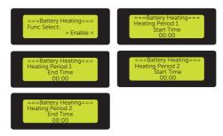
Figure 9-88 Enabling battery heating and setting working periods
