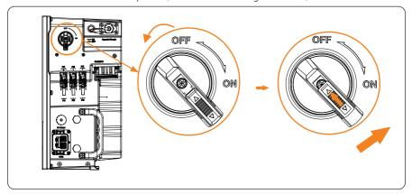
Figure 8-8 Locking DC switch
