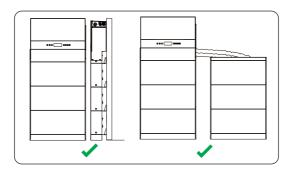
Figure 6-1 Correct installtion angle
