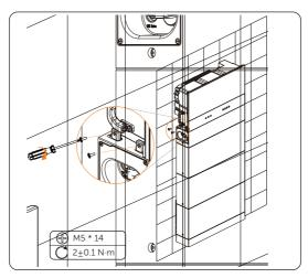
Figure 6-51 Locking the inverter with the BMS
