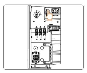
Figure 8-4 Pressing the inverter button
