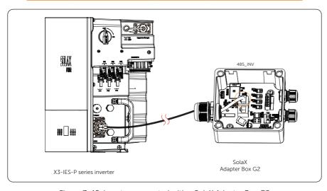
Figure 7-48 Inverter connected with a SolaX Adapter Box G2
