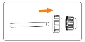
Figure 7-59 Threading the communication cable
