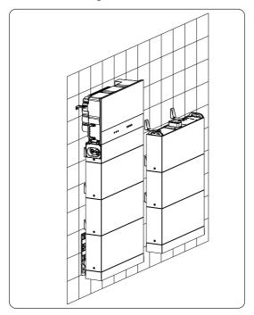
Figure 6-53 Installing two towers
