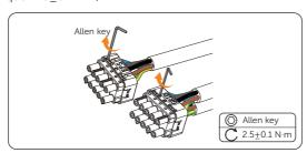
Figure 7-23 Locking wires in the AC connector
