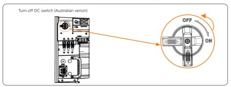
Figure 8-7 Turning off DC switch
