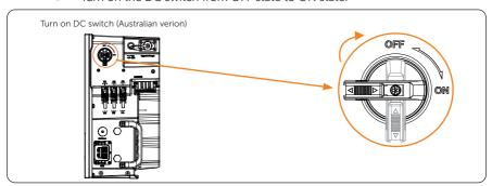
Figure 8-6 Turning on DC switch
