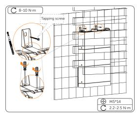
Figure 6-46 Securing the assembled bracket
