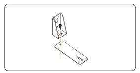
Figure 6-15 Attaching two brackets
