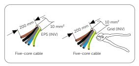
Figure 7-82 Stripping the EPS (INV) and Grid (INV)cable
