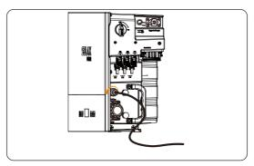
Figure 12-15 Disconnecting the CT/Meter cable
