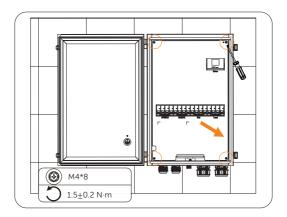
Figure 7-79 Loosening screws on the plate
