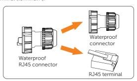
Figure 7-58 Disassembling the waterproof RJ45 connector
