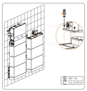
Figure 6-54 Placing the series box
