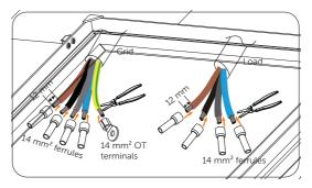
Figure 7-94 Assembling the Grid annd Load cable
