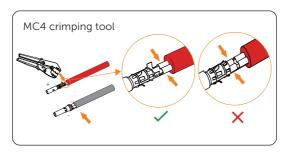
Figure 7-33 Crimping cables with PV pin contacts
