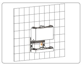
Figure 6-37 Placing battery module
