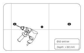
Figure 6-56 Drilling holes
