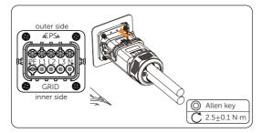
Figure 7-28 Tightening the lock on the AC connector
