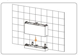
Figure 6-12 Placing the battery module
