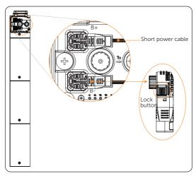
Figure 7-6 Removing short power cable
