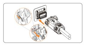
Figure 7-27 Plugging the AC connector into the port on the inverter
