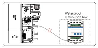
Figure 14-13 Connecting inverter to meter
