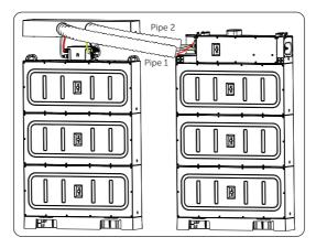
Figure 7-11 Inserting pipes into the cover
