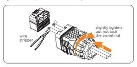
Figure 7-51 Stripping cables
