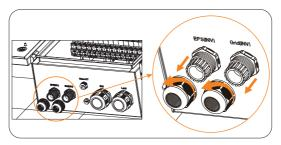
Figure 7-85 Loosening the Grid (INV) and EPS (INV) swivel nut
