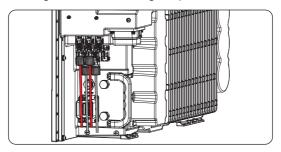
Figure 7-41 Well connected PV cables
