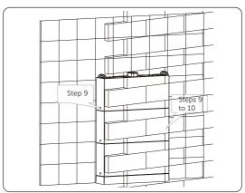
Figure 6-14 Placing battery modules
