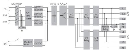
Figure 2-23 Circuit Diagram
