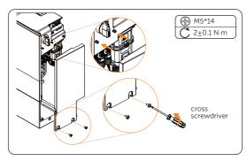
Figure 7-65 Locking the cable shielding board
