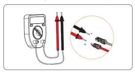
Figure 7-37 Measuring the voltage of PV connectors
