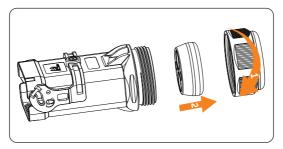
Figure 7-18 Disassembling the AC connector
