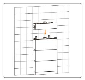
Figure 6-22 Placing the BMS
