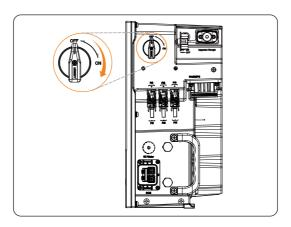
Figure 8-2 Turning on the DC switch
