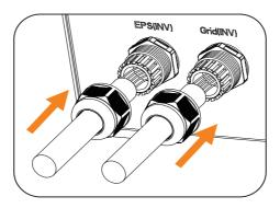
Figure 7-86 Threading EPS (INV) and Grid (INV) cables through the ports
