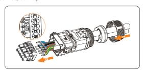
Figure 7-22 Inserting Grid and EPS cables into the AC connector
