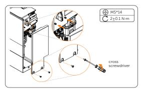
Figure 7-67 Locking the cable shielding board
