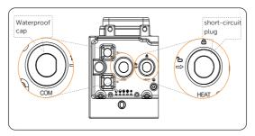
Figure 7-7 Removing waterproof cap
