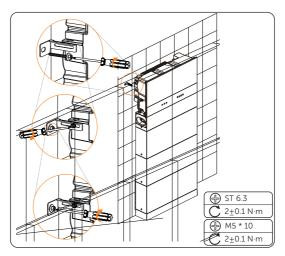
Figure 6-28 Locking the inverter brackets
