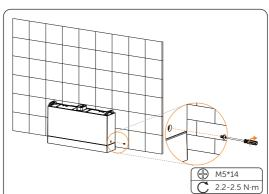
**Step 10:** Insert and tighten M5\*14 screws on both sides (torque: 2.2-2.5 N·m).
