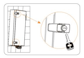
Figure 7-78 Unlocking the buckles
