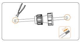
Figure 7-60 Stripping the communication cable for CT
