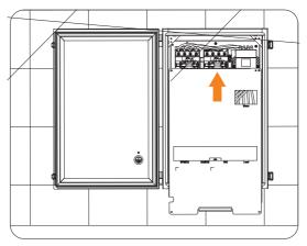
Figure 7-99 Reinstalling the plate
