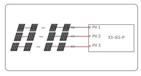
Figure 7-29 "Multi" mode connection diagram
