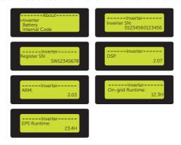
Figure 9-103 Displaying the inverter information
