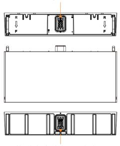
A hot-plug interface that is connected to the bottom of the battery module or the Base.
