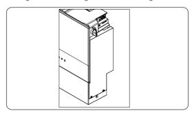
Figure 7-68 Locking the board well
