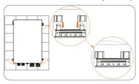
Figure 6-59 Hanging the matebox on the bracket
