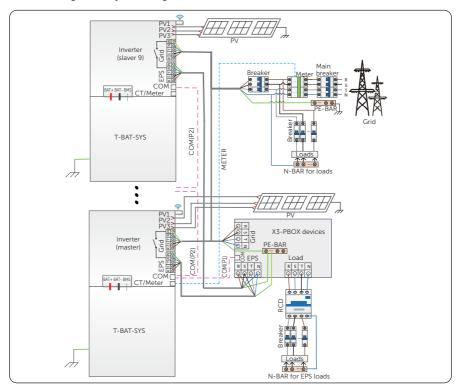
Figure 7-42 System diagram with SolaX X3-PBOX device
