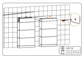
Figure 7-13 Tightening M5 screws
