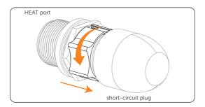
Figure 7-8 Closing short-circuit plug
