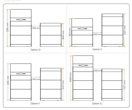
Figure 4-4 Installation options for two towers
