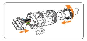
Figure 7-24 Wiring the AC connector
