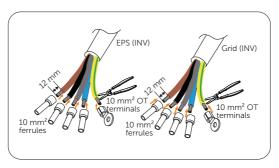
Figure 7-83 Stripping cables and inserting terminals into cables
