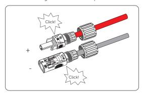
Figure 7-35 Securing PV cables
