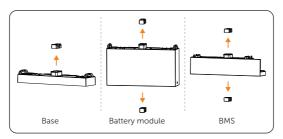
Figure 6-31 Removing dust covers
