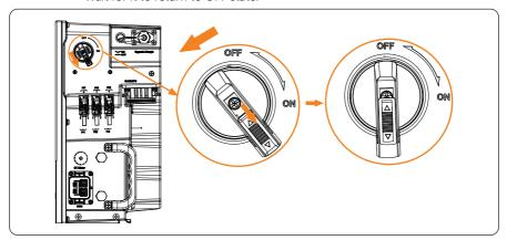
Figure 8-9 Unlocking DC switch
