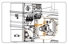
Figure 12-14 Disconnecting the communication connector
