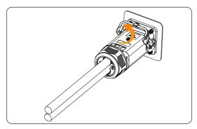
Figure 12-11 Removing the latch of the AC connector
