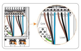
Figure 7-98 Connecting assembled Grid and Load cables to the matebox
