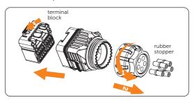
Figure 7-50 Disassembling the communication connector
