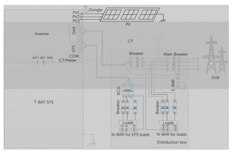
Figure 2-26 System diagram without X3-Matebox G2 for Australia
