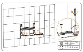
Figure 6-36 Securing the base
