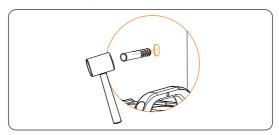
Figure 6-10 Inserting the expansion bolt
