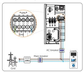
Figure 8-1 Turning on AC breaker
