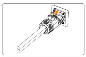
Figure 12-10 Loosening the AC connector
