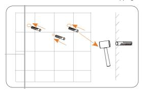
Figure 6-57 Knocking expansion tubes into the wall
