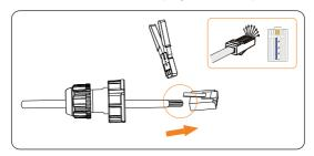
Figure 7-63 Crimping the communication cable for meter
