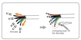
Figure 7-17 Crimping the Grid and EPS cables
