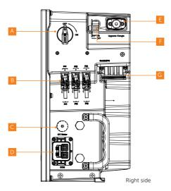
Figure 2-14 Ports of an inverter
