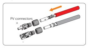
Figure 7-34 Threading PV cables with PV pin contacts connected
