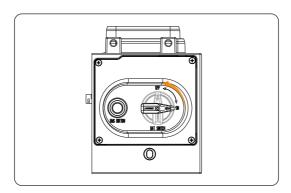
Figure 12-3 Turning off the BAT switch
