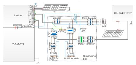
Figure 2-28 Micro grid system diagram
