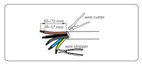
Figure 7-16 Striping the Grid and EPS cables
