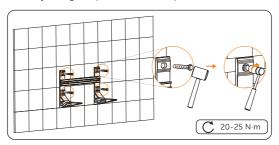
Figure 6-35 Tightening expansion screws
