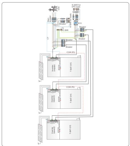
Diagram 2: System diagram without SolaX X3-PBOX device
