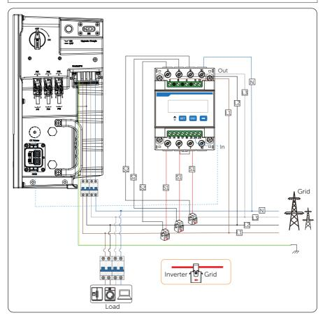
Figure 14-10 System wiring with CT-connected meter
