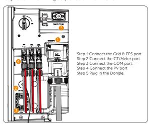
Figure 7-14 Wiring sequence of the inverter
