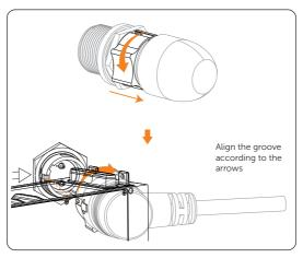
Figure 7-12 Locking heater cable
