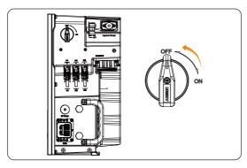
Figure 12-2 Turning off the DC switch
