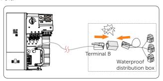
Figure 14-3 Connecting the inverter to the CT
