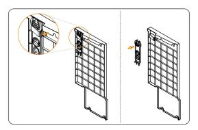
Figure 12-5 Remove the disassembling tool
