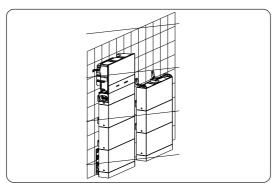
Figure 6-29 Installing two towers
