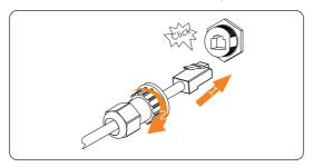
Figure 7-64 Connecting cable to the CT/Meter port
