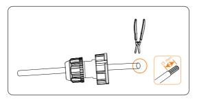
Figure 7-62 Stripping the communication cable for meter
