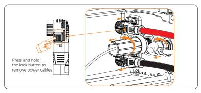
Figure 12-17 Disconnecting battery connectors
