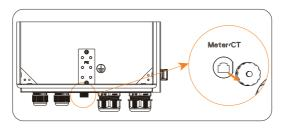
Figure 7-89 Removing the cap
