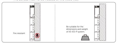
Figure 4-5 Installation carrier requirement
