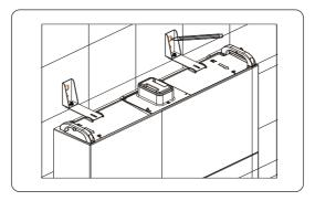
Figure 6-41 Marking the position of BMS
