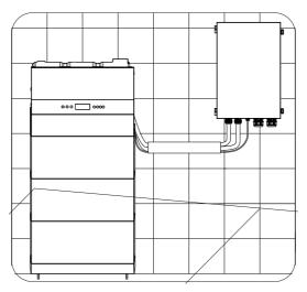
Figure 7-91 Well connected meter cable
