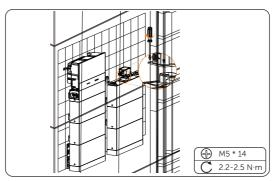
Figure 6-30 Placing the series box
