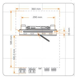
Figure 6-55 Positioning the matebox bracket
