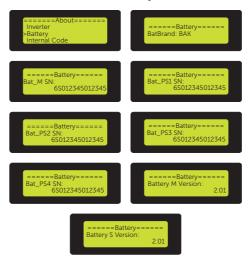
Figure 9-104 Displaying the battery information
