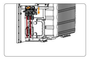
Figure 12-8 Pulling out PV dustproof buckles
