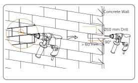
Figure 6-9 Drilling holes
