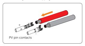
Figure 7-32 Inserting PV pin contacts into PV cables
