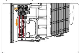
Figure 12-7 Pulling out PV connectors
