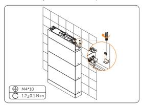
Figure 6-24 Install the anti-tamper bracket
