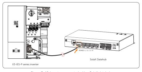
Figure 7-46 Inverter connected with a SolaX datahub
