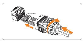
Figure 7-54 Inserting wires into ferrules
