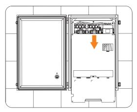
Figure 7-80 Removing the plate
