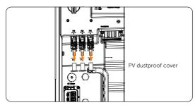
Figure 7-38 Removing the dustproof cover
