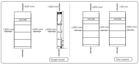
Figure 4-6 Clearance requirement
