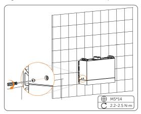
Figure 6-38 Tightening screws
