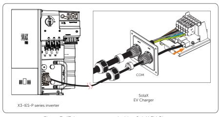
Figure 7-47 Inverter connected with a SolaX EV Charger
