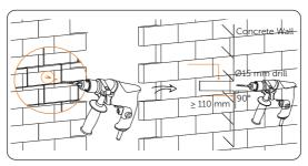
Figure 6-34 Drilling holes
