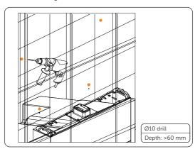
Figure 6-19 Drilling holes
