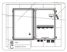
Figure 7-100 Securing the plate
