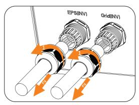
Figure 12-19 Disassembling EPS(INV) and Grid(INV) cables
