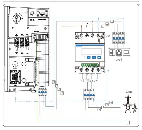
Figure 14-5 System wiring with direct-connected meter
