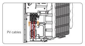
Figure 7-39 Connecting PV cables
