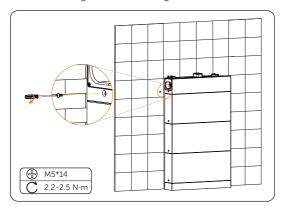
Figure 6-23 Tightening M5 screws
