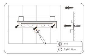
Figure 6-58 Securing the bracket
