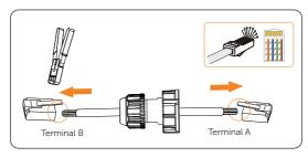
Figure 7-61 Crimping the communication cable for CT
