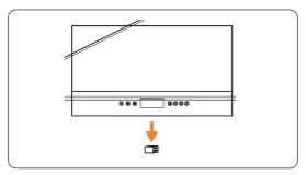
Figure 6-25 Removing the dustproof cover
