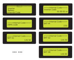
Figure 9-105 Displaying the internal code information
