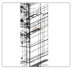
Figure 6-50 Installing the inverter
