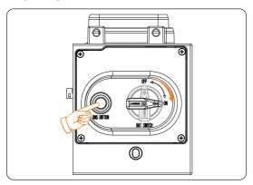
Figure 8-3 Turning on the battery
