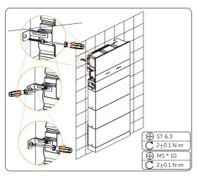
Figure 6-52 Locking the inverter brackets
