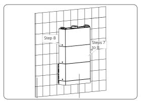
Figure 6-39 Placing battery modules
