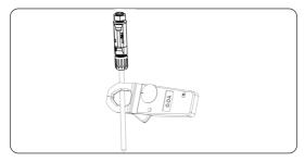
Figure 12-4 Detecting the current
