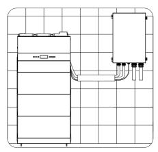
Figure 7-88 Well connected EPS (INV) and Grid (INV) cable
