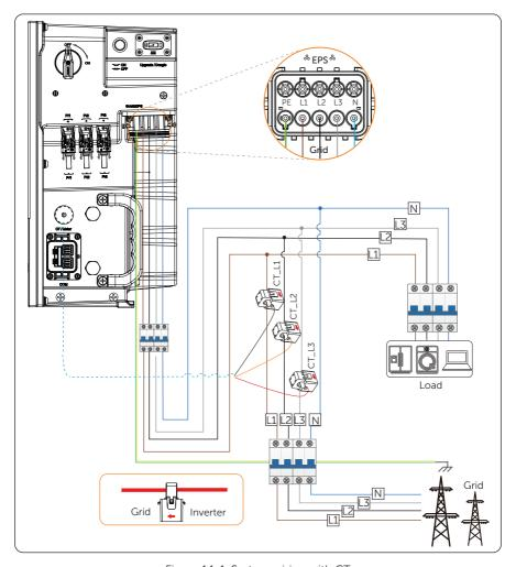
Figure 14-1 System wiring with CT
