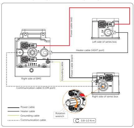
Figure 7-9 Connecting cables
