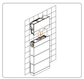
Figure 6-26 Installing the inverter
