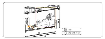
Figure 12-18 Disconnecting grounding cable
