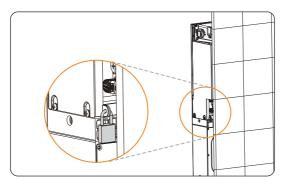
Figure 7-69 Installing the padlock
