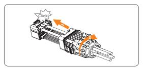
Figure 7-56 Inserting the terminal block into the connector
