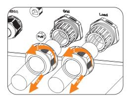
Figure 12-20 Disassembling Grid and Load cables
