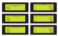
Figure 9-14 Displaying PV1 and PV2 status
