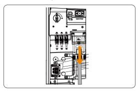
Figure 12-12 Unplugging the AC connector
