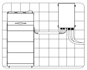
Figure 7-102 Well connected Grid and Load cables
