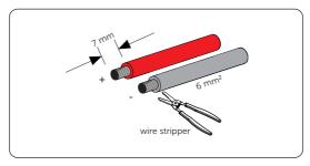
Figure 7-31 Stripping PV cables
