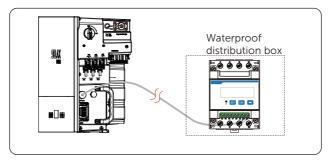
Figure 14-8 Connecting inverter to meter
