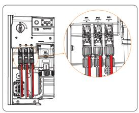
Figure 7-30 Well connected PV cables
