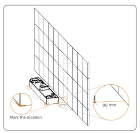
Figure 6-6 Placing the base
