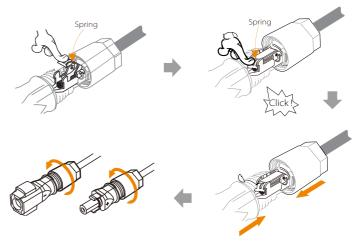
**Step 5.** Insert the battery cables into the corresponding BAT port (+), (-) of the inverter.
