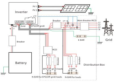
Diagram B: N line and PE line separate wiring, M series inverters; (For most countries)
