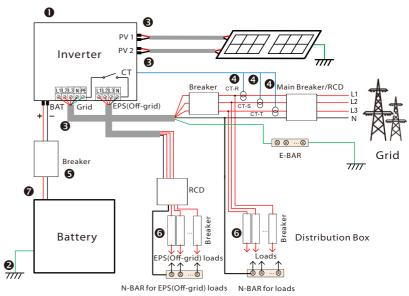
Note: The RCD on the figure represents a leakage protection device with a circuit breaker function.
