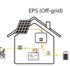
In case of power failure, the system will provide uninterrupted power supply to the EPS loads using the power from PV and the battery. It is important to ensure that a battery is installed, and the EPS loads should not exceed the maximum output power of the battery. The power generated by PV will prioritize supplying power to the loads, while any surplus power will be utilized to charge the battery.
