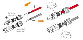
Step 6. Then screw down the cable nut.
