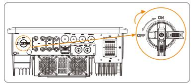
• To turn off the DC switch i) Rotate the DC switch from ON state to OFF state.
