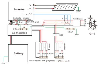
Diagram D: N line and PE line together, all load connection EPS(Off-grid) scheme: (Applicable to Australia)
