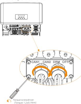
**Step 6**. Tighten the screws and lock the cover on the inverter. And then tighten the swivel nuts.
