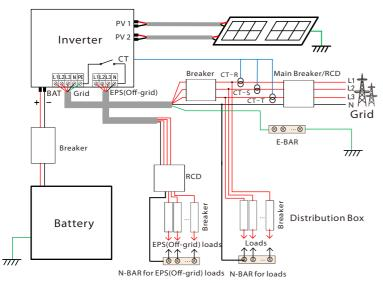
Diagram B: N line and PE line separate wiring, M series inverter; (For most countries)
