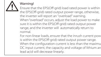
For non-linear loads, ensure that the inrush current power is within the EPS(Off-grid) rated output power range. When the configuration current is less than the maximum DC input current, the capacity and voltage of lithium and lead acid will decrease linearly.
