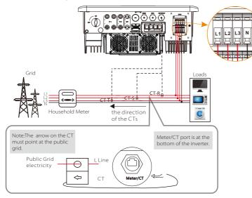
Note: CT-R must be connected to L1, CT-S connected to L2 and CT-T connected to L3 in accordance with the L1, L2 and L3 of the inverter's grid port. The household meter should be installed on the power lines.
