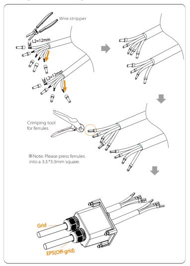
**Step 4.** Insert the L1, L2, L3, N wires of Grid cable into the corresponding ports of the Grid terminal block, and insert the L1, L2, L3 wires of EPS (off-grid) into the corresponding ports of EPS terminal block. And then tighten the wires with a flat-head screwdriver. (Torque: 1.5±0.1N·m)
