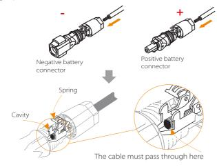
**Step 4.** Press down the spring by hand and you can hear a "click" sound, and then push the ends together, and tighten the joints of the connectors.
