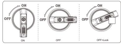
• To turn on the DC switch i) Turn on the DC switch from OFF state to ON state.
