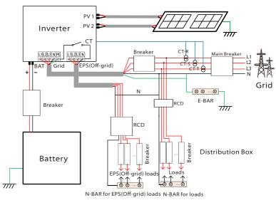
Diagram D: N line and PE line together, M series inverter; (Applicable to Australia)
