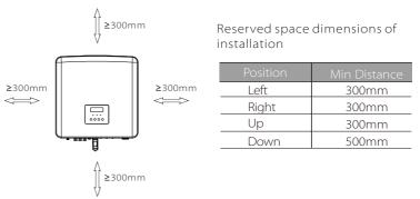
For multi-inverter installation scenarios, the inline installation method is recommended; when the space is insufficient, the recommended method of installation in the form of "products"; it is not recommended to install multiple inverters in stacks. If you choose stack installation, please refer to the installation separation distance below.
