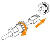
**Step3:** For a CT connection, plug the terminal B to RJ45 connector. For a meter connection, connect pin 4 and pin 5 of the stripped end directly to the pin 24 and pin 25 of a meter. Please refer to a meter manual for a specific connection method.
