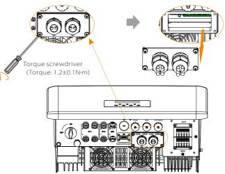
**Step 3.** Thread communication cables through CAN1/ CAN2/ DRM/ OFF port of the cover. And then strip off 15 mm insulation layer.
