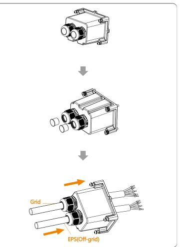
**Step 3.** Strip off 12mm insulation layer at one end of the two cables. Insert the ferrules into the stripped end of cables respectively, and finally use a crimping tool for ferrules to tighten the ferrules.
