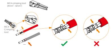
Step 5. Separate the DC connector as two parts: the plug and the cable nut. Insert the wire into plug forcibly, when a "click" is heard or felt, the pin contact assembly is seated correctly.
