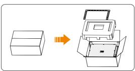
• Unpacking the inverter according to the following figure.
