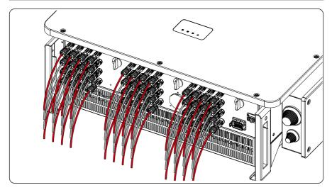
Figure 7-1 Inverter PV full connection diagram
