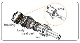
Figure 7-61 Plugging the cable
