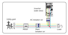
Figure 8-68 Turning on AC breaker
