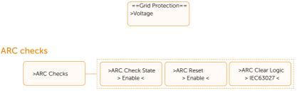
**ARC Check State** enables arc detection, allowing the system to detect and report any corresponding arc faults that occur during arcing. **ArcSelfCheck** enables a self-check for arc detection functionality, verifying whether the device can correctly identify any detection mechanism faults. **ArcSensitivity** function allows users to adjust the sensitivity of arc fault detection.
