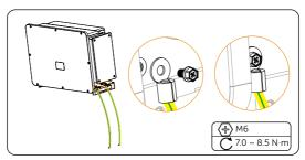
Figure 7-7 Securing the PE cable
