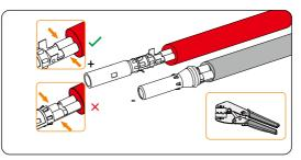
Figure 7-50 Crimping the terminal
