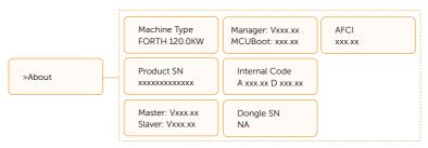
This interface shows information of the inverter, include model, SN, software version of master DSP, slaver and ARM board and internal code.
