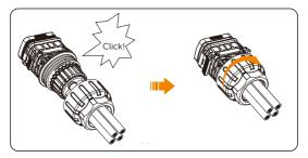
Figure 7-62 Securing the nut
