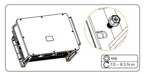
Figure 6-12 Locking the inverter
