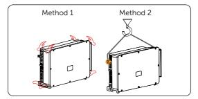
Figure 6-19 Lifting the inverter
