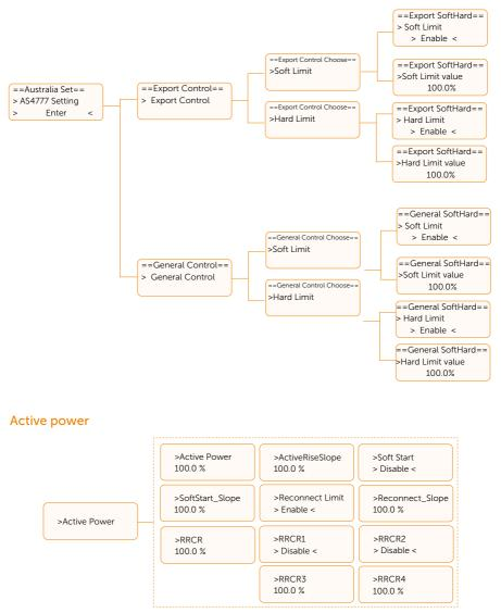
This interface is used to set the active power according to the requirement of utility grid.
