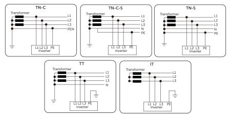
Figure 2-4 136 kW and 150 kW inverters supported power grid
