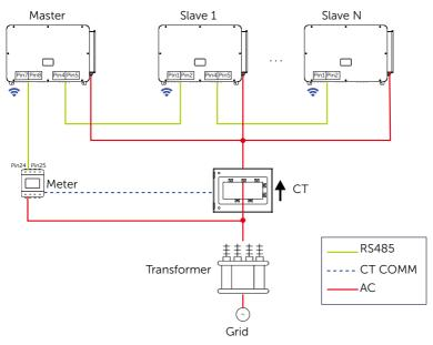
Figure 14-2 Parallel system diagram with Modbus
