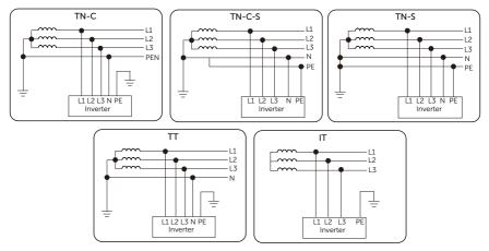
136 kW and 150 kW models are directly connected to the medium voltage power grid through a 500 V or 540 V transformer without an N line access, as shown in Figure 2-4.
