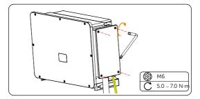
Figure 7-18 Re-installing the cover
