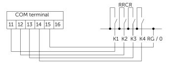
Figure 14-5 RRCR connection diagram
