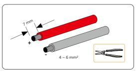
Figure 7-48 Stripping the PV cable
