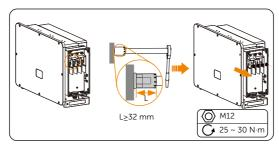
Figure 7-13 Disassembling the M12 nut (40 kW ~ 70 kW / 75 kW ~ 125 kW inverter for example)
