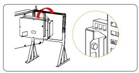
Figure 6-11 Securing the inverter
