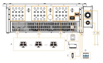
Figure 7-2 Cable connections of inverter
