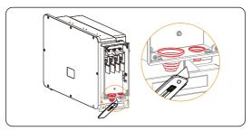
Figure 7-14 Cutting off the pagoda-shaped coil
