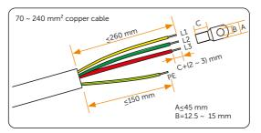
Figure 7-9 Stripping the AC cable (136 kW ~ 150 kW inverter)
