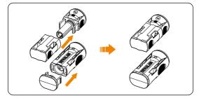
Figure 7-55 Sealing the unused ports
