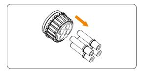
Figure 7-59 Removing the waterproof plug
