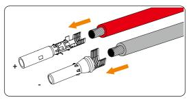
Figure 7-49 Inserting the PV pin contact
