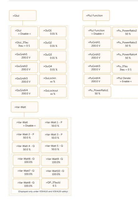
Usually end user do not need to set the grid protection. All default value have been set before leaving factory according to safety rules. If reset is needed, any changes should be made according to the requirements of local grid.
