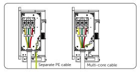
Figure 7-17 Wiring connection diagrams for PE cable (136 kW ~ 150 kW inverter)
