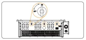
Figure 8-67 Turning on DC switch
