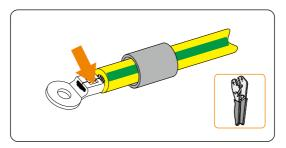
Figure 7-5 Crimping the cable
