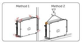
Figure 6-18 Lifting the inverter
