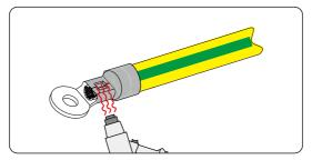
Figure 7-6 Shrinking the tubing
