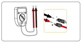
Figure 7-53 Measuring the voltage of PV connectors
