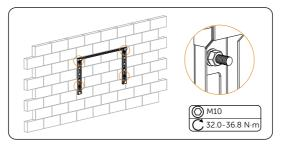
Figure 6-17 Securing the bracket
