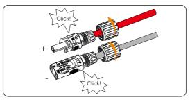
Figure 7-52 Securing the PV cable
