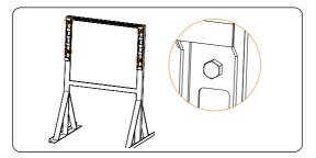
Figure 6-8 Tightening the screws
