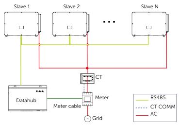
Figure 14-1 Parallel system diagram with Datahub
