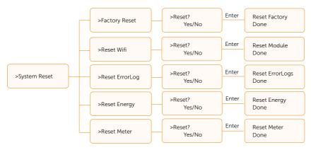
Here you can reset dongle, error logs, energy logs, and meter. In addition, restoring factory default setting is allowed.
