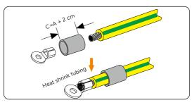
Figure 7-4 Installing the tubing and OT terminal
