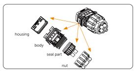
Figure 7-58 Disassembling the connector
