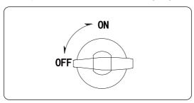
Figure 12-1 Turning off the DC switch
