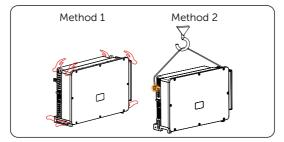
Figure 6-10 Lifting the inverter
