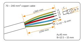
Figure 7-8 Stripping the AC cable (40 kW ~ 70 kW / 75 kW ~ 125 kW inverter)
