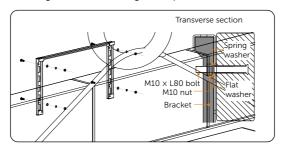
Figure 6-15 Inserting the expansion screws
