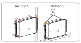
Figure 6-9 Lifting the inverter
