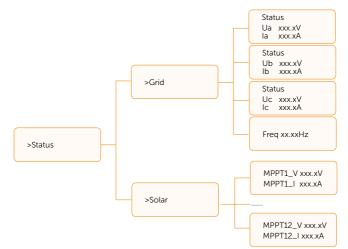
The status function contains **Grid** and **Solar**. Press **Up** and **Down** to select and press **Enter** to confirm the selection. Press **ESC** to return to menu.
