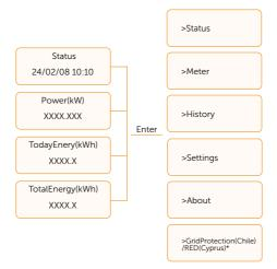
The main interface (Level 1) is the default interface, the inverter will automatically jump to this interface when the system started up successfully or not operated for a period of time.
