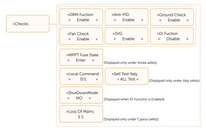
This interface is used to activate the needed functions. Users configure the enable settings for each branch, including Italy self-test, MPPT fuse state, etc.
