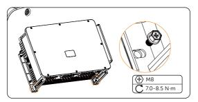
Figure 6-21 Securing the inverter
