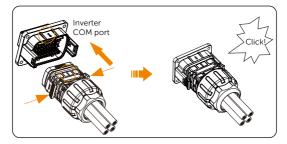
Figure 7-63 Securing and connecting the cable
