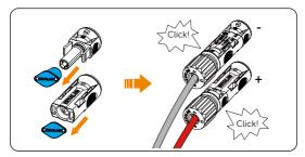
Figure 7-54 Connecting the PV cable
