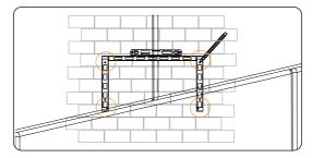
Figure 6-13 Marking the holes
