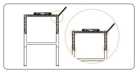
Figure 6-5 Marking the holes
