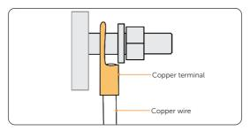
Figure 7-14 Copper terminal crimping
