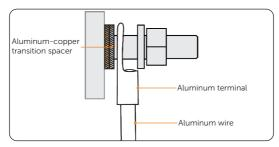
Figure 7-16 Aluminum terminal crimping
