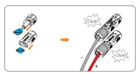
Figure 7-35 Connecting the PV cable
