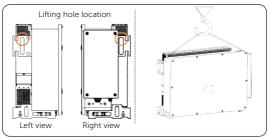
Figure 6-9 Crane handling
