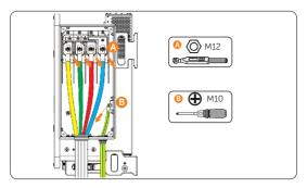
Figure 12-6 Disconnecting cables
