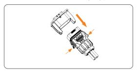
Figure 12-8 Disconnecting the communication connector
