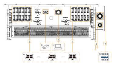
Figure 7-2 Cable connections of inverter
