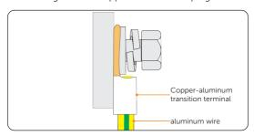
Figure 7-5 Aluminum-copper transition terminal crimping
