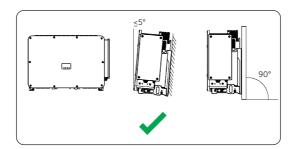
Figure 6-1 Correct installation
