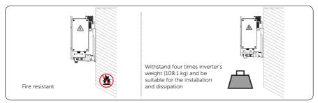
Figure 4-3 Installation carrier requirement
