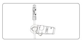
Figure 12-3 Measuring DC current
