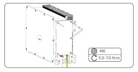
Figure 7-25 Closing the AC wiring box
