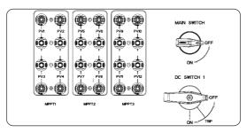
Figure 7-26 DC SWITCH 1 controls the DC terminals PV1 ~ PV12
