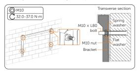
Figure 6-15 Securing the bracket
