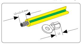
Figure 7-7 Stripping the PE cable
