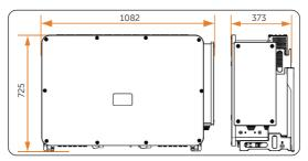
Figure 6-3 Dimensions 1 (Unit: mm)
