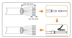
Figure 7-41 Stripping and crimping
