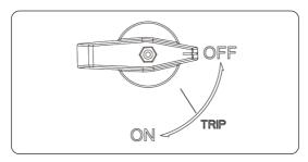
Figure 12-1 Turning off the DC switches
