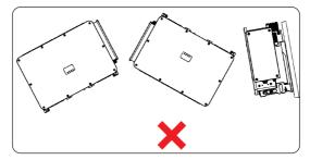
Figure 6-2 Incorrect installation
