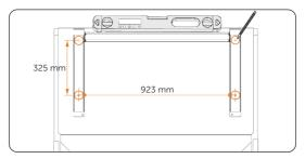
Figure 6-5 Marking the holes
