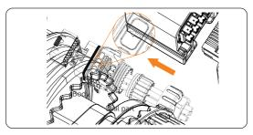
Figure 7-44 Running a cable through
