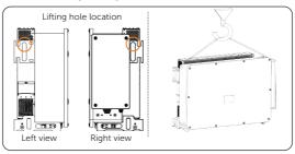
Figure 6-17 Crane handling
