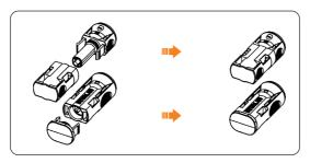
Figure 7-36 Installing the dustproof buckles
