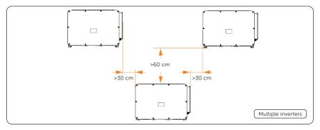
Figure 4-5 Clearance requirement for multiple inverters
