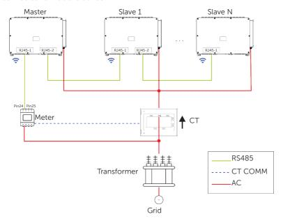
Figure 14-2 Parallel system diagram with Modbus
