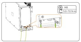
Figure 7-12 Securing the PE cable
