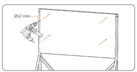
Figure 6-6 Drilling holes
