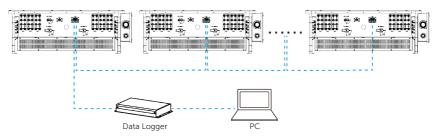
Figure 7-40 Multi-inverter communication diagram
