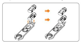
Figure 7-37 Disassembling the dustproof buckles
