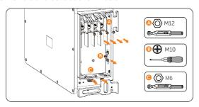
Figure 7-18 Removing the nuts and bolts
