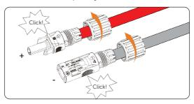
Figure 7-33 Securing the PV cable
