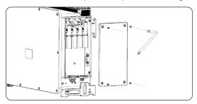
Figure 7-17 Opening the AC wiring box cover
