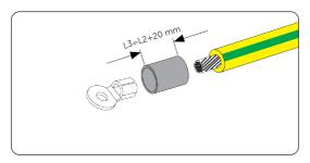
Figure 7-8 Installing the tubing and OT terminal
