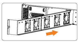
Figure 11-4 Replacing the fan bracket
