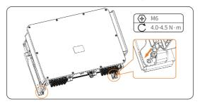
Figure 6-19 Securing the inverter
