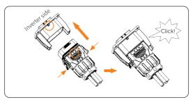
Figure 7-46 Connect to inverter
