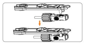
Figure 12-4 Disconnecting the PV connector
