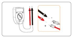
Figure 7-34 Measuring the voltage of PV connectors
