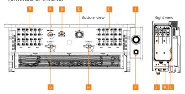
Figure 7-1 Terminals of inverter
