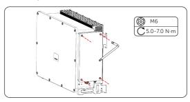
Figure 12-7 Closing the AC wiring box
