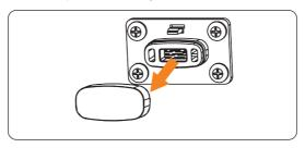
Figure 7-50 Removing the dust cap
