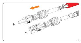
Figure 7-32 Threading the PV cable
