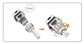
Figure 7-45 Assembly connector
