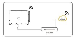
Figure 7-48 LAN mode connection diagram
