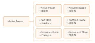
This interface is used to set the active power according to the requirement of grid.
