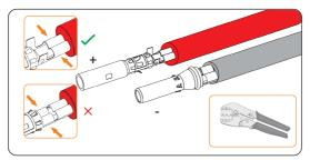
Figure 7-31 Crimping the terminal
