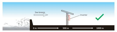
Figure 4-1 Recommended installation position
