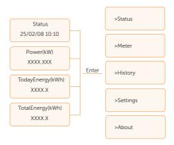
The main interface (Level 1) is the default interface, the inverter will automatically jump to this interface when the system started up successfully or not operated for a period of time.
