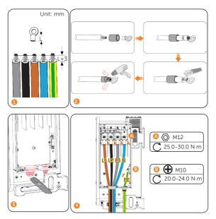
Figure 7-24 Single core wiring solution
