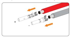
Figure 7-30 Inserting the PV pin contact
