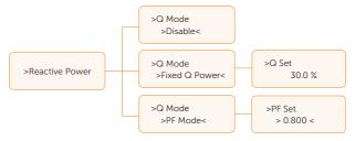
This interface is used to set the reactive power. Please set the value according to the requirement of utility grid.
