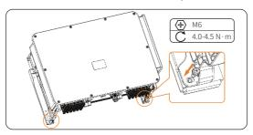
Figure 6-11 Securing the inverter
