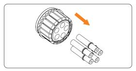
Figure 7-43 Removing the waterproof plug
