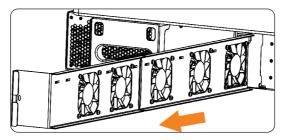
Figure 11-3 Pulling out the fan bracket completely
