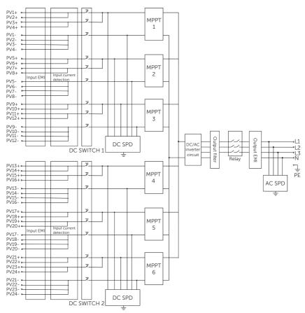
Figure 2-4 Circuit diagram
