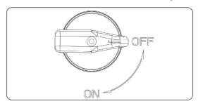
Figure 12-2 Checking the main switch
