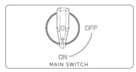
Figure 8-1 Turning on the main switch
