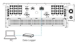
Figure 7-39 Single inverter communication diagram
