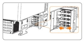
Figure 11-2 Disconnecting the cable
