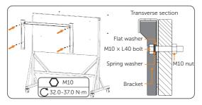
Figure 6-7 Securing the bracket
