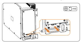
Figure 7-11 Removing the M8 screws
