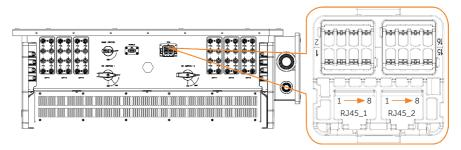
Figure 7-38 Communication port pin number
