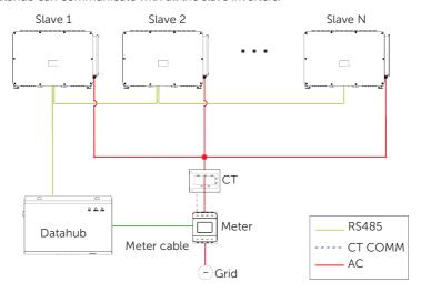
Figure 14-1 Parallel system diagram with Datahub
