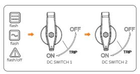
Figure 8-2 Turning on DC switches
