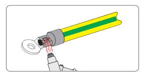
Figure 7-10 Shrinking the tubing
