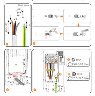
Figure 7-23 Multi-core wiring without N wire solution - Separate PE wiring
