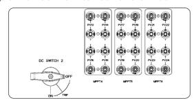
Figure 7-27 DC SWITCH 2 controls the DC terminals PV13 ~ PV24
