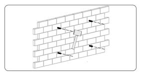
Figure 6-14 Inserting the expansion screws
