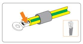
Figure 7-9 Crimping the cable
