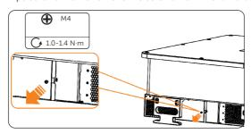
Figure 11-1 Removing the screws
