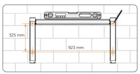
Figure 6-12 Marking the holes
