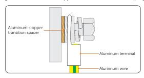
Figure 7-6 Aluminum terminal crimping
