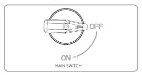
Figure 8-3 Turning off the main switch
