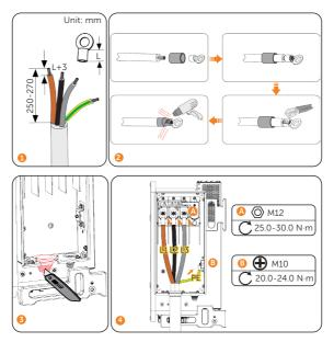
Figure 7-22 Multi-core wiring without N wire solution - Not separate PE wiring
