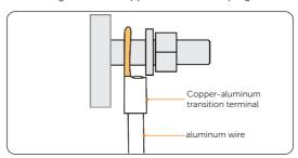
Figure 7-15 Aluminum-copper transition terminal crimping
