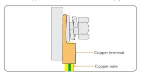
Figure 7-4 Copper terminal crimping
