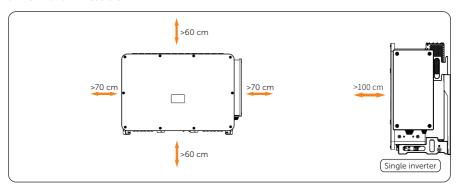
Figure 4-4 Clearance requirement for single inverter
