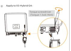
(For specific installation steps, please refer to the EPS port installation chapter of the X3-Hybrid /Fit Quick Installation Guide.)
