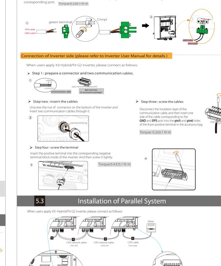
Meter Port: The first RJ45 port from left sid
