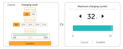
Figure 10-28 Setting maximum charging current
