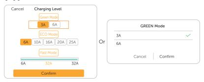
Figure 10-6 Charging current level for Green mode
