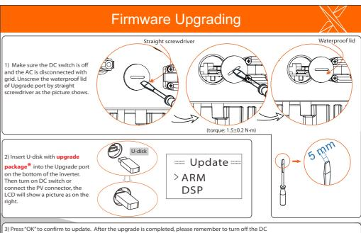
switch or disconnect the PV connector, then pull off the U-disk, screw the waterproof lid.
