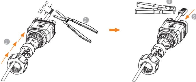
If the communication cable is with RJ45 terminal
