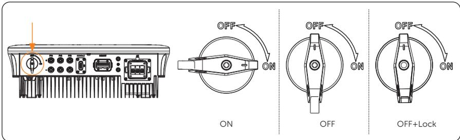
b. Operation of the lockable DC switch (Type 2):
