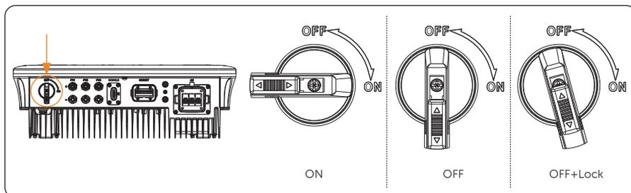
b. Operation of the lockable DC switch (Type 1):
