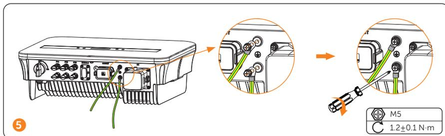
\* The external protective grounding terminal must meet at least one of the following requirements.
