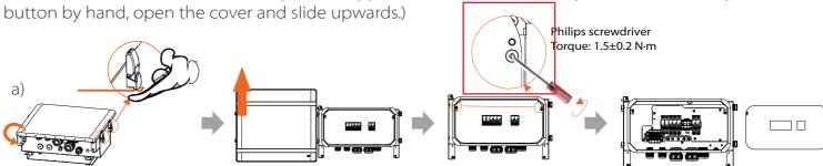
b) Put the matebox on the bracket. Make sure the box is well fixed on the bracket by screwing all nuts
