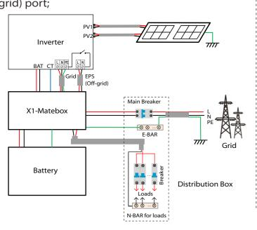
Diagram A: Neutral line and PE line are separated : Diagram B: Neutral line and PE line are combined together, all loads connect to the EPS (Off-grid)
