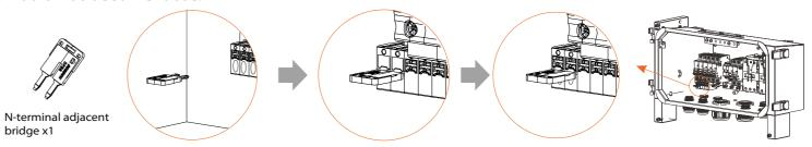
6.6 Finally, use a philips screwdriver to install the baffle back, install the upper cover, and then lock the buckle with a key
