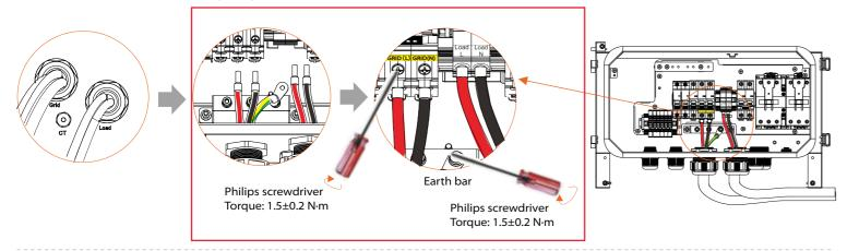
3) Take out the power cable from the BMS accessories, and cut it to 560-600 mm and strip 7 mm of the insulation layer from the wire ends. Crimp the 6 mm<sup>2</sup> BAT terminals on the wires. Then pass the cable through the BAT port of the matebox, then find the BAT+ and BAT- ports in the matebox, insert each wire accordingly, and use the philips screwdriver to lock the screws.
