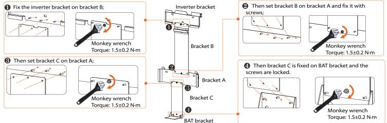
Step 2: Connect the BAT bracket and battery and push the whole structure to the wall
