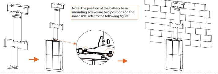
Step 3: Fix the position, drill holes and install the whole structure on the wall a) With the position of the brackets as a template in ; b) Move away the structure and drill holes at marked
