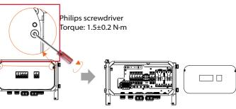
b) Put the matebox on the bracket. Make sure the box is well fixed on the bracket by screwing all nuts tightly.
