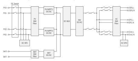
Figure 2-7 Circuit Diagram for X1-Hybrid-LV series inverter
