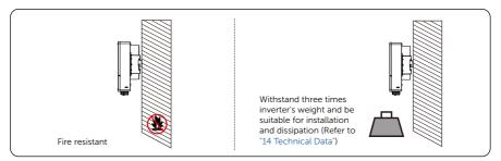
Figure 5-3 Installation carrier requirement
