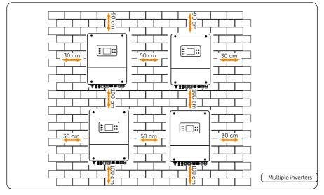
Figure 5-5 Clearance requirement for multiple inverter
