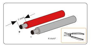
Figure 8-22 Striping the PV cable
