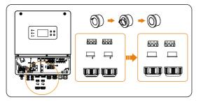
Figure 8-35 Remove the sealing cover
