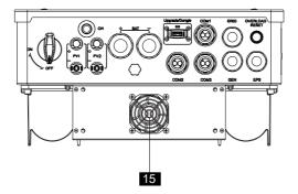
Figure 8-3 Terminals of Inverter (Bottom view 2)
