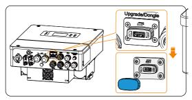
Figure 8-79 Remove the waterproof plug
