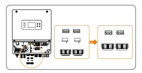
Figure 8-39 Remove the plug
