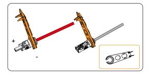
Figure 8-27 Unlocking the PV cable
