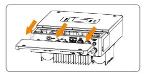
Figure 8-4 Remove the lower cover
