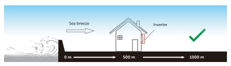
Figure 5-1 Recommended installation position
