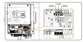
Figure 8-63 Insert the cable
