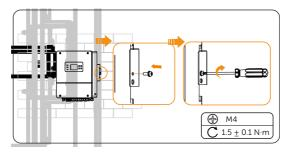
Figure 7-10 Securing the inverter
