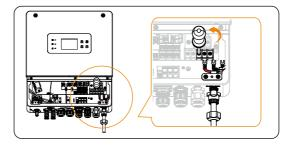
Figure 8-12 Insert the Grid cable
