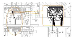
Figure 8-70 Insert the cable
