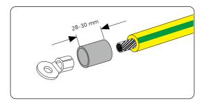
Figure 8-5 Installing the tubing and OT teriminal
