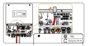
Figure 8-42 Tighten the cable
