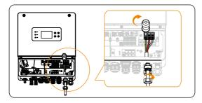
Figure 8-19 Tighten the EPS cable
