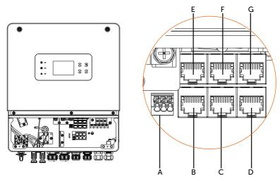
Figure 8-46 Communication ports
