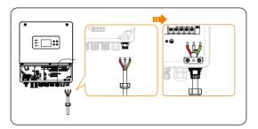
Figure 8-7 Pass the Grid cable
