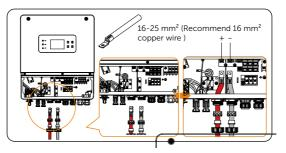
Figure 8-36 Pass and insert the cable
