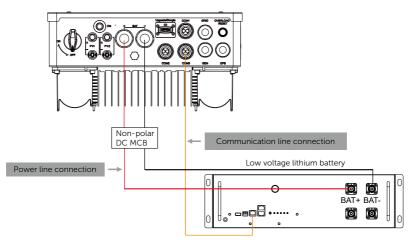
Figure 8-58 Lithium battery connection diagrm
