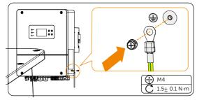
Figure 8-8 Securing the PE cable
