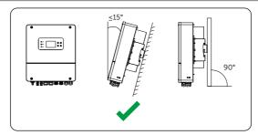
Figure 7-1 Correct installation
