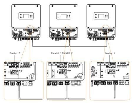
Figure 8-66 Parallel connection diagram
