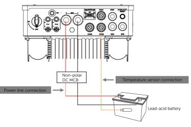
Figure 8-43 Battery temperature sensor connection diagram
