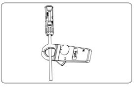
Figure 13-3 Measuring the current
