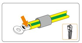
Figure 8-6 Crimping the cable
