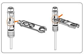
Figure 13-4 Disassembling the PV cables
