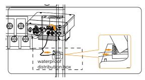
Figure 8-53 Insert the other side of the cable into the waterproof distribution box
