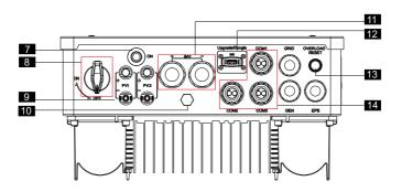
Figure 8-2 Terminals of Inverter (Bottom view 1)
