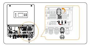
Figure 8-15 Insert the GEN cable
