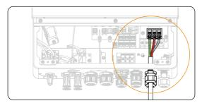
Figure 8-20 EPS cable connected
