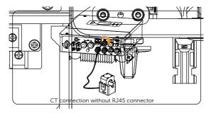
Figure 8-55 Insert the other side of the cable into the CT connection
