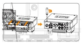
Figure 8-71 Close the lower cover and tighten the screws
