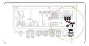
Figure 8-14 Grid cable connected
