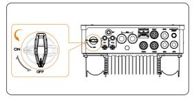
Figure 13-2 Turning off DC switch
