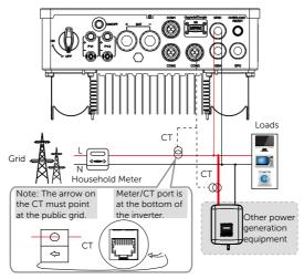
Figure 8-48 CT connection diagram
