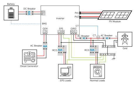
Figure 2-9 Wiring methods for Australia
