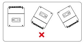
Figure 7-2 Incorrect installation
