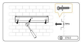
Figure 7-8 Securing the wall mounting bracket
