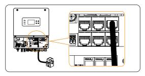
Figure 8-54 Insert one side of the cable into the inverter
