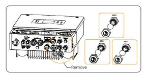
Figure 8-5 Remove the plug
