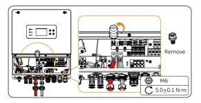
Figure 8-41 Remove the screw
