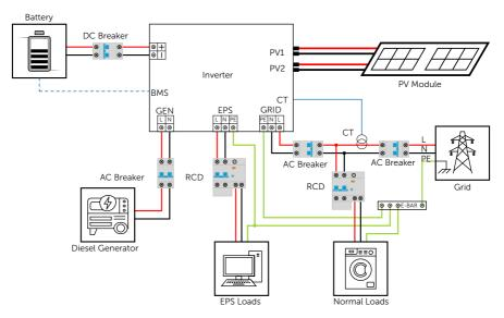
Figure 2-8 Wiring methods for most of the countries
