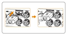
Figure 8-80 Plug the communication dongle
