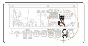
Figure 8-17 GEN cable connected
