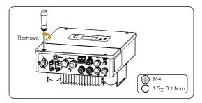
Figure 8-3 Loosen the screws
