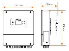
Figure 2-5 Dimension of Inverter
