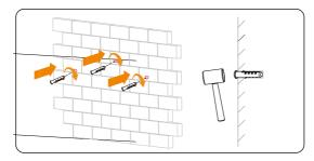
Figure 7-7 Insert the expansion bolt
