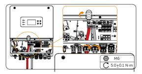
Figure 8-38 Tighten the cable
