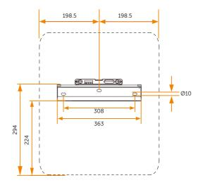
Figure 7-4 Dimensions 2 (Unit: mm)
