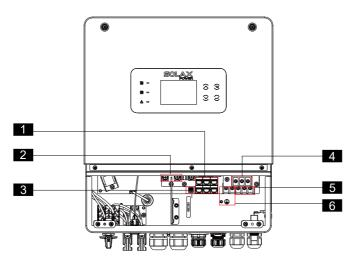
Figure 8-1 Terminals of Inverter (Front perspective view)
