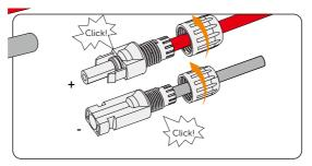
Figure 8-26 Securing the PV cable
