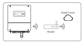
Figure 8-72 Wi-Fi mode connection diagram
