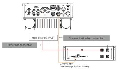
Figure 8-30 Battery connection diagram
