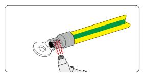
Figure 8-7 Shrinking the tubing
