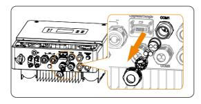
Figure 8-50 Remove the plug
