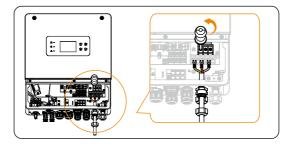
Figure 8-18 Insert the EPS cable
