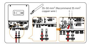
Figure 8-40 Pass and insert the cable
