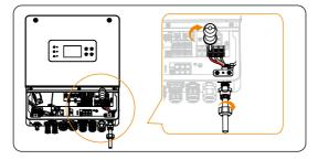
Figure 8-13 Tighten the Grid cable
