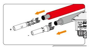
Figure 8-23 Inserting the PV pin contact
