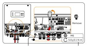
Figure 8-37 Remove the screw
