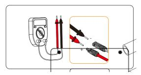
Figure 8-28 Measuring the voltage of PV connectors
