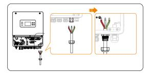
Figure 8-8 Pass the GEN cable
