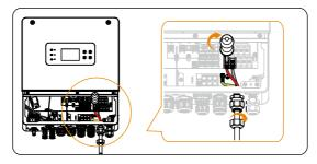
Figure 8-16 Tighten the GEN cable
