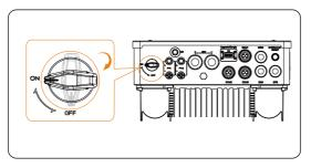
Figure 9-2 Turning on DC switch
