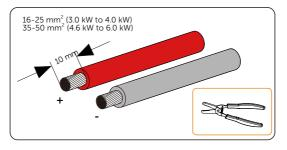
Figure 8-31 Striping the battery cable
