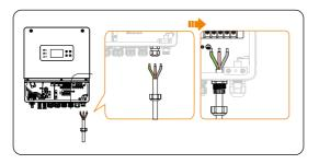
Figure 8-9 Pass the EPS cable
