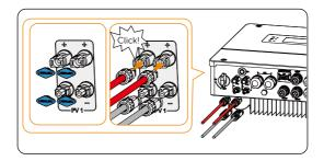
Figure 8-29 Connecting the PV cable
