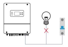
Figure 8-1 Wrong connection of load and inverter
