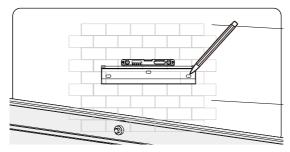
Figure 7-5 Marking the holes
