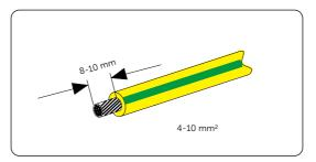
Figure 8-4 Striping the PE cable
