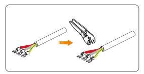
Figure 8-11 Insert and press the terminal
