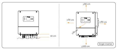
Figure 5-4 Clearance requirement for single inverter
