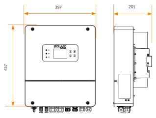
Figure 7-3 Dimensions 1 (Unit: mm)
