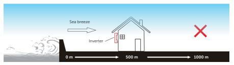
Figure 5-2 Incorrect installation position
