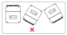
Figure 7-2 Incorrect installation
