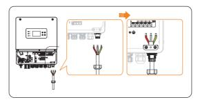
Figure 8-14 Pass the Grid cable
