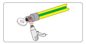
Figure 8-7 Shrinking the tubing
