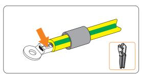
Figure 8-6 Crimping the cable
