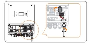
Figure 8-20 Tighten the Grid cable
