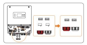
Figure 8-45 Remove the plug
