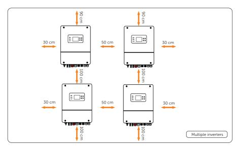
Figure 5-5 Clearance requirement for multiple inverter
