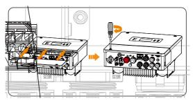
Figure 8-65 Close the lower cover and tighten the screws
