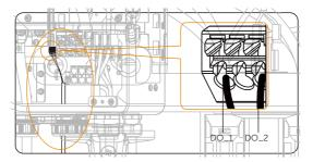
Figure 8-64 Insert the cable
