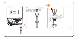
Figure 8-15 Pass the GEN cable
