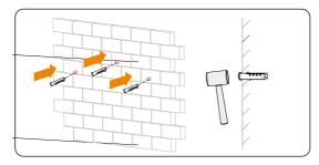
Figure 7-7 Insert the expansion tubes
