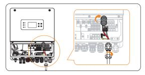
Figure 8-23 Tighten the GEN cable
