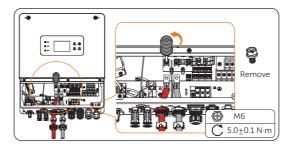
Figure 8-47 Remove the screw
