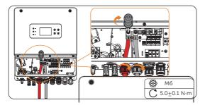
Figure 8-48 Tighten the cable
