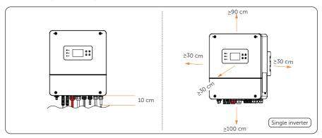
Figure 5-4 Clearance requirement for single inverter
