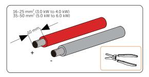
Figure 8-38 Stripping the battery cable
