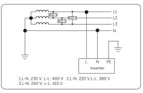
Figure 2-2 Supported power grid-TT
