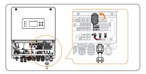
Figure 8-22 Insert the GEN cable
