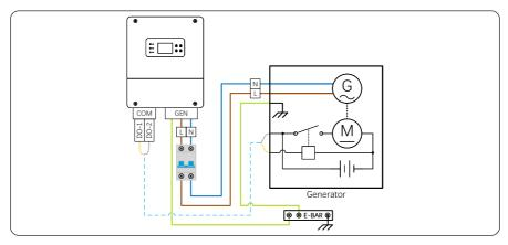
Figure 15-1 Dry contact wiring diagram
