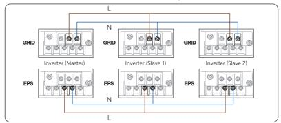
Figure 15-5 Power cable wiring
