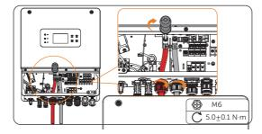
**Step 7:** Use cross screwdriver to tighten the screw. Twist to tighten the swivel nut.
