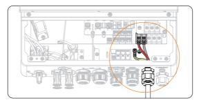
Figure 8-24 GEN cable connected
