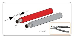
Figure 8-28 Striping the PV cable
