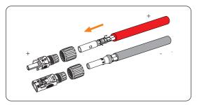
Figure 8-31 Threading the PV cable
