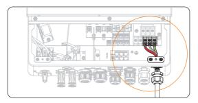
Figure 8-21 Grid cable connected
