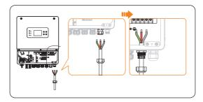
Figure 8-16 Pass the EPS cable
