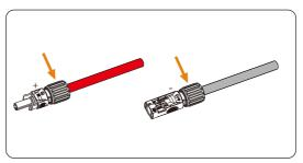
Figure 8-33 Loosening the swivel nut
