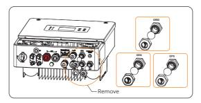
Figure 8-12 Remove the plug
