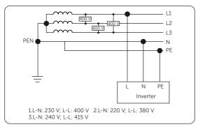
Figure 2-4 Supported power grid-TN-C-S
