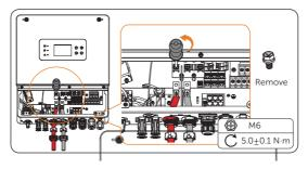
Figure 8-43 Remove the screw
