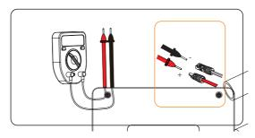
Figure 8-34 Measuring the voltage of PV connectors
