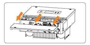
Figure 8-11 Remove the lower cover
