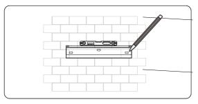
Figure 7-5 Marking the holes
