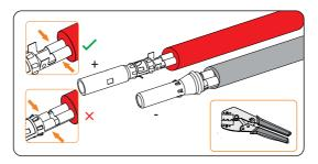
Figure 8-30 Criping the terminal
