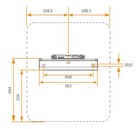
Figure 7-4 Dimensions 2 (Unit: mm)
