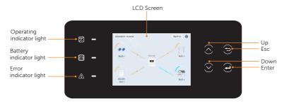
Figure 10-1 Control Panel of the inverter
