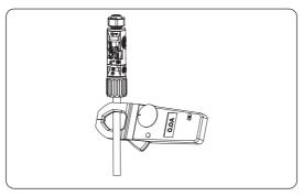
Figure 13-1 Measuring the current
