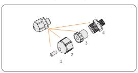
Figure 8-70 Disassembling the waterproof connector
