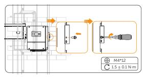
Figure 7-10 Securing the inverter
