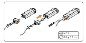
Figure 8-71 Assembling the dongle
