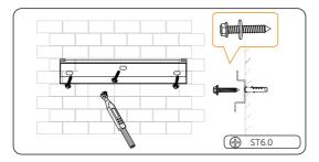
Figure 7-8 Securing the wall mounting bracket
