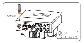
Figure 8-10 Loosen the screws
