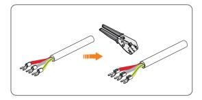
Figure 8-18 Insert and press the terminal
