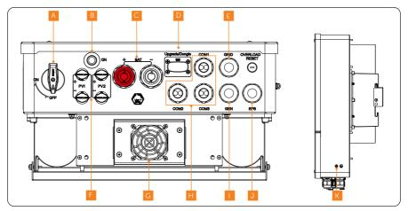
Figure 8-1 Terminals of Inverter (Bottom view)
