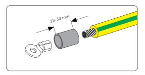
Figure 8-5 Installing the tubing and OT teriminal
