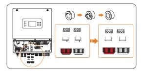
Figure 8-41 Remove the sealing cover
