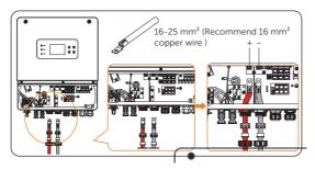
Figure 8-42 Pass and insert the cable
