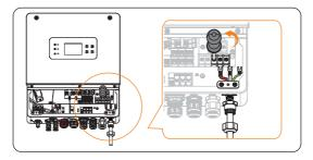
Figure 8-19 Insert the Grid cable
