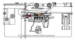
Figure 8-56 Insert the other side of the cable into the CT connection
