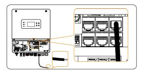
Figure 8-53 Insert one side of the cable into the inverter
