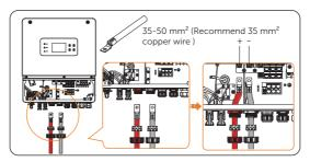
Figure 8-46 Pass and insert the cable
