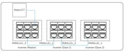
Figure 15-6 Communication wiring
