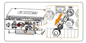
Figure 8-51 Remove the plug
