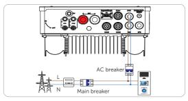
Figure 9-1 Turning on AC BREAKER
