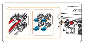
Figure 8-35 Connecting the PV cable
