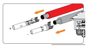
Figure 8-29 Inserting the PV pin contact
