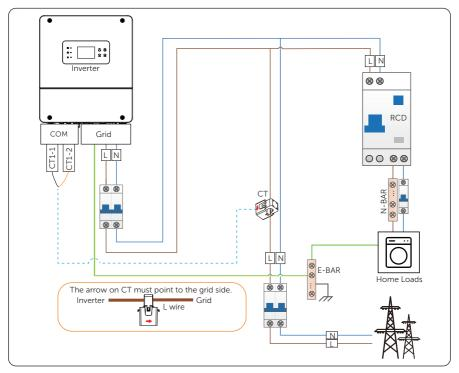
Figure 8-49 CT connection diagram
