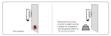
Figure 5-3 Installation carrier requirement
