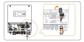
Figure 8-26 Tighten the EPS cable
