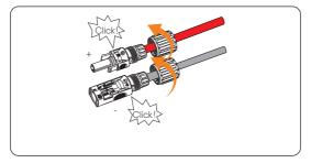
Figure 8-32 Securing the swivel nut
