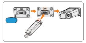
Figure 8-69 Dongle connection procedure
