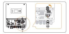
Figure 8-25 Insert the EPS cable
