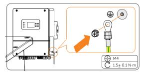
Figure 8-8 Securing the PE cable
