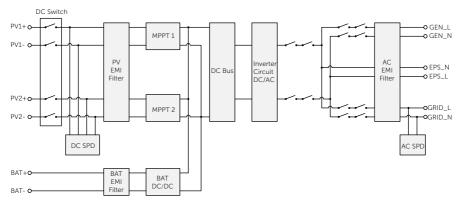
Figure 2-5 Circuit Diagram for X1-HYB-LV series inverter
