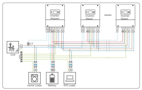
15.2.3 System wiring diagram
