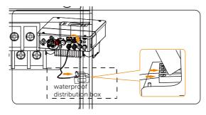
Figure 8-54 Insert the other side of the cable into the waterproof distribution box
