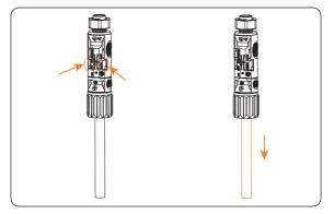
Figure 13-2 Disassembling the PV cables
