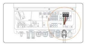
Figure 8-27 EPS cable connected
