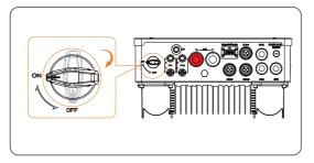
Figure 9-2 Turning on DC switch
