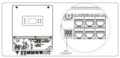
Figure 15-2 Connection terminal for generator
