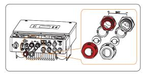
Figure 8-40 Connecting the battery connector
