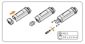
Figure 8-68 Assembling the dongle
