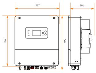
Figure 7-3 Dimensions 1 (Unit: mm)
