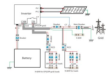
Diagram B: Neutral line and PE line are separated from each other, all loads connect to the EPS(Off-grid) port; (For most countries)
