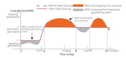
The D-A period is the battery charging period during which discharging is not allowed and the PV will charge the battery first for peak shaving. The ChargeFromGrid" setting determines whether or not to charge from the grid. When "ChargeFromGrid" is set to "Disable", the battery cannot charge from the grid; when "ChargeFromGrid" is set to "Enable" and the actual battery SOC is less than "Max\_SOC", the battery will charge from the grid at no more than "ChargePowerLimits" power.
