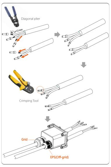
**Step 4.** Find the location of the AC interface on the inverter, insert the crimped terminals into the UW10 terminals L, N, and P according to the wire sequence, and use a flat-blade screwdriver to tighten the screws. (Torque:  $1.5\pm0.1~\rm N\cdot m$ )
