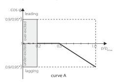
\*) If the grid-connected power of the inverter ≤ 4.6kW, the Power Factor is 0.95 at 1.0 power; if the grid-connected power of the inverter > 4.6kW, the Power Factor is 0.90 at 1.0 power.
