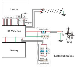
Diagram C: Neutral line and PE line are combined together, and the common load is connected to the EPS(Off-grid) port;
