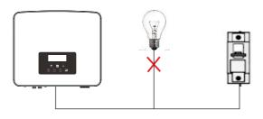
Figure: Wrong connection of load and inverter
