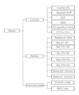
★ Register1 SN: Represents the serial number of external monitoring equipment, such as WiFi Dongle, LAN Dongle and GPRS Dongle.
