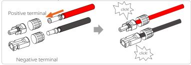
**Step 6.** Tighten the fastening head and insert into the corresponding positive and negative (BAT-/BAT+) ports of the inverter.
