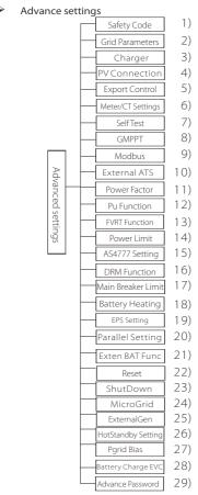
All advanced settings can be set here, such as battery, grid, EPS(Off-grid), etc.. "Advanced" setting is generally customization and resetting for battery and grid. Each part has lower level parts.
