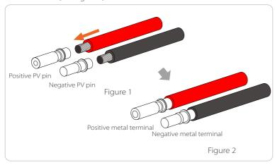
**Step 4.** Tighten the PV pin contact and the wiring harness to make the connection tight without looseness
