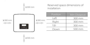
For multi-inverter installation scenarios, the inline installation method is recommended; when the space is insufficient, the recommended method of installation in the form of "products"; it is not recommended to install multiple inverters in stacks. If you choose stack installation, please refer to the installation separation distance below.
