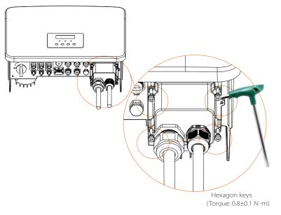
Step 6. Tighten the waterproof fastening head.
