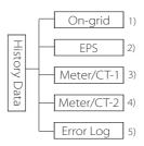
The history data contains five pieces of information: on-grid power of the inverter, EPS power generation, power of the meter/CT and error logs.
