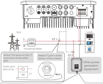
If the user has other power generation equipment (such as inverter) at home and wants to monitor both, X1-Hybrid G4 inverter provides CT2 communication function to monitor the power generation equipment. For more information, please contact us.
