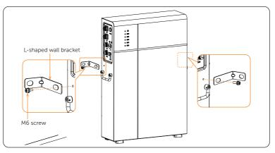
Figure 6-2 Fixing L-shaped wall bracket to the battery module
