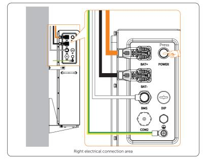
Step 1: Press the POWER button to shut down the system before unplugging.
