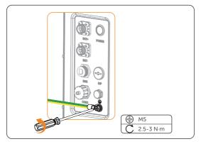
**Step 4:** Unscrew the screws counter-clockwise to remove the grounding cable.
