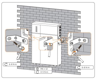
Figure 6-17 Tightening tapping screws and M6 screws
