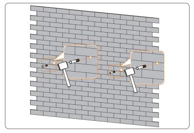
**Step 5:** Insert the expansion bolt (Part H) (x 2 pcs) into the two holes.
