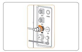
Figure 10-3 Removing communication cable
