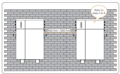
**Step 10:** Repeat steps 1 to 9 to install the second battery module, as well as the remaining battery modules (if any).
