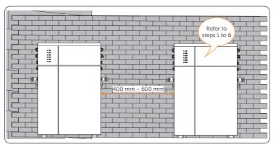
Figure 6-8 Installing the remaining battery module
