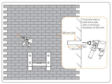
Figure 6-15 Drilling holes
