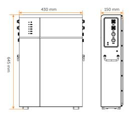
Figure 2-2 Dimension: Battery module (TP-LD53)
