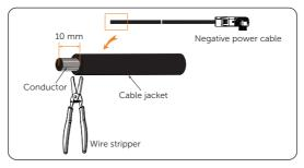
Figure 7-7 Stripping power cable
