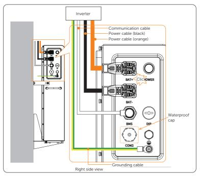
Figure 7-20 Cable connection of the right electrical connection area
