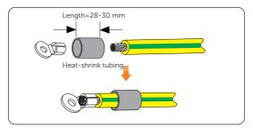
Figure 7-2 Cutting heat-shrink tubing
