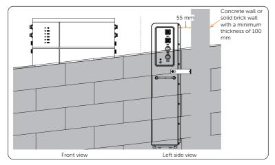
**Step 2:** Locate the L-shaped wall bracket against the wall.
