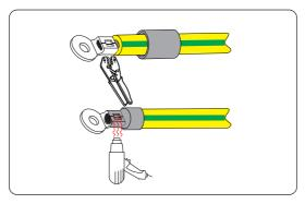
Figure 7-3 Crimping and heating
