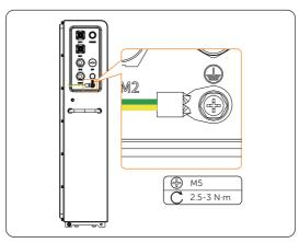
Figure 7-4 Tightening M5 screws
