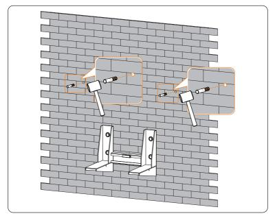
**Step 8:** Insert the expansion bolt (Part H) (× 2 pcs) into the two holes.
