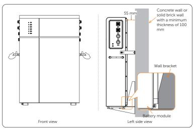
Figure 6-13 Lifting the battery module
