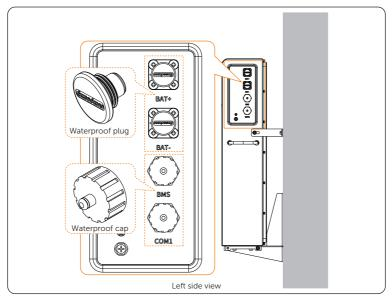
Figure 7-18 Left electrical area of the battery module
