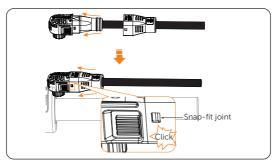
Figure 7-14 Assembling connector
