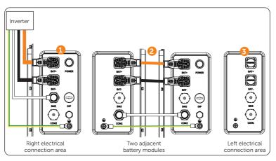
Figure 7-19 Wiring diagram of two battery modules
