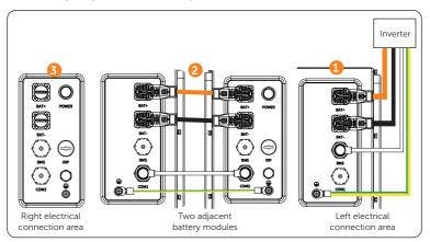
Figure 7-25 Wiring diagram of two battery module
