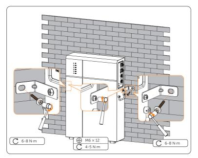
Figure 6-7 Tightening tapping screws and M6 screws
