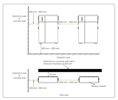
Figure 4-3 Clearance requirement about wall mounting
