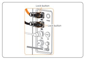
Figure 10-2 Unplugging power cables
