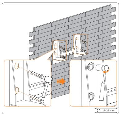
Figure 6-11 Tightening expansion screw
