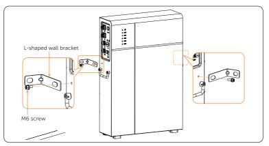
Figure 6-12 Fixing L-shaped wall bracket to the battery module
