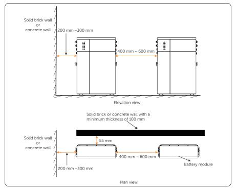
Figure 4-2 Clearance requirement about floor mounting
