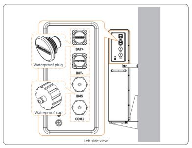
Figure 7-22 Left electrical area of the battery module
