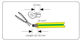
Figure 7-1 Striping cable jacket
