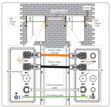
Figure 7-27 Cable connection of two adjacent battery module
