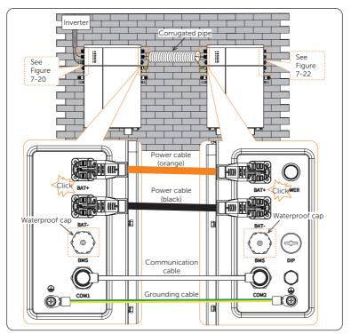
Figure 7-21 Cable connection between adjacent battery module
