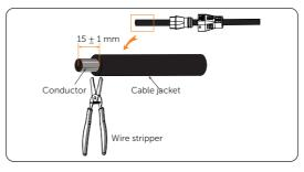
Figure 7-12 Striping cable jacket
