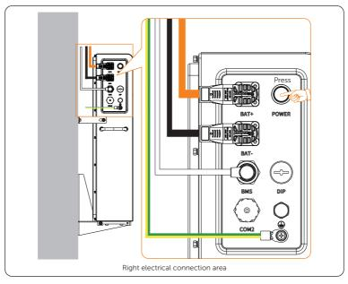
Figure 8-1 Power on/off the system
