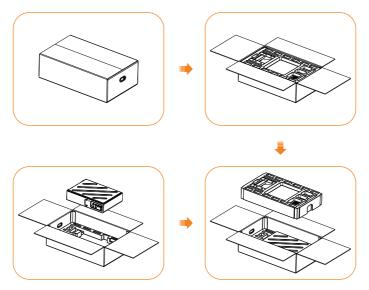
Figure 5-1 Unpacking the battery module
