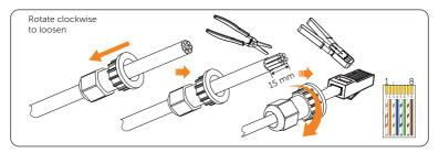
Figure 7-6 Making RJ45 connector to communication cable
