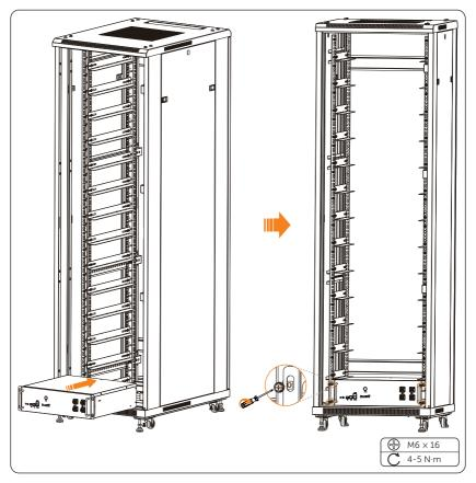
Figure 6-18 Placing battery modules and tightening M6 screws
