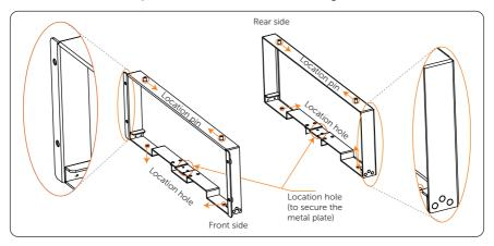
Figure 6-2 Placing the supports
