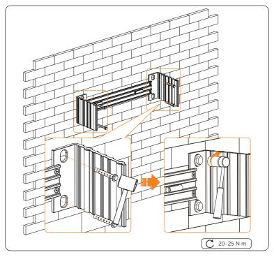
Figure 6-23 Tightening expansion screw
