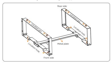
Figure 6-3 Inserting metal plate
