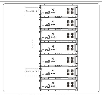
Figure 6-10 Placing the remaining battery modules
