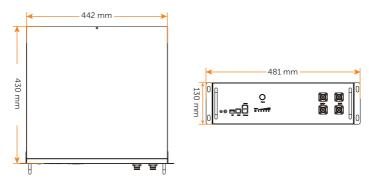
Figure 2-2 Dimension: Battery module (T-BAT LR25/ T-BAT LR36)
