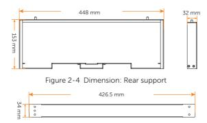
Figure 2-5 Dimension: Metal plate
