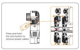
Figure 10-2 Unplugging power cables
