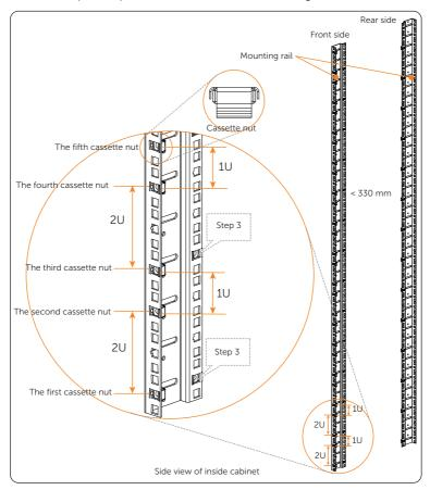
Figure 6-15 Inserting cassette nuts
