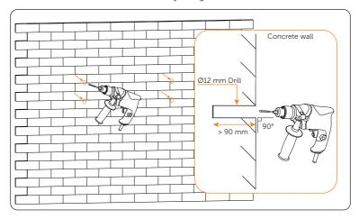
Figure 6-22 Drilling holes
