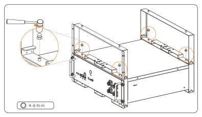
Figure 6-7 Tightening cap nuts
