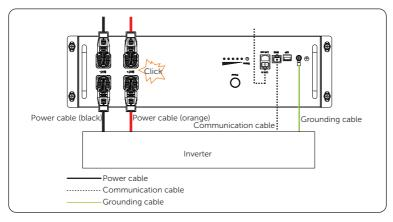
Figure 7-13 Connecting cables between the battery module and the inverter
