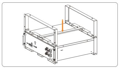
Figure 6-8 Placing the metal plate
