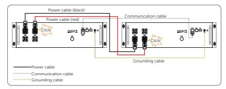
Figure 7-12 Cable connection between battery modules
