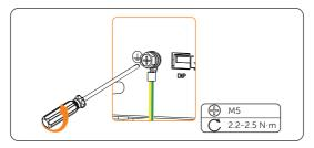
Figure 10-4 Removing grounding cable
