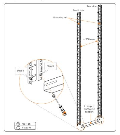
Figure 6-16 Attaching I-shaped transverse support and tightening M6 screws
