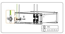
Figure 7-4 Tightening M5 screws
