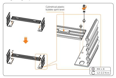
Figure 6-20 Securing I-shaped wall brackets and transverse plate
