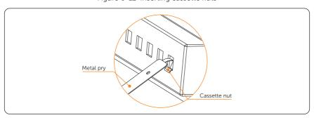
Figure 6-13 How to use a metal pry
