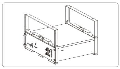
Figure 6-6 Placing front-side and rear-side supports
