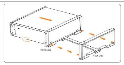
Figure 6-4 Placing the battery module into the rack
