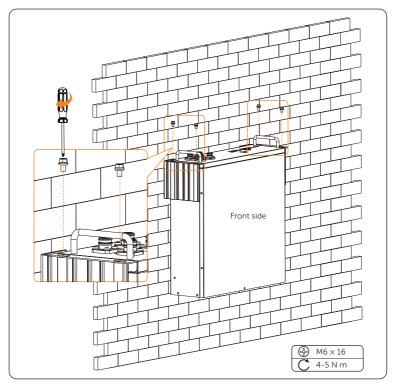
Figure 6-25 Tightening M6 screws
