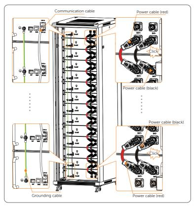
Figure 7-9 Cable connection between battery modules
