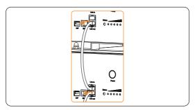
Figure 10-3 Removing communication cable
