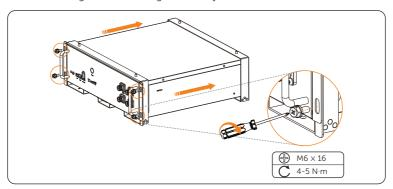
Figure 6-5 Tightening M6 screws
