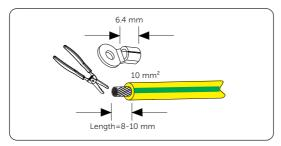
Figure 7-1 Striping cable jacket
