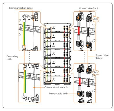
Figure 7-7 Cable connection between battery modules
