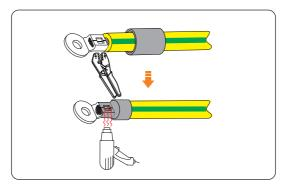
Figure 7-3 Crimping and heating
