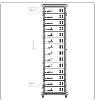
**Step 8:** Repeat step 6 to place the remaining battery modules. See figure below.
