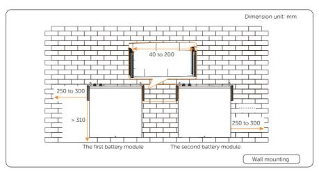
Figure 4-1 Clearance requirement
