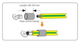
Figure 7-2 Cutting heat-shrink tubing
