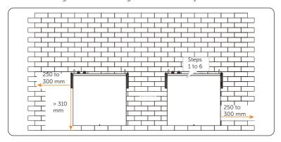
Figure 6-27 Installing other battery modules
