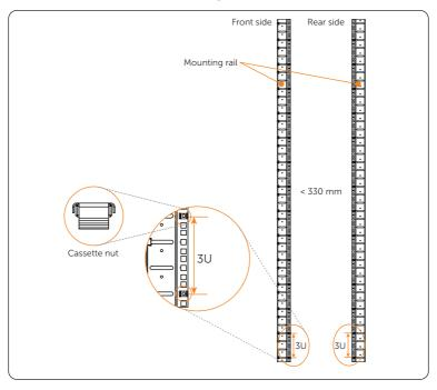
Figure 6-14 Inserting cassette nuts
