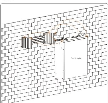
**Step 5:** Gently place the battery module on the assembled wall bracket and align the holes.
