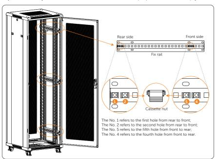
**Step 2:** Correctly insert cassette nuts into the fix rails via proper use of a metal pry.
