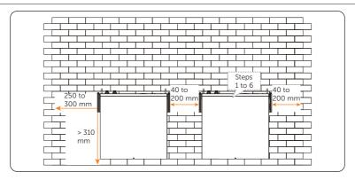
Figure 6-26 Installing the second battery module
