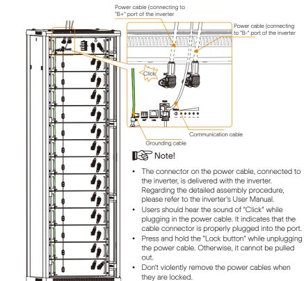
• The "Link port" on the battery management system (BMS) is for parallel connections only. Don't use it
