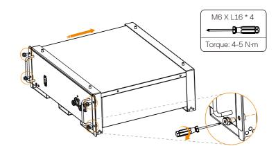
Step 3. Add the rack and battery module
