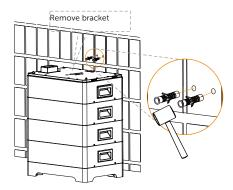
Secure the assembled bracket to the wall with Self-tapping screw (Part H) ( $\times$  2 pcs) and Washer (Part G) ( $\times$  2 pcs), and tighten them (Torque: 4 N·m);
