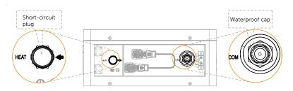
\*Note: In case of one tower, a waterproof cap shall be put on the unconnected "COM" port, as well as a short-circuit plug on the unconnected "HEAT" port.
