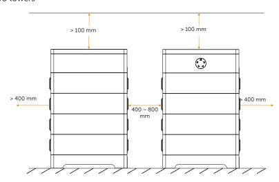
\*Note: The above figures show an example of installation space of "One Tower" and "Two Towers".
