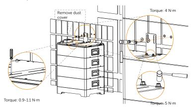
Step 8. Place BMS, and tighten M4x14 Phillips-head screw (Part L) ( $\times$  4 pcs) and gasket (Part K) ( $\times$  4 pcs) on both sides (Torque: 0.9 to 1.1 N·m)
