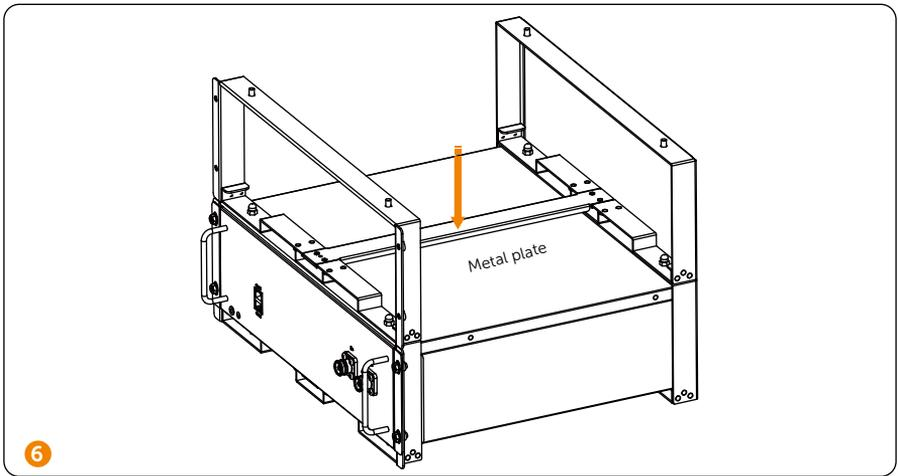
Gently place the battery into the rack, and tighten 4 M6 screws
