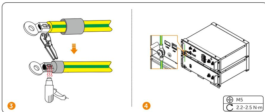
In case of a rated current of 30 A, the wire size of 5.5-6.5 mm<sup>2</sup> for cables (including grounding cable) is recommended; in case of a rated current of 45 A, the wire size of 8.5-9.5 mm<sup>2</sup> for cables (grounding cable) is recommend.
