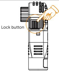
The terminal connector (see left figure) is on the power cable.
