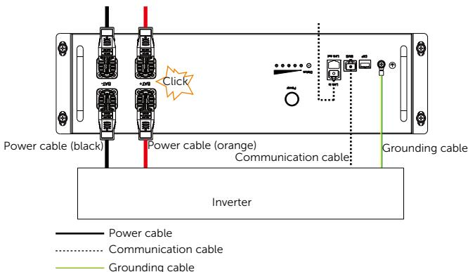
The terminal connector (see left figure) is on the power cable.
