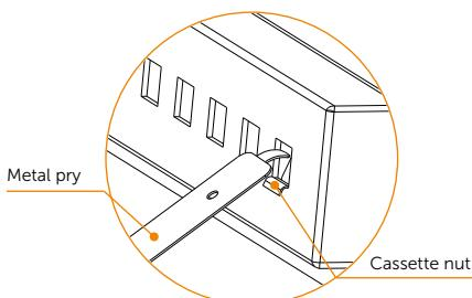
A metal pry can be used while inserting or removing cassette nuts.
