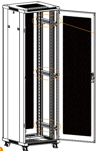
Cassette nuts shall be inserted before installing fixed rails. There are totalling 3 fixed rails on each left and right side. 4 cassette nuts shall be inserted into each fixed rail.
