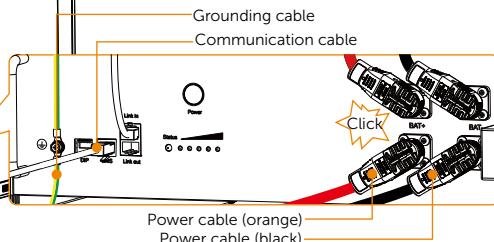
The terminal connector (see left figure) is on the power cable.
