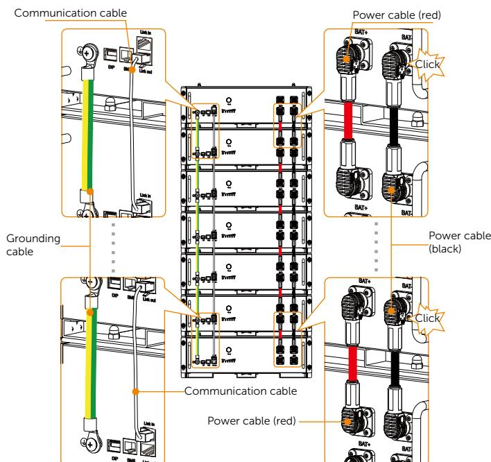
The terminal connector (see left figure) is on the power cable.
