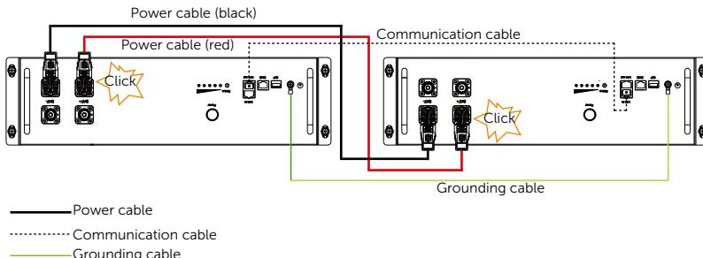
The terminal connector (see left figure) is on the power cable.
