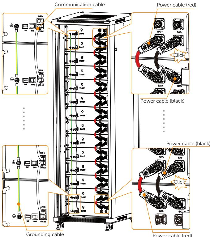
The terminal connector (see left figure) is on the power cable.
