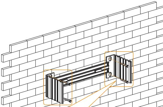
A total of 4 expansion screws shall be inserted.
