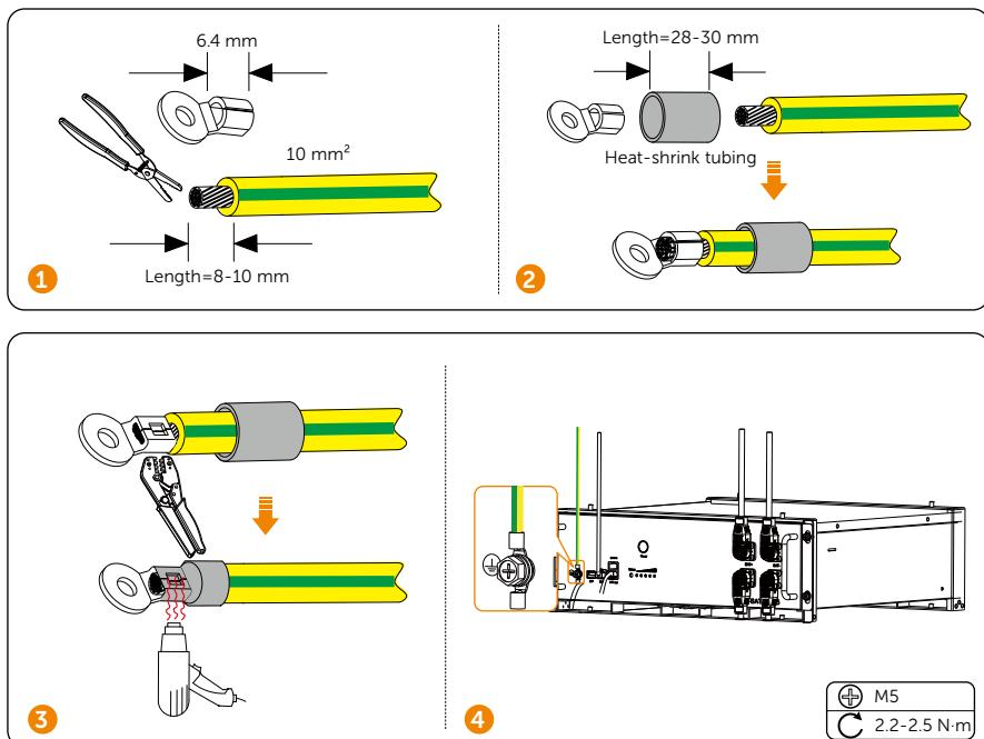
Regarding the cables that are prepared by the users themselves, the wire size of  $10\text{ mm}^2$  for cables is recommend.
