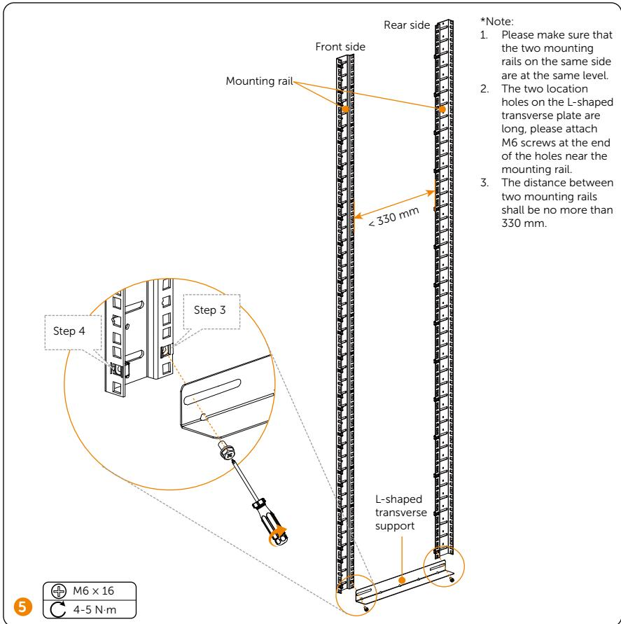
After all I-shaped transverse supports are secured, attach the assembled mounting rails into the cabinet, and tighten screws to fasten mounting rail and fix rail.
