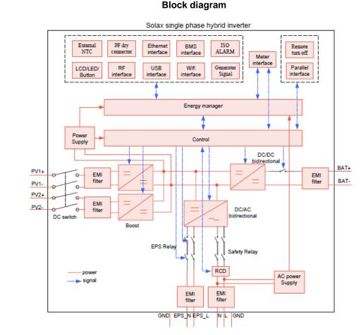
The internal control is redundant built, It consists of master controller(U2-A) and slave controller(U2-B), the master controller(U2-A) can control relays, measures voltage, frequency, AC current with injected DC, insulation resistance and residual current. The slave controller (U2-B) can control the relays, measures the voltage and frequency. Both controllers communicate with each other.
