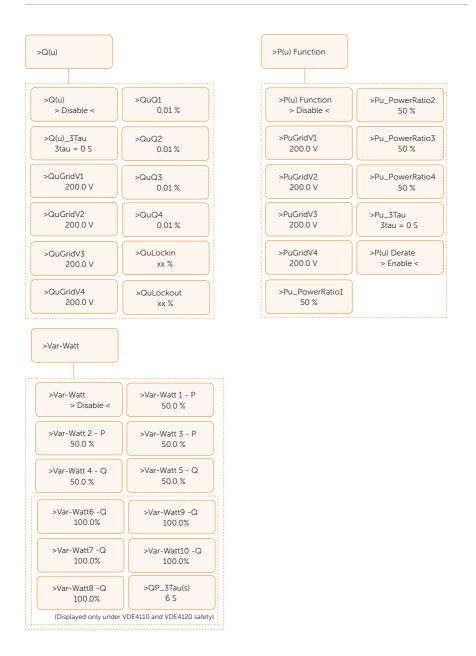
Usually end user do not need to set the grid protection. All default value have been set before leaving factory according to safety rules. If reset is needed, any changes should be made according to the requirements of local grid.
