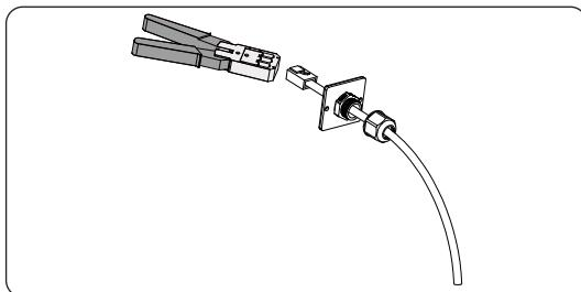
Figure 6-27 Crimp the RJ45 terminal
