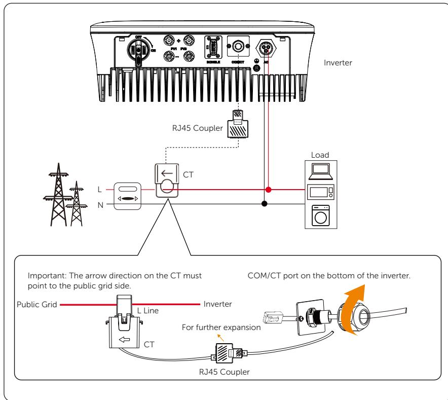
Figure 6-32 CT connection diagram
