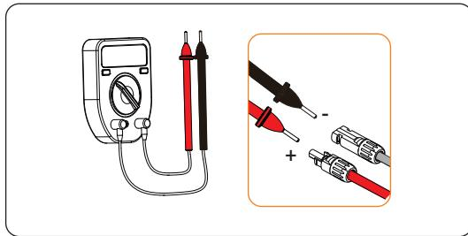
Figure 6-21 Measuring the voltage of PV connectors
