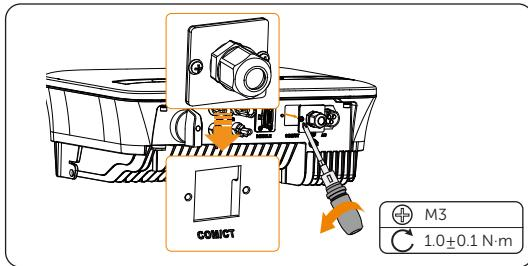
Figure 6-33 Disassemble COM/CT port
