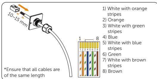
Figure 6-26 Insert the communication cable
