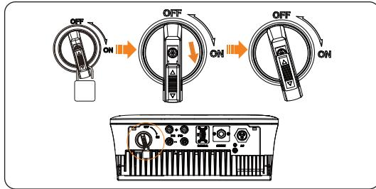
Figure 7-46 Unlock DC switch
