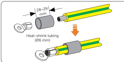
Figure 6-4 Installing the tubing and OT terminal
