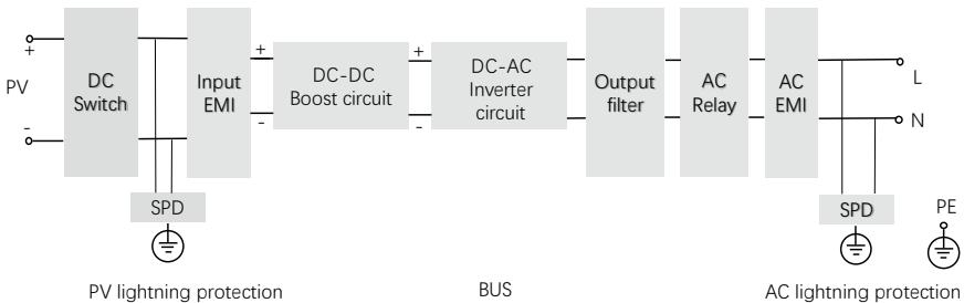
Figure 2-5 Circuit diagram for X1-BOOST G4 series inverter
