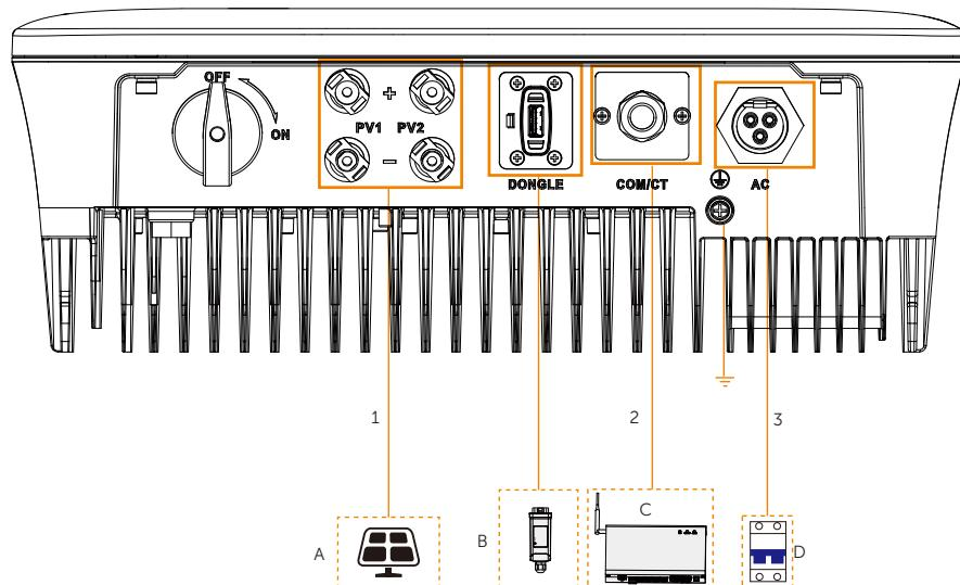
Figure 6-2 Cable connections of inverter
