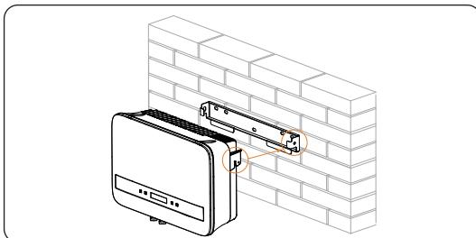
Figure 5-8 Mounting the inverter
