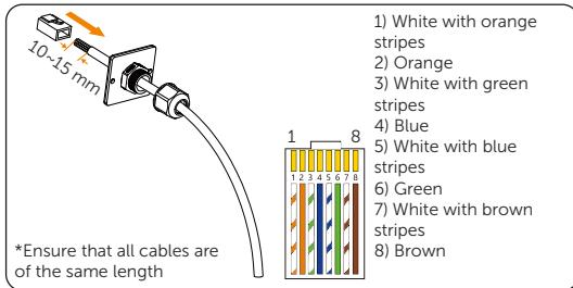
Figure 6-34 Insert the communication cable
