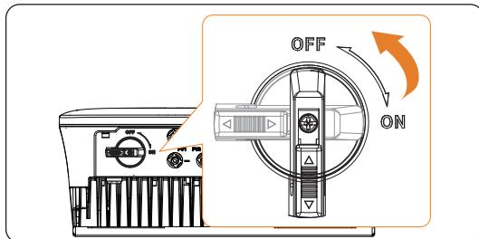
Figure 7-44 Turn off DC switch
