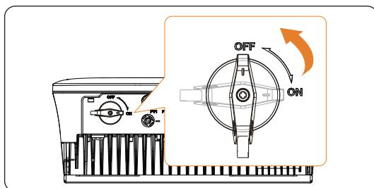
Figure 7-50 Turn off DC switch
