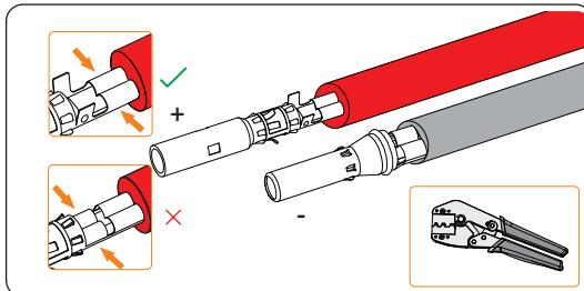
Figure 6-18 Crimping the terminal
