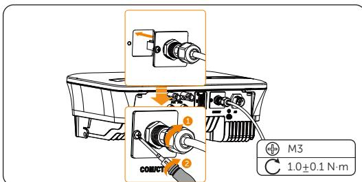
Figure 6-28 Insert the terminal into COM/CT port
