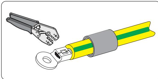
Figure 6-5 Crimping the cable
