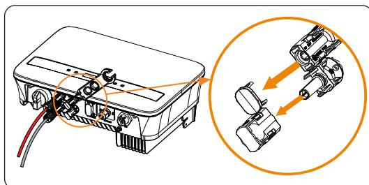
Figure 11-1 Disassemble the dust-proof buckles
