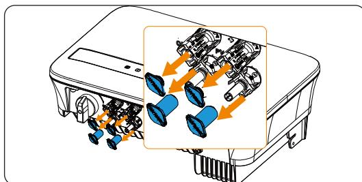
Figure 6-22 Remove the PV terminal caps
