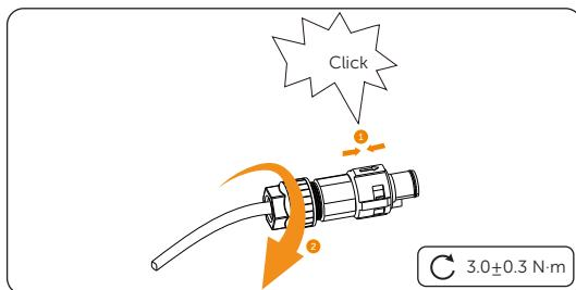
Figure 6-14 Screw down component 1
