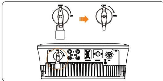
Figure 7-52 Unlock DC switch
