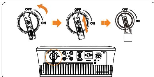
Figure 7-45 Lock DC switch
