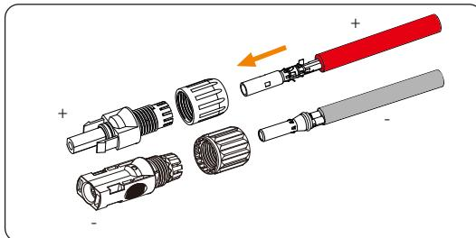
Figure 6-19 Threading the PV cable
