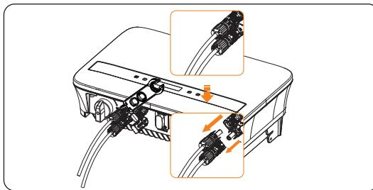
Figure 11-2 Releasing the PV connector
