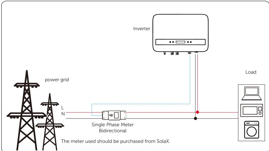
Figure 6-30 Wiring diagram-meter without CT
