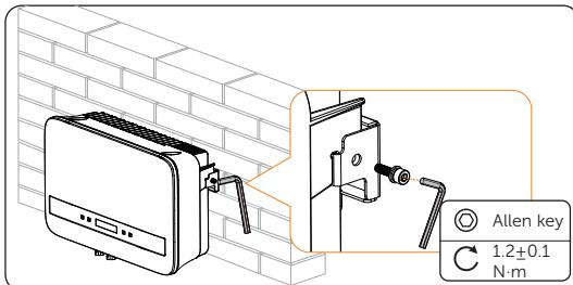
Figure 5-9 Securing the inverter
