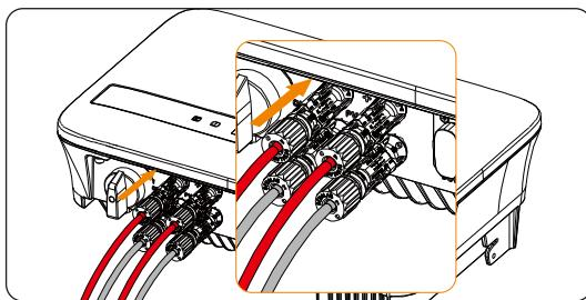
Figure 6-23 Connecting the PV cable
