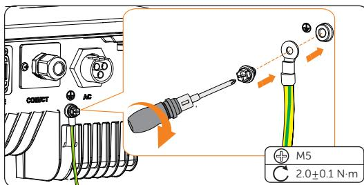
Figure 6-8 Securing the PE cable
