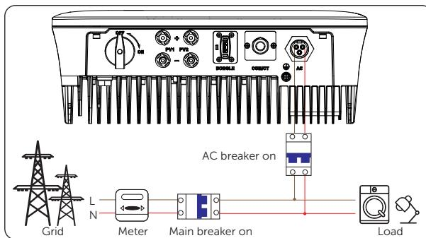
Figure 7-40 Turn on the AC breaker
