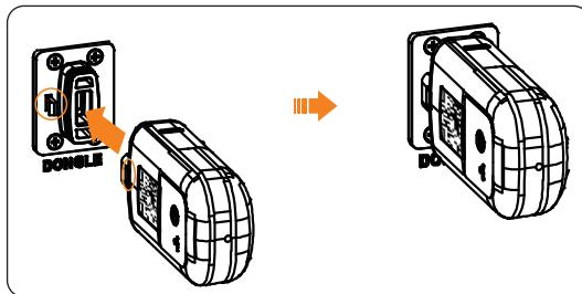
Figure 6-38 Dongle connection procedure
