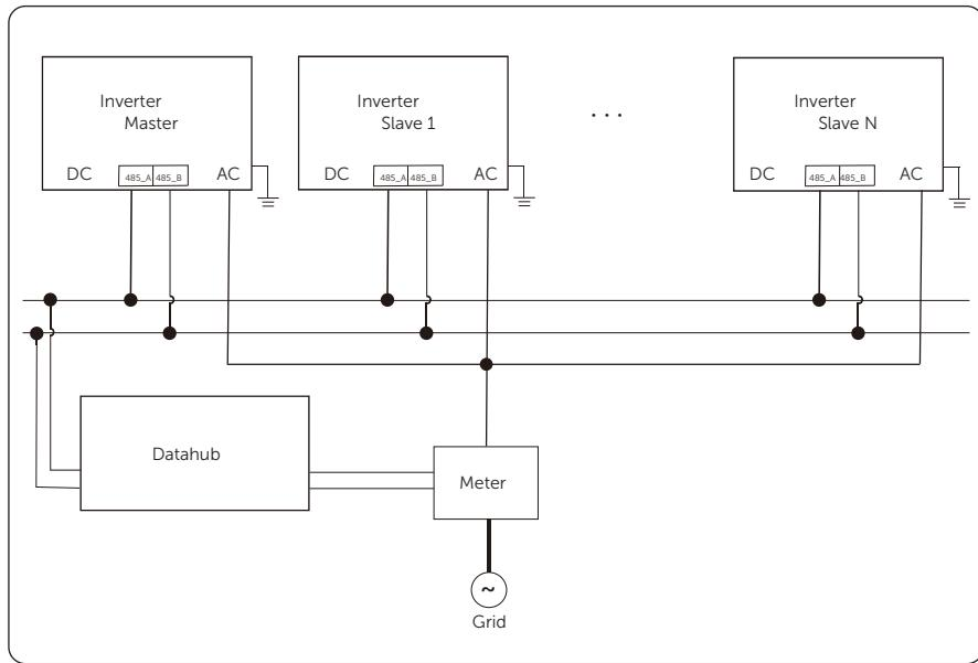
Figure 13-5 Wiring diagram-parallel system with DataHub
