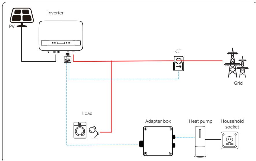
Figure 13-1 Adapter Box G2 wiring diagram
