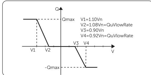
Figure 8-4 Curve  $Q = f(V)$
