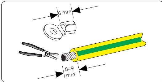
Figure 6-3 Stripping the PE cable
