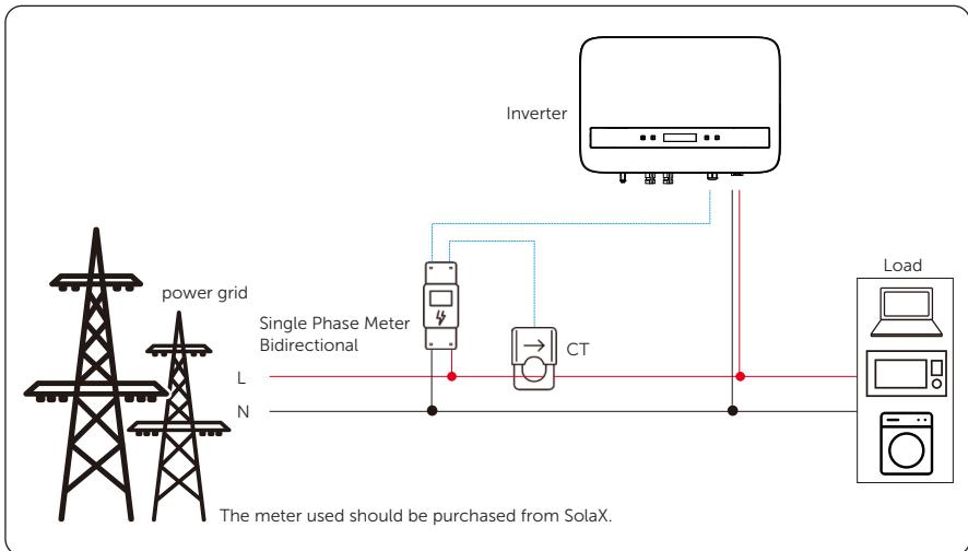
Figure 6-29 Wiring diagram-meter with CT
