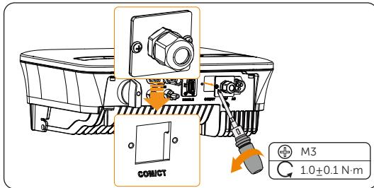
Figure 6-25 Disassemble COM/CT port
