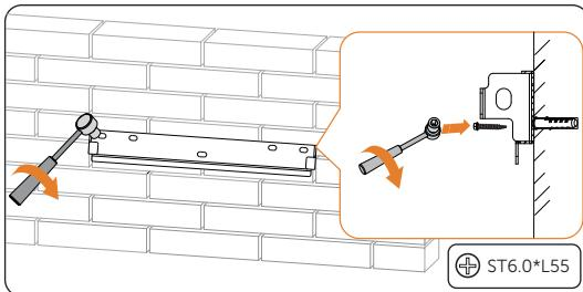
Figure 5-7 Securing the wall mounting bracket
