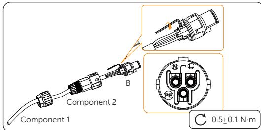
Figure 6-13 Insert wires in to the corresponding holes
