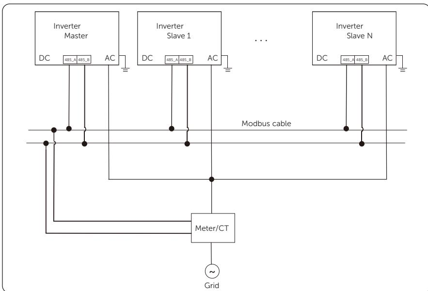
Figure 13-4 Wiring diagram-parallel system with modbus function
