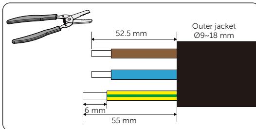
Figure 6-9 Strip the L, N, PE wires
