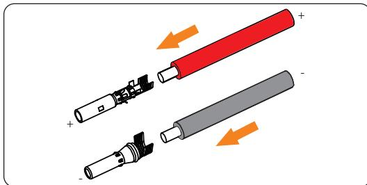
Figure 6-17 Inserting the PV pin contact
