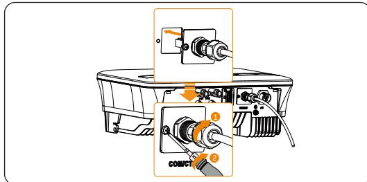
Figure 6-36 Insert the terminal into COM/CT port
