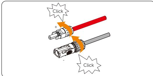
Figure 6-20 Securing the PV cable
