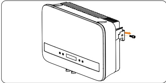
Figure 11-5 Unscrewing the M5 screws
