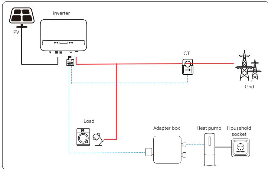
Figure 13-1 Adapter box wiring diagram
