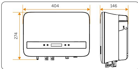
Figure 5-3 Dimensions 1 (Unit: mm)
