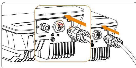
Figure 6-15 Connect AC plug to the inverter
