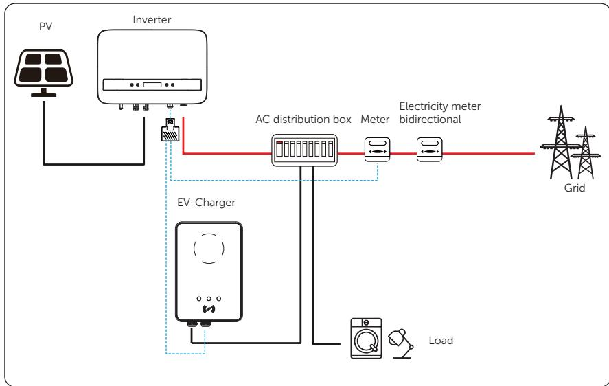
Figure 13-3 EV-Charger wiring diagram
