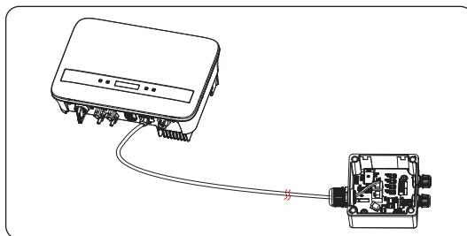
Figure 13-2 Adapter Box G2 connection
