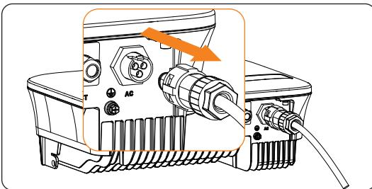
Figure 11-4 Releasing the AC connector
