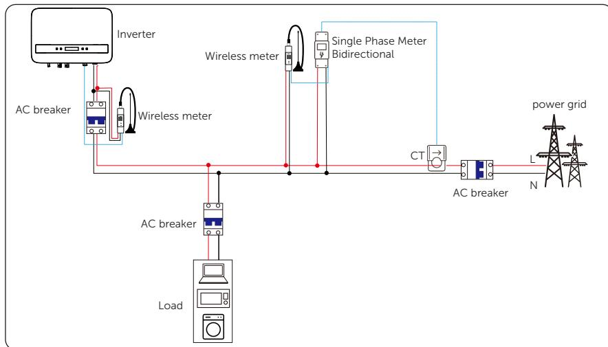
Figure 6-31 Wiring diagram-wireless meter
