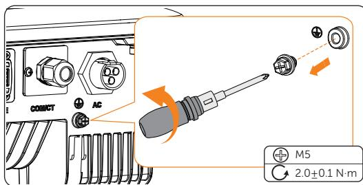
Figure 6-7 Uninstalling the screw
