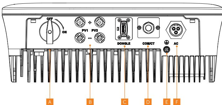
Figure 6-1 Terminals of Inverter
