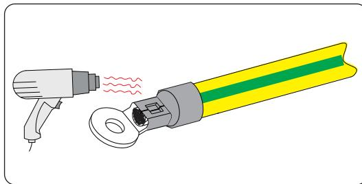
Figure 6-6 Shrinking the tubing
