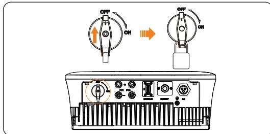
Figure 7-51 Lock DC switch
