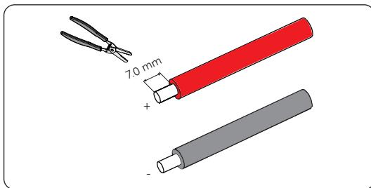
Figure 6-16 Stripping the PV cables
