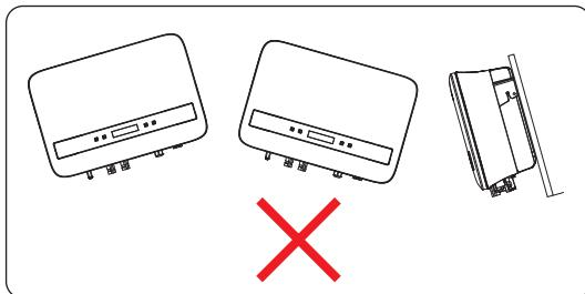
Figure 5-2 Incorrect installation
