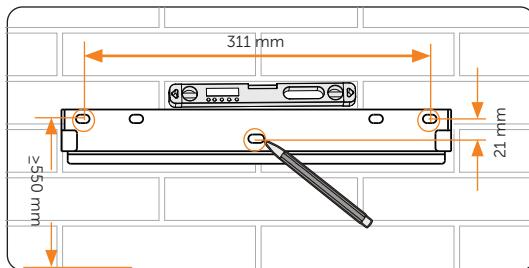
Figure 5-5 Marking the holes
