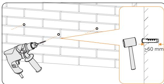
Figure 5-6 Drilling holes (Unit: mm)
