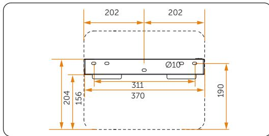
Figure 5-4 Dimensions 2 (Unit: mm)
