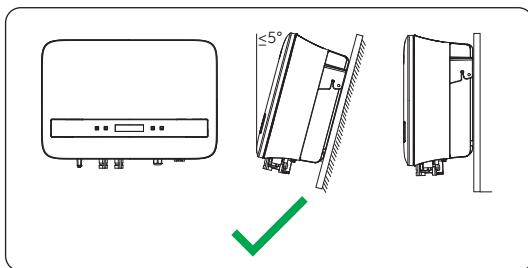
Figure 5-1 Correct installation
