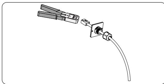
Figure 6-35 Crimp the RJ45 terminal
