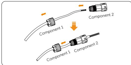
Figure 6-12 Slide component 1&2 on to AC cable
