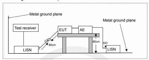
LISN: Line Impedance Stabilization Network
