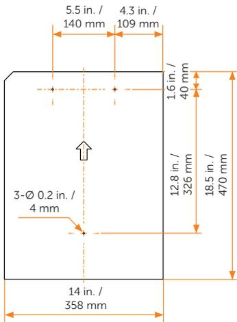
Figure 4-5 Dimensions of mounting template
