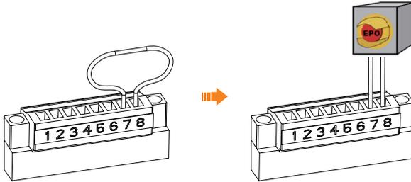
Figure 5-14 Emergency stop switch connection
