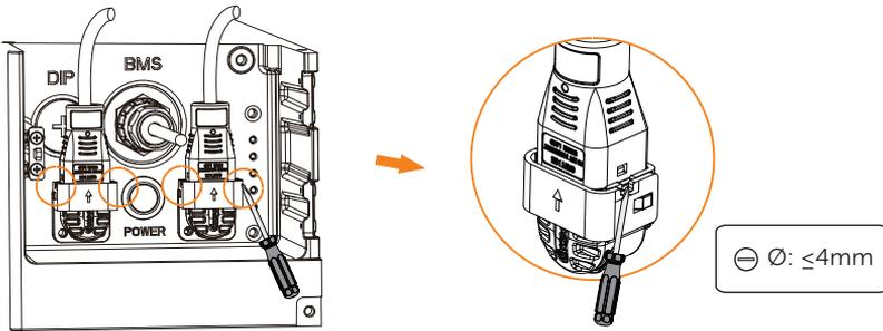
Figure 5-18 Pry open the buckles
