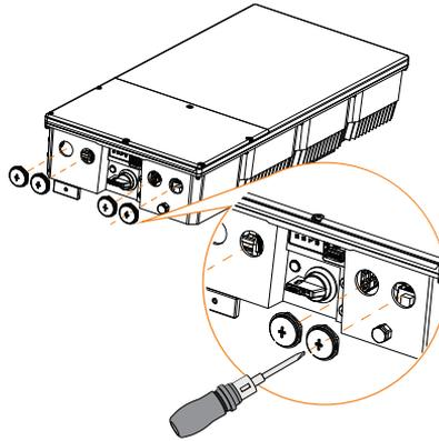
Figure 5-3 Remove the wiring box waterproof plugs
