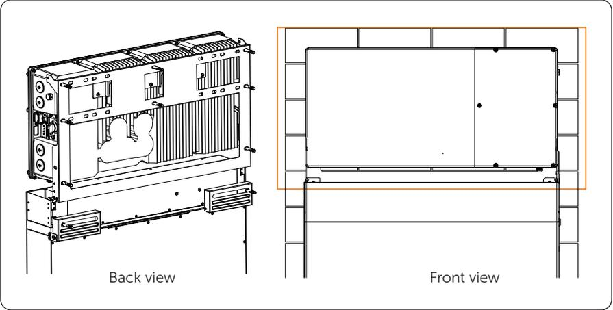
**Step 7:** Place the protective guard [Inverter (part F)] on the correct position of battery's BMS prior to the wiring connection between inverter and battery and fix it with the inverter bracket with M5 screws [Inverter (part C)].
