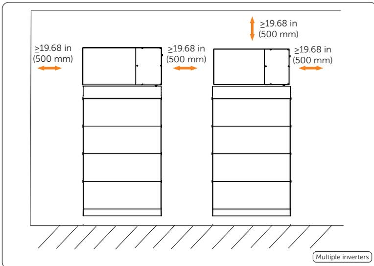
Figure 3-3 Clearance requirement for multiple inverters
