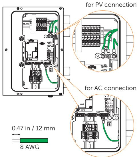
Figure 5-6 GND cable connection
