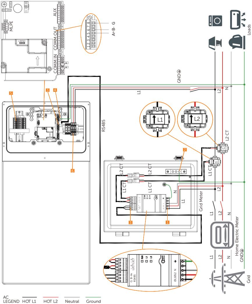
Figure 5-20 Electrical Connection Diagram A
