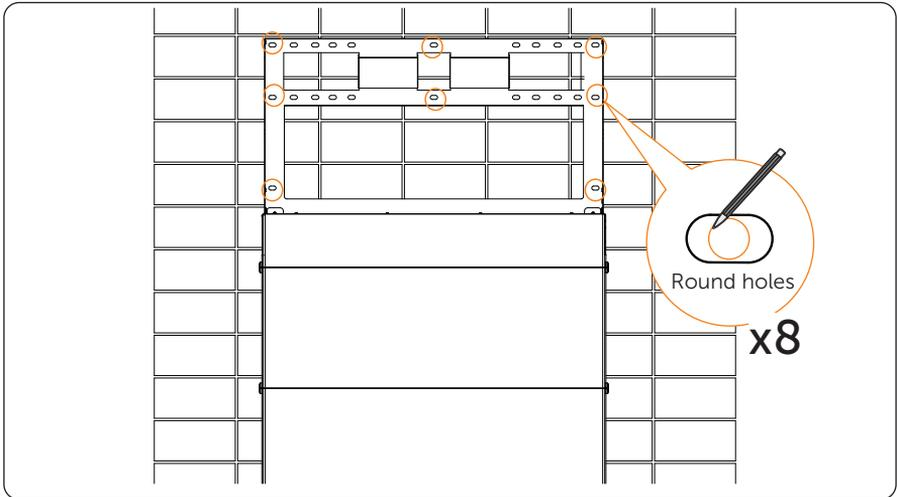
**Step 3:** Unscrew the two M4 screws to disassemble the bracket. Drill holes with power drill, and make sure the holes are deep enough (2.16 in / 55 mm) to support the inverter.
