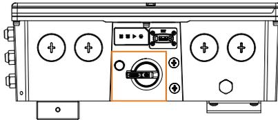
Figure 5-1 Turning DC switch to "OFF"
