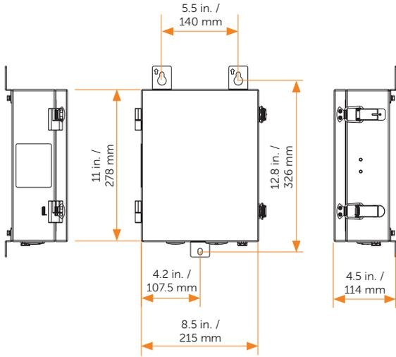
Figure 4-4 Dimensions of meter box
