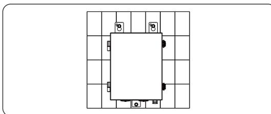
Figure 4-11 Fixing the meter
