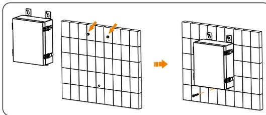
Figure 4-10 Seating the meter and securing the screw
