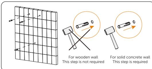
Figure 4-8 Inserting expansion holes
