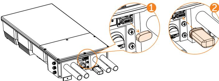
Figure 5-15 Monitoring Connection
