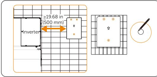
Figure 4-6 Marking the holes
