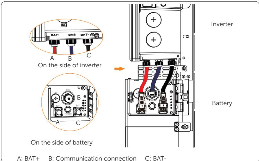
Figure 5-17 Battery connection
