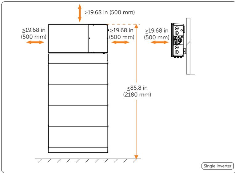
Figure 3-2 Clearance requirement for single inverter
