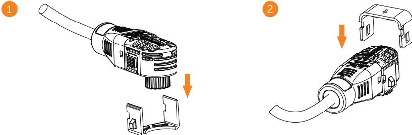
Figure 5-19 Reinstall the buckles
