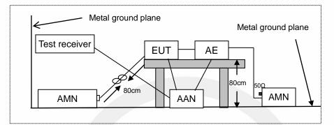
AMN: Artificial mains network AE: Associated equipment EUT: Equipment under test AAN: Asymmetric artificial network
