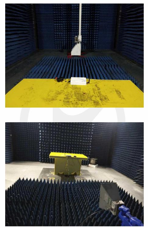
8.4. Photo of Radiation Emission Measurement (Above 1GHz)
