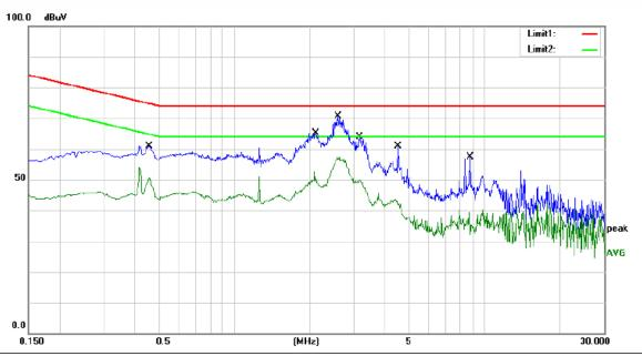
Site site #1 Temperature: 24 Phase: Limit: (CE)AS/NZS CISPR 32 Class B TELECOM\_QP Power: AC 240V/50Hz Humidity:
