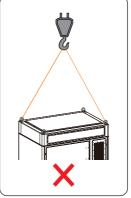
Figure 6-4 Improper way of hoisting
