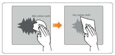
Figure 14-5 Cleaning the scratched area
