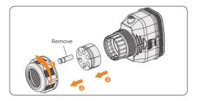
Figure 7-32 Disassembling the connector
