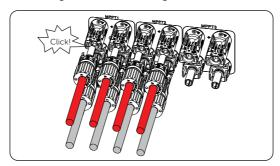
Figure 7-22 Connecting assembled PV cables to the inverter
