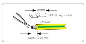
Figure 7-3 Striping cable jacket
