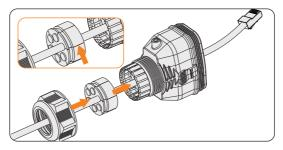
Figure 7-50 Threading the cable with RJ45 terminal
