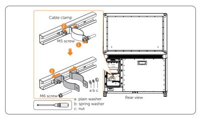
Figure 7-81 Unscrewing M6 screw
