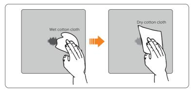
Figure 14-2 Cleaning the scratched area
