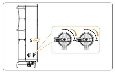
Figure 8-8 Starting the inverter
