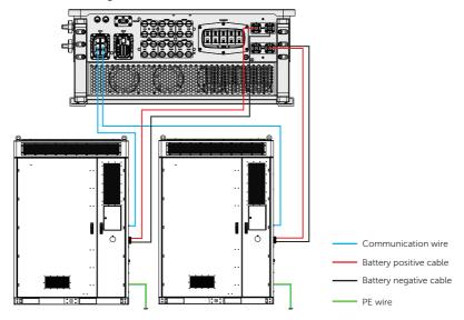
Figure 7-39 BMS connection diagram
