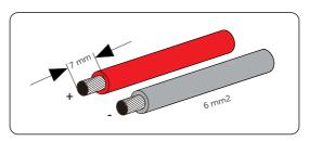
Figure 7-15 Striping the PV cable
