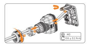
Figure 7-38 Securing the connector
