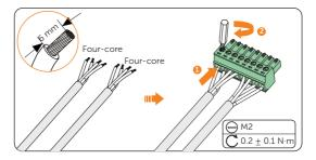
Figure 7-59 Connecting to 8-pin terminal block
