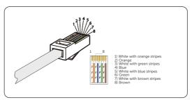
Figure 7-44 Crimping the communication cable
