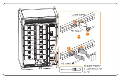
Figure 7-67 Unscrewing M6 screw
