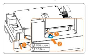
Figure 6-25 Installing the eye bolts
