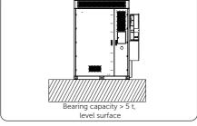
Figure 4-2 Foundation requirement
