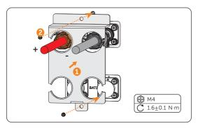
Figure 7-29 Installing the battery protective cover
