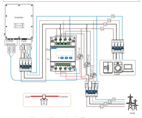
Figure 14-14 System wiring with CT-connected meter
