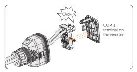
Figure 7-37 Inserting the connector to COM 1
