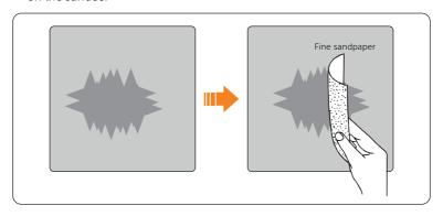
Figure 14-4 Sanding the scratched area
