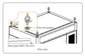
Figure 6-4 Tightening eye bolts
