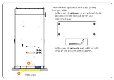
Figure 7-84 Threading grid wires
