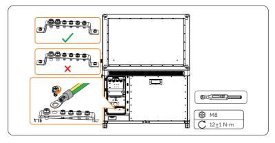
Figure 7-88 Connecting PE wire
