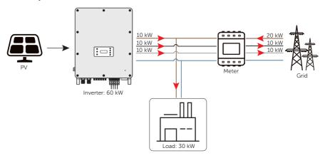
Figure 2-31 Zero export control with Phase Unbalance disabled
