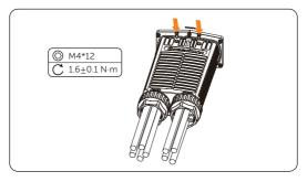
Figure 7-13 Securing the AC connector on the inverter
