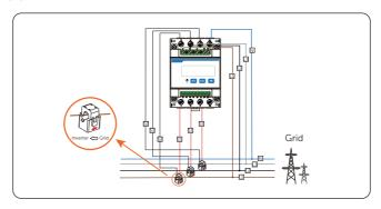
Figure 14-15 Connecting CT-connected meter to the grid
