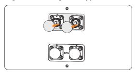
Figure 7-27 Removing battery caps
