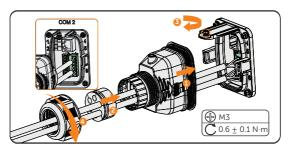
Figure 7-60 Connecting to the inverter
