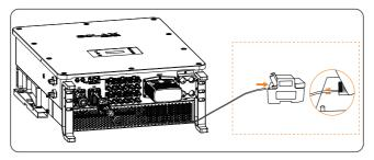
Figure 14-12 Connecting inverter to meter
