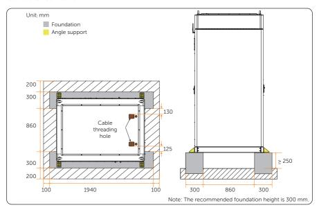
Figure 4-3 Foundation requirements for angle supports installed at front and rear sides
