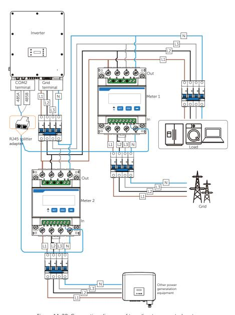
Figure 14-20 Connection diagram of two direct-connected meters
