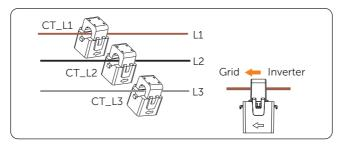
Figure 14-6 Clipping CTs to grid cables
