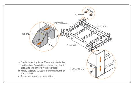
Figure 4-6 Detail description of steel foundation
