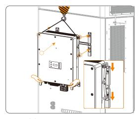
Figure 6-27 Hooking the inverter on the bracket
