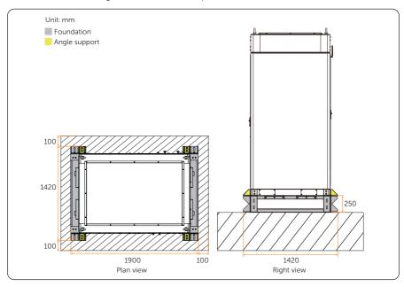
Figure 4-7 Angle supports at front and rear sides
