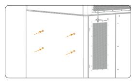
Figure 6-23 Confirming the position of the mounting bracket
