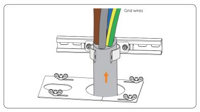
Figure 7-85 Threading grid wires
