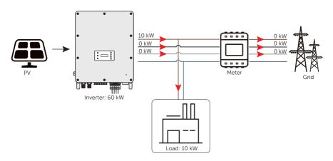
Figure 2-32 Zero export control with **Phase Unbalance** enabled
