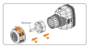
Figure 7-42 Disassembling the connector
