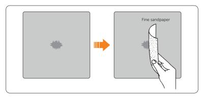
Figure 14-1 Sanding the scratched area
