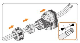
Figure 7-34 Threading the cables and striping the insulation
