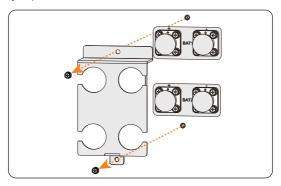
Figure 7-26 Removing the battery protective cover
