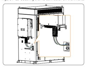
Figure 7-14 Well connected AC connector
