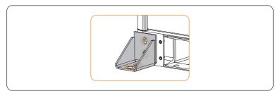
Figure 6-11 Aligning screw holes
