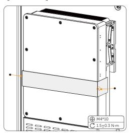
Figure 9-3 Securing the cover with the inverter
