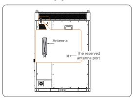
Figure 6-18 Installing an antenna
