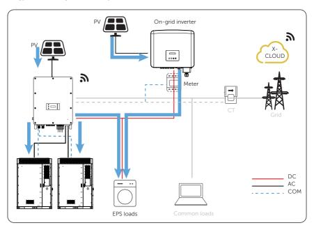
Figure 14-3 Power flowing when grid off
