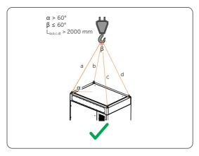
Figure 6-5 Proper way of hoisting
