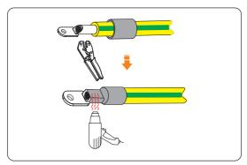
Figure 7-5 Crimping and heating
