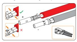
Figure 7-17 Crimping the terminal
