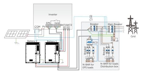
Figure 2-35 Partial load backup for Australia
