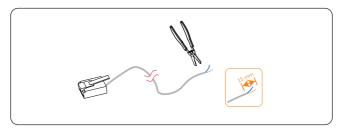
Figure 14-16 Stripping communication cable for meter
