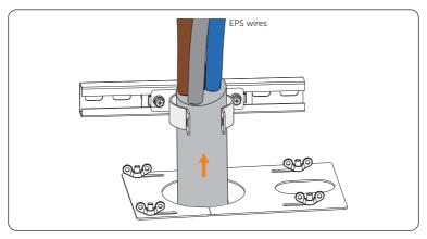
Figure 7-71 Threading grid wires
