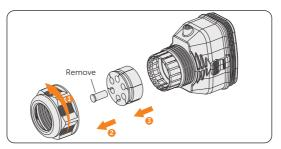
Figure 7-49 Disassembling the connector
