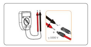
Figure 7-20 Measuring the voltage of PV connectors
