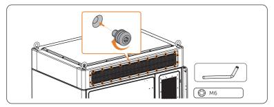
Figure 11-11 Tightening M6 screws
