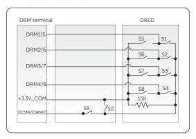
Figure 7-46 DRED connection diagram
