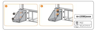
Figure 6-12 Tightening M12 screws
