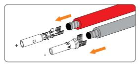
Figure 7-16 Inserting the PV pin contact
