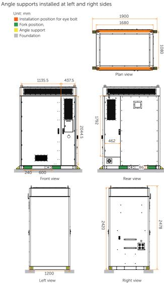
Figure 6-2 Dimension of battery cabinet
