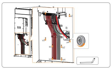
Figure 7-92 Unscrew M6 screws
