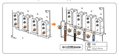
Figure 7-86 Connecting L1, L2, L3 and N wires
