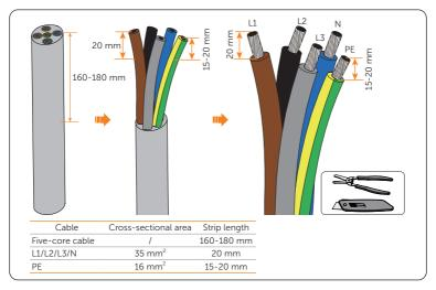
Figure 7-76 Striping cable jacket
