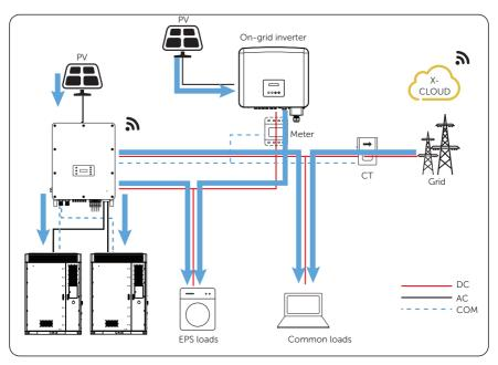
Figure 14-2 Power flowing when grid on and PV sufficient
