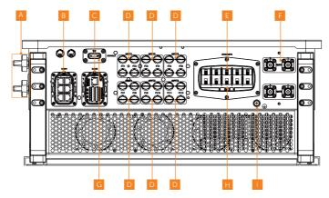
Figure 7-8 Terminals of Inverter
