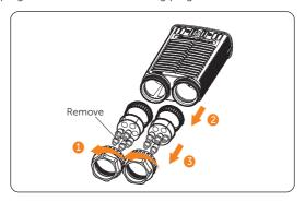
Figure 7-9 Disassembling the AC connector
