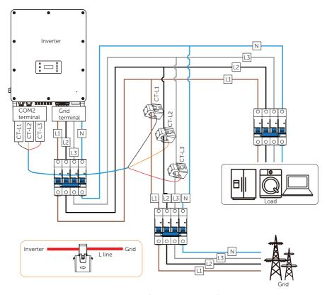
Figure 14-5 System wiring with CT
