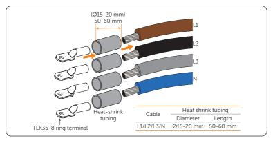
Figure 7-63 Slipping wires
