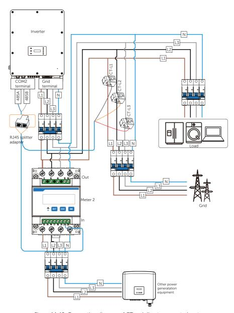
Figure 14-19 Connection diagram of CT and direct-connected meter
