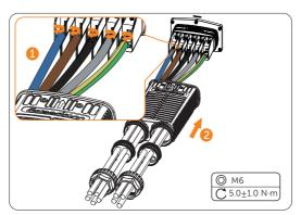
Figure 7-11 Connecting the Grid cable
