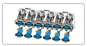
Figure 7-21 Connecting the PV cable
