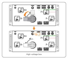
Figure 8-6 Starting the high-voltage box
