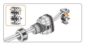
Figure 7-36 Installing the cable to the cable clamp
