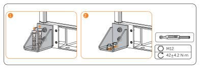
Figure 6-13 Tightening expansion bolts
