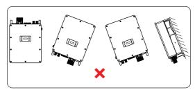
Figure 6-20 Incorrect installation
