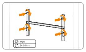
Figure 6-24 Securing the mounting bracket
