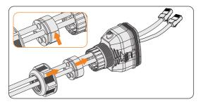
Figure 7-33 Threading the cables with RJ45 terminal
