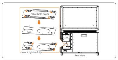
Figure 7-80 Unscrewing M5 butterfly nuts
