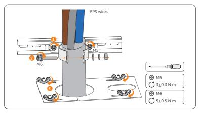
Figure 7-73 Tightening screws
