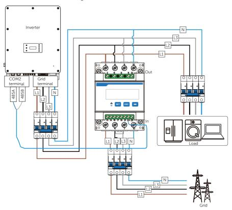
Figure 14-9 System wiring with direct-connected meter
