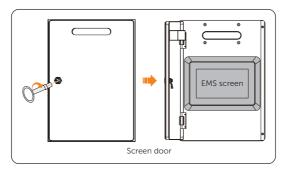
Figure 9-5 Unlocking screen door
