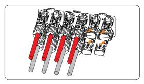
Figure 7-23 Installing PV dustproof buckles
