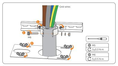
Figure 7-87 Tightening screws
