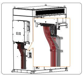
Figure 7-24 Well connected PV cables
