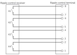
Figure 7-52 Connection diagram for ripple control
