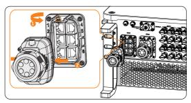
Figure 7-31 Removing the connector enclosure
