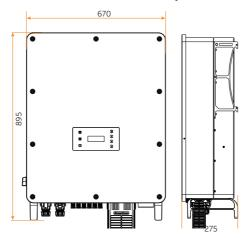
Figure 6-21 Dimensions (Unit: mm)
