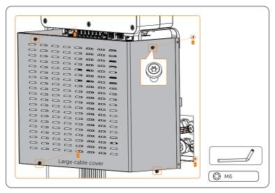
Figure 7-93 Attaching large cable cover
