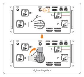
Figure 11-2 Shutting down the high-voltage box
