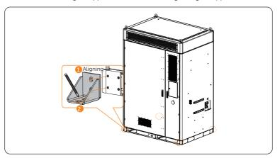
Figure 6-9 Marking hole position
