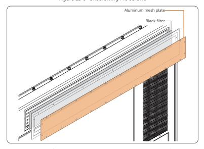
Figure 11-10 Dismantling aluminum mesh plate and black filter
