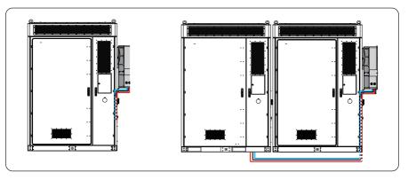
Figure 7-25 Inverter with battery cabinet(s)
