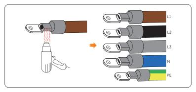
Figure 7-79 Heating heat-shrink tubing
