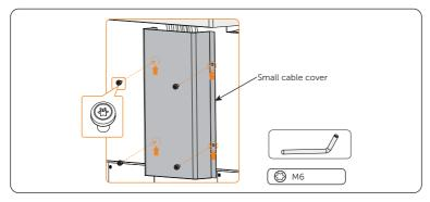
Figure 7-94 Attaching small cable cover
