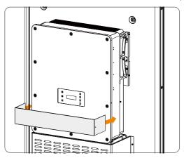
Figure 9-2 Putting the screen cover on the inverter
