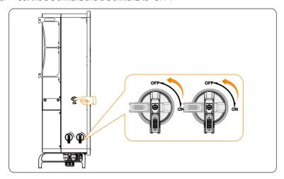
Figure 11-3 Shutting down the inverter
