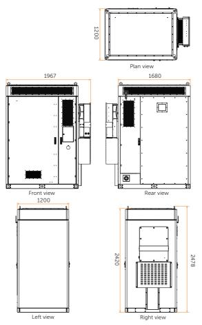
Figure 2-2 Dimension (unit: mm)
