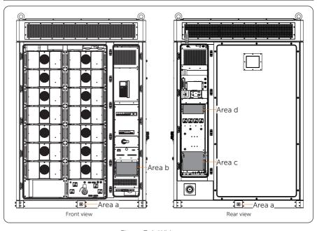
Figure 7-1 Wiring area
