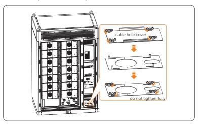
Figure 7-66 Unscrewing M5 butterfly nuts
