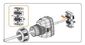
Figure 7-40 Installing RJ45 terminal to the cable clamp
