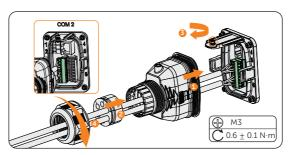
Figure 7-57 Connecting to the inverter
