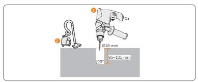
Figure 6-10 Drilling
