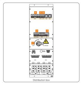
Figure 8-1 Starting sequence of distribution box
