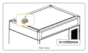
Figure 6-3 Unscrewing M20 screws
