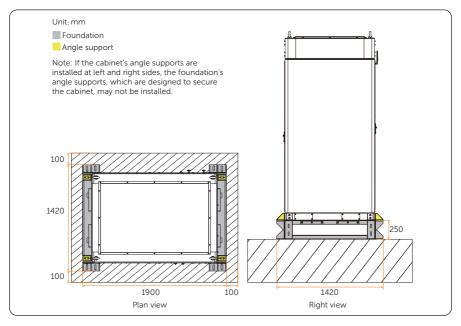
Figure 4-8 Angle supports at left and right sides
