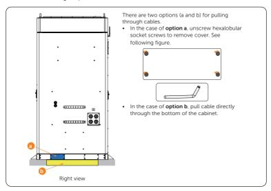
Figure 7-70 Threading EPS wires
