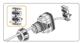
Figure 7-45 Installing RJ45 terminal to the cable fixture
