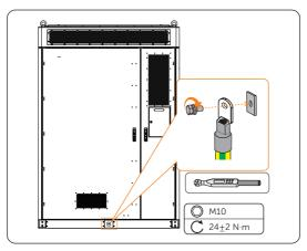
Figure 7-6 Tightening M12 screw
