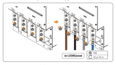
Figure 7-72 Connecting L1, L2, L3 and N wires
