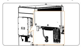
Figure 7-41 Well connected COM 1 cables
