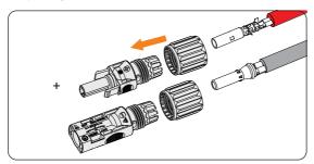
Figure 7-18 Threading the PV cable
