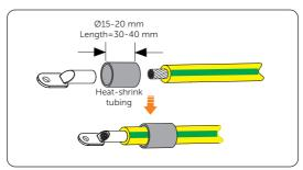
Figure 7-4 Cutting heat-shrink tubing
