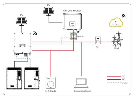
Figure 14-1 Micro-grid wiring connection
