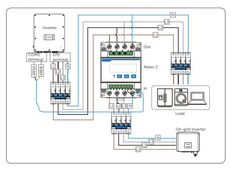
Figure 14-4 Connection diagram of Meter on EPS terminal
