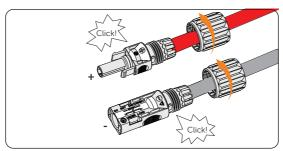
Figure 7-19 Securing the PV cable
