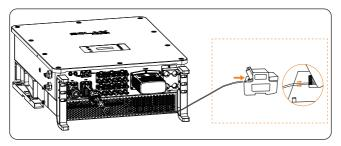
Figure 14-17 Connecting inverter to meter
