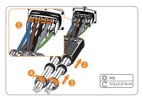
Figure 7-12 Connecting the EPS cable
