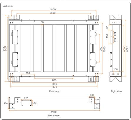
Figure 4-5 Dimension of steel foundation
