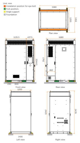
Figure 6-1 Dimension of battery cabinet
