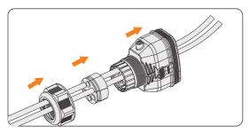
Figure 7-55 Threading the cables
