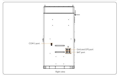
Figure 7-7 Prefabricated inverter cables in battery cabinet
