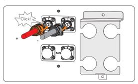
Figure 7-28 Connecting assembled battery cables
