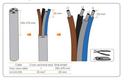
Figure 7-62 Striping cable jacket
