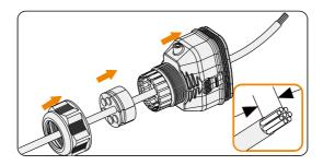
Figure 7-43 Threading the cables and striping the insulation
