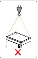
Figure 6-6 Improper way of hoisting
