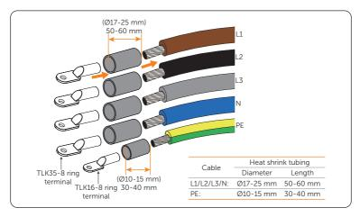
Figure 7-77 Cutting heat-shrink tubing
