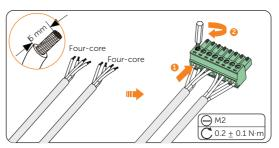
Figure 7-56 Connecting to 8-pin terminal block
