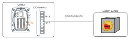
Figure 7-58 System switch connection diagram
