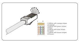
Figure 7-35 Crimping the communication cable
