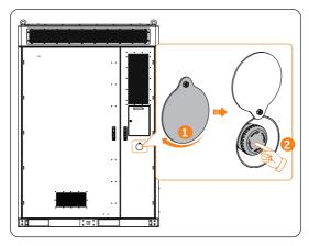
Figure 11-8 Pressing emergency stop button
