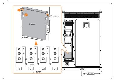
Figure 7-82 Removing cover
