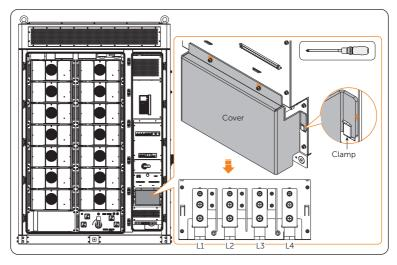
Figure 7-68 Removing cover
