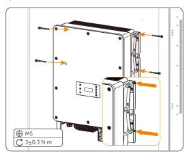
Figure 6-29 Securing the inverter
