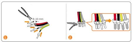
**Step 2:** Thread the crimping terminals into the ECC-PLC port according to cable variation.
