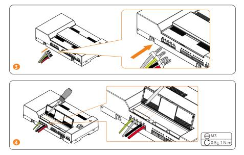
The graphics above shows the wiring steps of power cables in the split-phase. If you need to wire for the three-phase, please connect the corresponding cable to ECC-PLC according to the grid:
