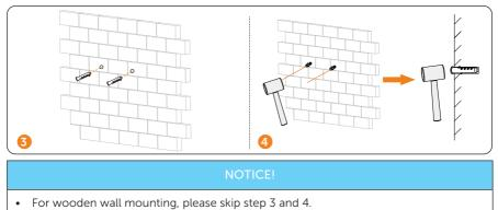
Step 4: Insert the expansion tubes in the holes.
