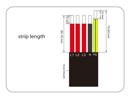
STEP 8: Insert the input cable through the waterproof connector in sequence as shown below.
