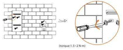
STEP 3: Hang the EV-Charger on the wall for trial, then estimate the required length of input cable and communication cable. After that, take the EV-Charger down.
