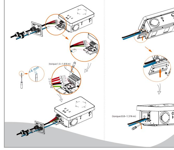
STEP 11: Push the rear cover to appropriate position of the cables and screw the self tapping screws with the cross screwdriver. Then tighten the waterproof fastening heads.
