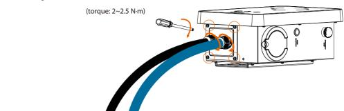
STEP 12: Hang the EV-Charger up carefully and steady the EV-Charger with the self tapping screw and the cross screwdriver.
