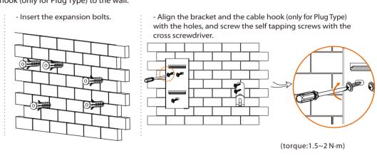
STEP 3: Hang the EV-Charger on the wall for trial, then estimate the required length of input cable (three-core for single-phase, five-core for three-phase, outer diameter: 12.5-18 mm) and communication cable. After that, take the EV-Charger down.
