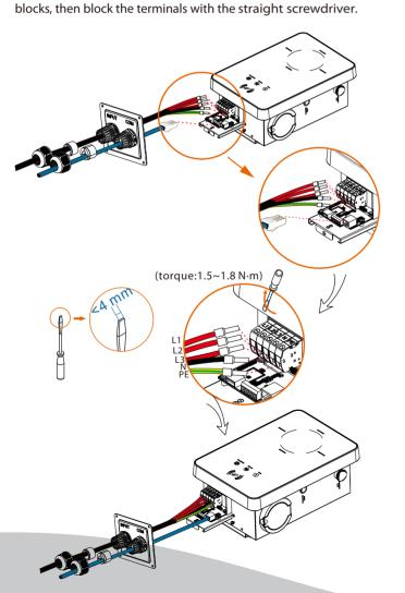
STEP 10: Press the spring upward and push the base plate of communication board in. Then screw the countersunk screw.
