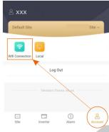
\*If manual WiFi configuration is required, the IP address is http://192.168.10.10/.
