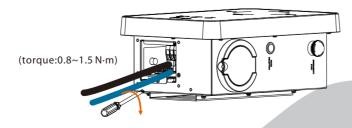
STEP 11: Push the rear cover to appropriate position of the cables and screw the self tapping screws with the cross screwdriver. Then tighten the waterproof fastening heads.
