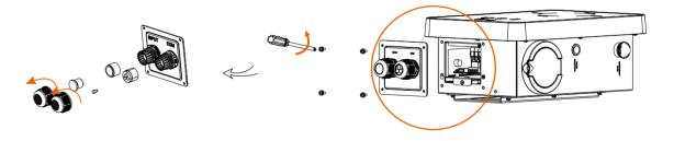
STEP 5: Unscrew the countersunk screw of the base plate of communication board with the cross screwdriver. Then pull the base plate of communication board out.
