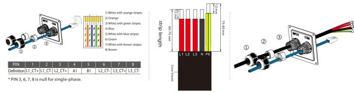
STEP 9: Insert the wires into the appropriate holes of the terminal
