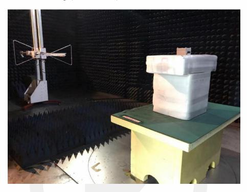
Spurious Emission Test Setup (Above 1GHz)
