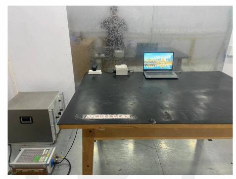
20.1.Photos of Conducted Emissions from the AC Mains Power Ports
