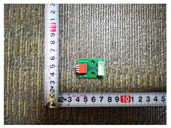
Dip switch board (Top view)
