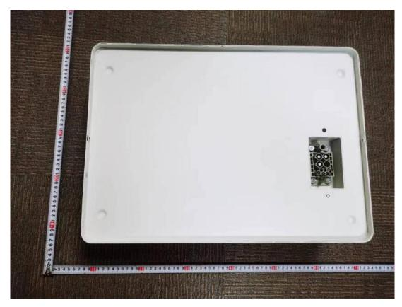
Battery module, Model: TP-HS36, (bottom view)
