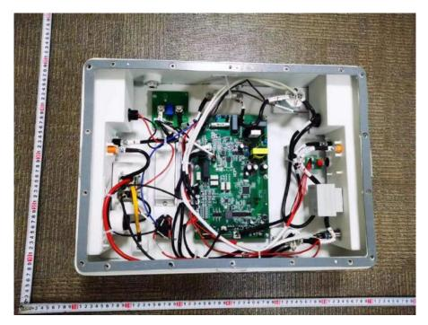
Inside of Main control unit, Model: TBMS-MCS0800
