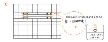
d) Hang the BI PRO on the bracket. Please make sure the cleat is well seated on the bracket.
