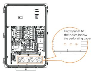
b) Drill the hole with a hole cutter. Choose 1 inch or 2 inch size (Metal chips must be cleaned after drilling).
