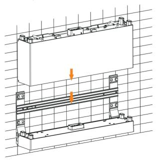
f) Mount the fixing plate (2 holes) [TP-HS50 (part G)] using M5\*10 cross screw [TP-HS50 (part E)], and secure M5\*10 screws (2 for each side) to connect Base and Battery Module.
