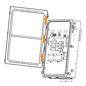
**Step 4:** Remove the dead front by unscrewing the seven screws with a screwdriver.
