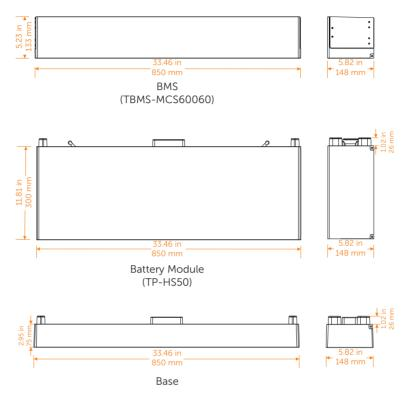
Figure 4-2 Dimensions of battery
