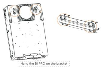
e) Secure the BI PRO by screwing in the tapping screw with washer on the bottom of BI PRO.
