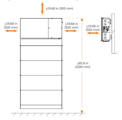
For multi-inverter installation, please reserve the space of 19.68 inch (500 mm) at least between each left and right inverter and at least 19.68 inch (500 mm) distance from the ceiling . If multiple inverter are mounted in areas with high ambient temperatures, increase the clearances between the inverter and batteries and ensure an adequate fresh-air supply if possible.
