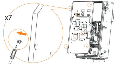
Unscrew the metal cover where circuit breakers are to be installed.
