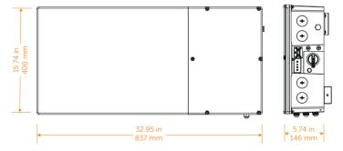
Figure 4-1 Dimensions of inverter
