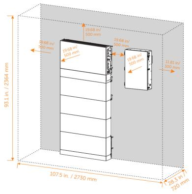
Recommend installation space: (W\*D\*H) 107.5 in. \* 28.3 in. \* 93.1 in. / 2730 mm \* 720 mm \* 2364 mm
