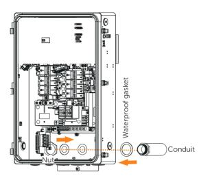
d) The top of the nut and contact surface of the threads must be cleaned after locking the nut, as well as the contact surface between the nut and the box.
