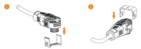
**Step 3:** Disconnect the series wiring terminal on the battery.
