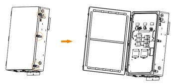
**Step 2:** Unscrew the seven M4 screws below with crosshead screw driver to disassemble the internal cover of BI PRO.
