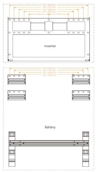
To ensure good heat dissipation and convenient disassembly of the inverter and battery, the minimum clearance around the inverter and battery shall not be less than the following values, as shown below. The height above the ground marked below is recommended assuming that four BATs are installed with floor-mounting.
