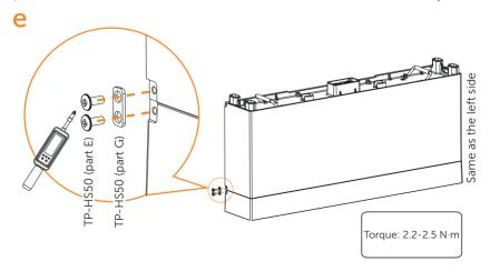
f) Place two battery modules in turn, and secure both left and right sides with screws (4×M5\*10 countersunk screw).
