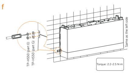
g) Place two battery modules in turn, and secure both left and right sides with screws  $(4\times M5*10 \text{ countersunk screw})$ .
