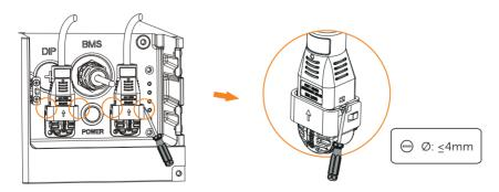
**Step 2:** (Optional) Reinstall and secure the buckles to the BAT cables. (1) Align the curve of the cable head to that of the buckle, and then stick the cable head into the buckle base.
