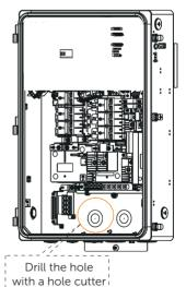
Choose 1 inch or 2 inch size (Metal chips must be cleaned after drilling)
