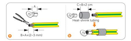
c) Crimp it with crimping tool, pull the heat-shrink tubing over the stripped section of the grounding terminal and use a heat gun to shrink it so that it can be firmly contacted with the terminal;
