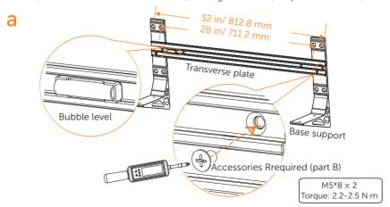
Studs spaced at 12, 20 and 24 inch: secure the transverse plate and base support using screws ( $2 \times M5*8$  countersunk head screw), and tighten them. See figure below.
