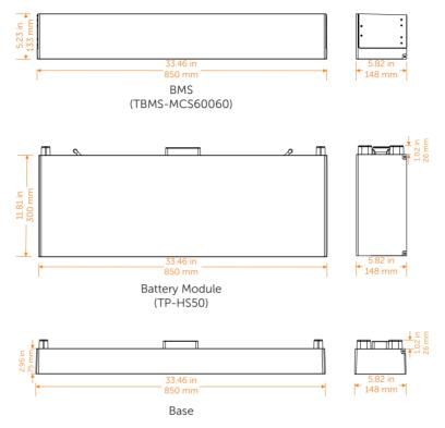
Figure 4-2 Dimensions of battery
