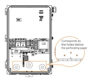
b) Drill the hole with a hole cutter. Choose 1 inch or 2 inch size (Metal chips must be cleaned after drilling).
