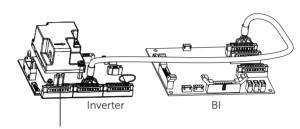
120-Ohm terminating resistor
