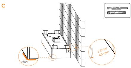
d) Manual-remove the top and bottom dust cover of the battery module and catch hold of the handle to stack the battery module to the base. Make sure that each connecting pole of the battery module or base is well pluged into the slot of the next battery module which is on the bottom of the module.
