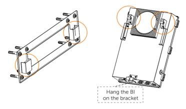
e) Secure the BI by screwing in the tapping screw with washer on the bottom of BI.
