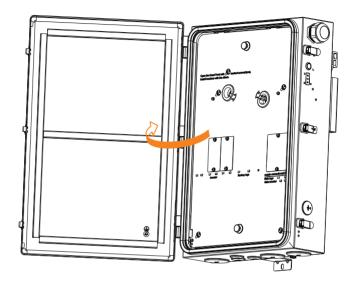
**Step 3:** Remove the door upwards.
