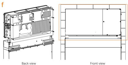
g) Place the protective guard [Inverter (part F)] on the correct position of battery's BMS prior to the wiring connection between inverter and battery and fix it with the inverter bracket with M5 screws [Inverter (part C)].
