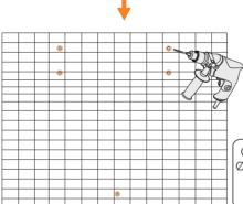
Ø4 drill for wooden wall Ø10 drill for concrete wall Depth: 2.16 in / 55 mm
