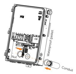
d) The top of the nut and contact surface of the threads must be cleaned after locking the nut, as well as the contact surface between the nut and the box.
