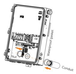
d) The top of the nut and contact surface of the threads must be cleaned after locking the nut, as well as the contact surface between the nut and the box.
