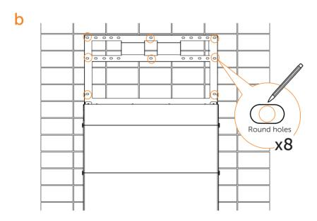
c) Unscrew the two M4 screws to disassemble the bracket. Drill holes with power drill, and make sure the holes are deep enough (2.16 in / 55 mm) to support the inverter.
