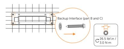
d) Hang the BI on the bracket. Please make sure the cleat is well seated on the bracket.
