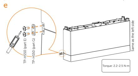
f) Place two battery modules in turn, and secure both left and right sides with screws  $(4\times M5*10 \text{ countersunk screw})$ .
