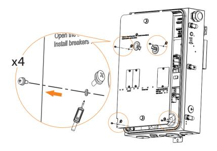
Unscrew the metal cover where circuit breakers are to be installed.
