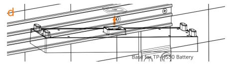
(2) Place Base on the Base Support and secure both left and right sides with screws (4  $\times$  M5\*20 countersunk screw) [Accessories Rrequired (part C)] (Torque: 2.2-2.5 N·m).
