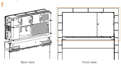
g) Place the protective guard [Inverter (part F)] on the correct position of battery's BMS prior to the wiring connection between inverter and battery and fix it with the inverter bracket with M5 screws [Inverter (part C)].
