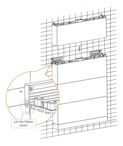
I) Fix the fixing plate (3 holes) [TP-HS50 (part F)] on both sides of battery module using M5\*10 cross screw [TP-HS50 (part E)], and then tighten M5\*10 screws.
