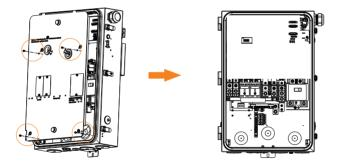
**Step 3:** Disconnect the fan cable, and unscrew the two M4 screws to disassemble the fan (pull out the fan).
