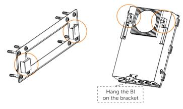
e) Secure the BI by screwing in the tapping screw with washer on the bottom of BI.
