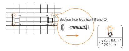
d) Hang the BI on the bracket. Please make sure the cleat is well seated on the bracket.
