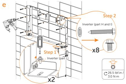
f) Place the inverter to be seated on the corresponding position of the bracket. As A1-HYB-G2 series inverters are heavy, weigh 75 lbs / 34 Kg. They should be lifted up by two persons and placed carefully onto the bracket. Then adjust the inverter to be centered on the whole system;
