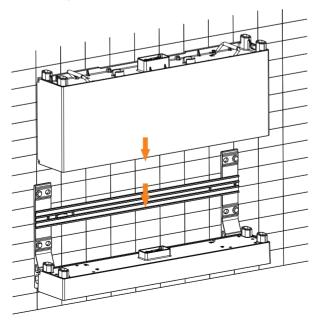
f) Mount the fixing plate (2 holes) [TP-HS50 (part G)] using M5\*10 cross screw [TP-HS50 (part E)], and secure M5\*10 screws (2 for each side) to connect Base and Battery Module.
