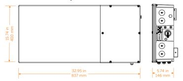
Figure 4-1 Dimensions of inverter
