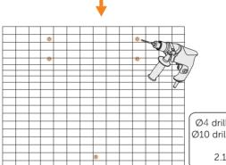
Ø4 drill for wooden wall Ø10 drill for concrete wall Depth: 2.16 in / 55 mm
