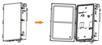
**Step 2:** Unscrew the four M4 screws below with crosshead screw driver to disassemble the internal cover of BI.
