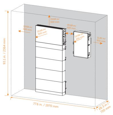
Recommend installation space: (W\*D\*H) 77.6 in. \* 28.3 in. \* 93.1 in. / 1970 mm \* 720 mm \* 2364 mm
