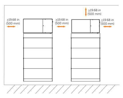
To ensure good heat dissipation and convenient disassembly of the BI, the minimum clearance around the BI shall not be less than the following values, as shown below.
