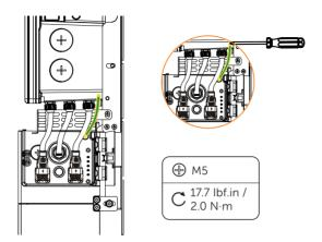
For easier connection, please connect the grounding conductor on the BMS first.
