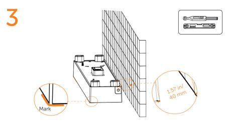
Step 2 Mount the battery module
