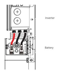
Connection between inverter and battery
