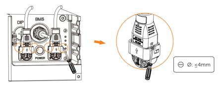
**Step 2:** (Optional) Reinstall and secure the buckles to the BAT cables.
