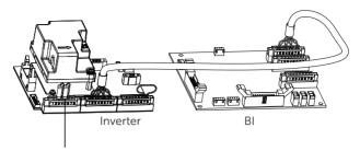
120-Ohm terminating resistor
