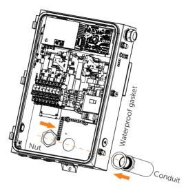
d) The top of the nut and contact surface of the threads must be cleaned after locking the nut, as well as the contact surface between the nut and the box.
