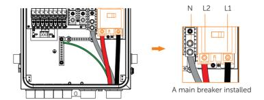
For the specific requirement of cable and torque, please refer to "Appendix A: Wiring and Breaker Requirement".
