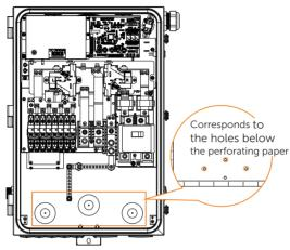
b) Drill the hole with a hole cutter. Choose 1 inch or 2 inch size (Metal chips must be cleaned after drilling).
