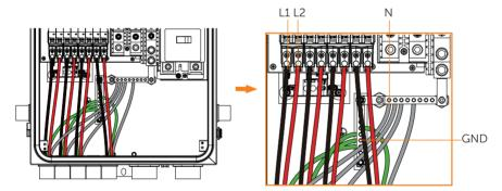
• Connect the load conductors to BI
