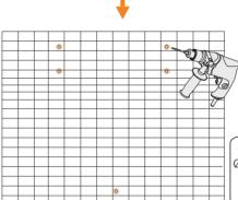
Ø4 drill for wooden wall Ø10 drill for concrete wall Depth: 2.16 in / 55 mm
