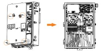
**Step 3:** Disconnect the fan cable, and unscrew the two M4 screws to disassemble the fan (pull out the fan).
