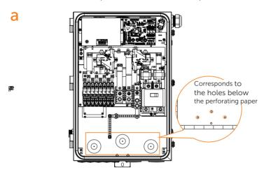
b) Drill the hole with a hole cutter. Choose 1 inch or 2 inch size (Metal chips must be cleaned after drilling).
