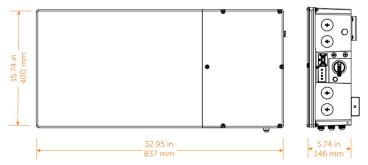
Figure 4-1 Dimensions of inverter
