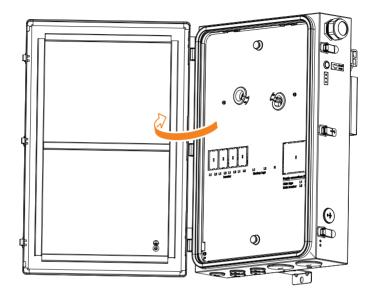
**Step 3:** Remove the door upwards.
