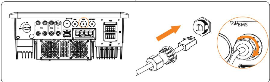
\* Note: It is recommended that the BMS communication cables between the inverter and the battery be no more than 3 meters.
