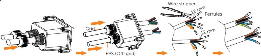
3 After threading through cables, lightly tighten waterproof screws in case of their falling down.
