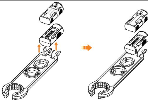
Disassembling the PV cables
