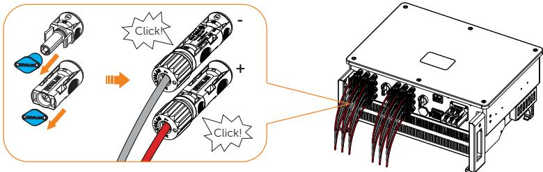
\* Seal the unused PV terminals with the dustproof buckles from the accessory.
