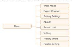
Work Mode: Select the working mode of the inverter, including Work mode for Pakistan: SUB, SBU, MKS and Force Time Use and Work mode for other countries: BackUp, Self Consumption and Force Time Use.
