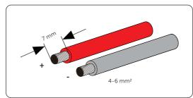
**Step 1:** Strip off the insulation of the PV cables to an appropriate length.
