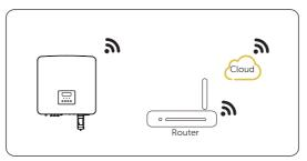
Figure 8-54 Wi-Fi mode connection diagram
