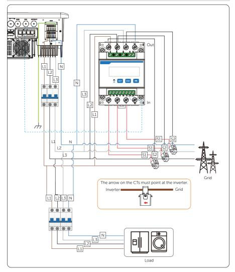
Figure 15-30 System wiring with CT-connected meter
