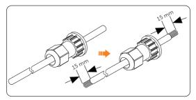
Figure 8-43 Stripping the insulation
