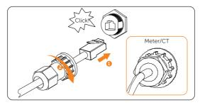
Figure 8-45 Connecting to inverter Meter/CT terminal
