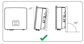
Figure 7-1 Correct installation
