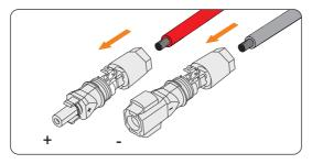
Figure 8-25 Inserting the battery connector
