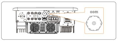
Figure 15-8 Connection terminal for EV-Charger
