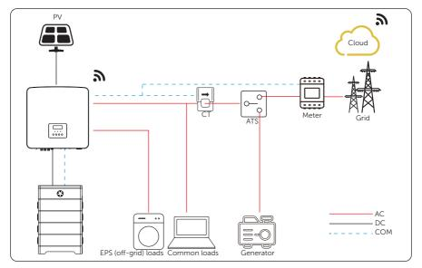
Figure 15-1 ATS control wiring diagram
