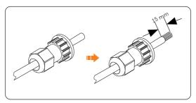
Figure 8-31 Stripping the insulation
