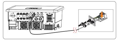
Figure 15-9 Connecting to EV-Charger
