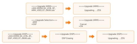
e. After the upgrade is completed, the LCD screen displays **Upgrade Successful**. If the upgrades fail, the LCD screen displays **Upgrade failed**.
