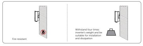
Figure 5-3 Installation carrier requirement
