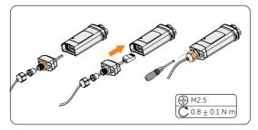
Figure 8-59 Assembling the dongle
