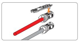
Figure 13-2 Disconnecting the PV connector
