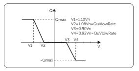
Figure 10-6 Curve Q = f(V)
