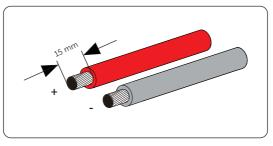
Figure 8-24 Stripping the battery cable
