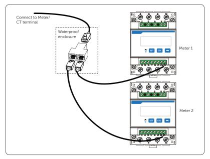
Figure 15-39 Connecting to RJ45 splitter adapter
