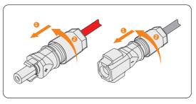
Figure 8-28 Tightening the cable grand
