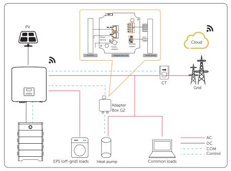
Figure 15-4 Adapter Box G2 wiring diagram
