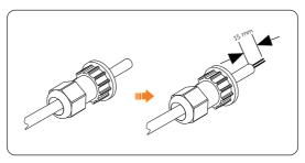
Figure 8-38 Stripping the insulation
