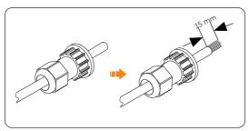
Figure 8-35 Stripping the insulation
