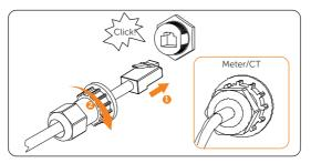
Figure 8-40 Connecting to inverter Meter/CT terminal
