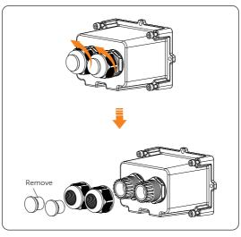
Figure 8-10 Disassembling the AC protective cover
