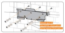
Figure 7-8 Securing the bracket
