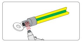
Figure 8-6 Shrinking the tubing
