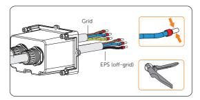
Figure 8-12 Crimping the conductors
