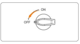
Figure 13-1 Turning off the DC switch
