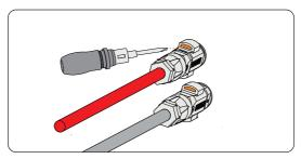
Figure 13-3 Disconnecting the battery connector
