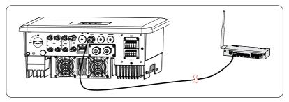
Figure 15-12 Connecting to DataHub
