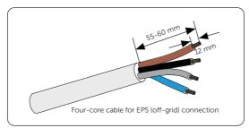
Figure 8-9 Stripping the EPS (off-grid) cable
