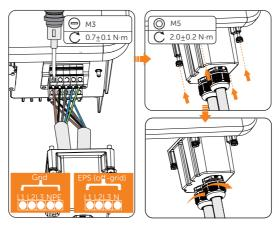
Figure 8-14 Installing the AC protective cover
