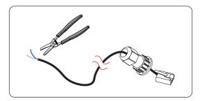
Figure 15-33 Stripping communication cable for meter
