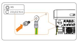
Figure 8-7 Securing the PE cable
