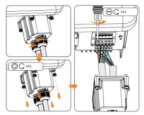
Figure 13-4 Disconnecting the AC connector
