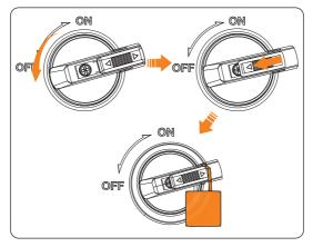
Figure 9-8 Locking the DC switch
