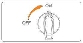
Figure 9-1 Turning on the DC switch
