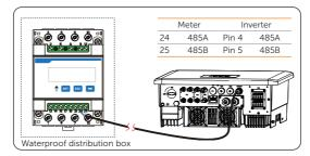
c. Connect the conductors to terminal 24 and 25 of the meter.
