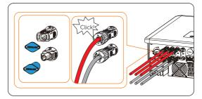
Figure 8-22 Connecting the PV cable
