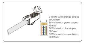
Figure 8-44 Crimping the network cable
