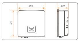
Figure 7-3 Dimensions 1 (Unit: mm)
