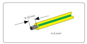
**Step 1:** Strip off the insulation of the PE cable to an appropriate length.
