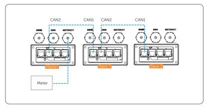
Figure 15-18 Communication wiring without X3-PBOX device
