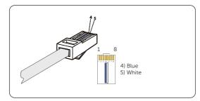
Figure 8-39 Crimping the network cable
