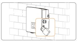
Figure 7-11 Locking the inverter
