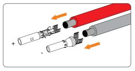
Step 2: Insert the stripped cable into the PV pin contact (part K and M).
