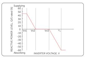
For Q(u), the curve required for the volt-var control mode can be referred to the below.
