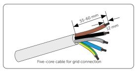
Figure 8-8 Stripping the Grid cable
