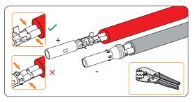
Figure 8-18 Crimping the terminal
