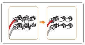
Figure 8-23 Installing the dustproof buckles
