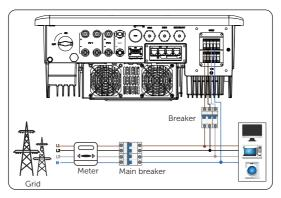
Figure 9-2 Switching on the AC breaker
