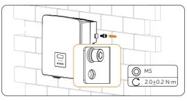
Figure 7-10 Securing the inverter
