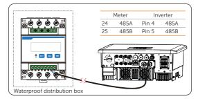
e. Connect the conductors to terminal 24 and 25 of the meter.
