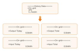
EPS: A record of the output electric energy of the inverter totay and the total, when it is disconnected from grid (through EPS (off-grid) connection terminal).
