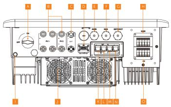
Figure 8-1 Terminals of Inverter
