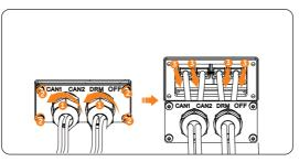
Figure 13-6 Disconnecting the CAN1 / CAN2 / DRM / OFF cable
