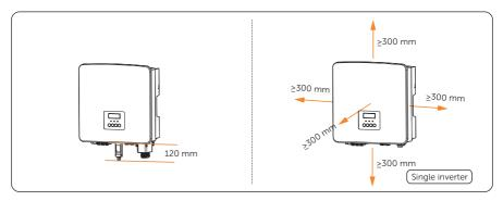
Figure 5-4 Clearance requirement for single inverter
