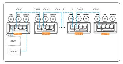
Figure 15-16 Communication wiring with X3-PBOX device
