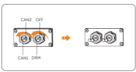
Figure 8-49 Removing the sealing plugs
