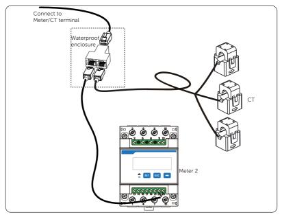
Figure 15-42 Connecting to RJ45 splitter adapter
