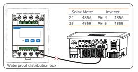
Figure 8-41 Connecting to Solax Meter
