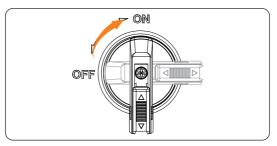
Figure 9-6 Turning on the DC switch
