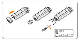
Figure 8-56 Assembling the dongle
