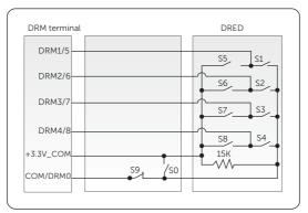
Figure 8-47 DRED connection diagram
