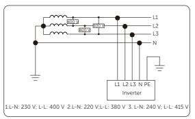
Figure 2-2 Supported power grid-TT
