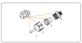
Figure 8-58 Disassembling the waterproof connector
