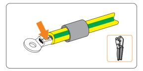
Figure 8-5 Crimping the cable
