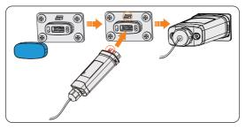
Figure 8-60 Connecting to the inverter
