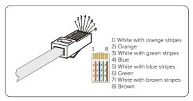
Figure 8-51 Crimping the communication cable
