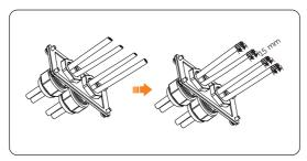
Figure 8-50 Threading and striping the cable
