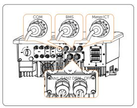
Figure 8-30 The completed communication connection
