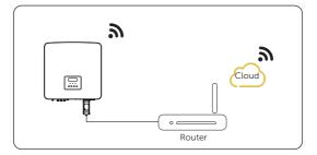
Figure 8-55 LAN mode connection diagram
