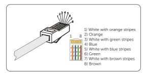
Figure 8-36 Crimping the network cable
