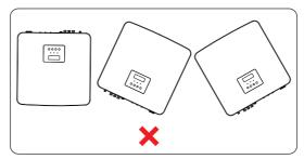
Figure 7-2 Incorrect installation
