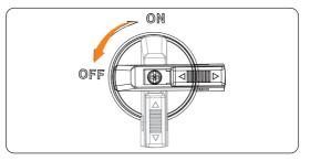
Figure 9-7 Turning off the DC switch
