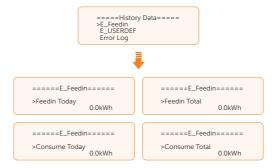
• **E\_USERDEF**: The output electricity of the connected on-grid inverter totay and the total (detected by Meter 2). This function is only available when meter 2 is connected.
