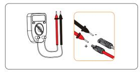
Figure 8-21 Measuring the voltage of PV connectors
