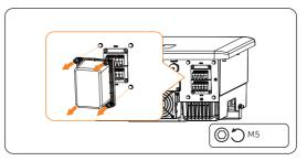
Figure 8-13 Removing the dustproof cover
