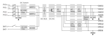
Figure 2-5 Circuit Diagram for X3-Hybrid G4 series inverter
