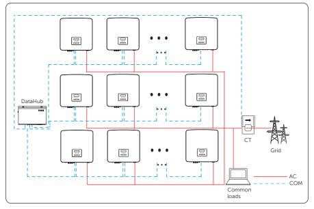
Figure 15-10 DataHub wiring diagram
