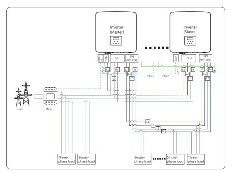
Figure 15-14 Without X3-PBOX-150kW-G2 system wiring diagram
