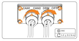
Figure 8-53 Securing the cables
