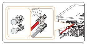
Figure 8-29 Connecting the battery connector
