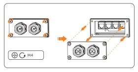
Figure 8-48 Disassembling the cover
