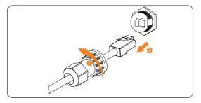
Figure 13-5 Disconnecting the COM / BMS / Meter / CT cable
