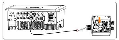
Figure 15-6 Connecting to Adapter Box G2
