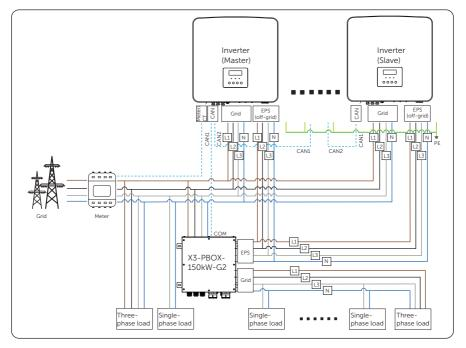
Figure 15-13 With X3-PBOX-150kW-G2 system wiring diagram
