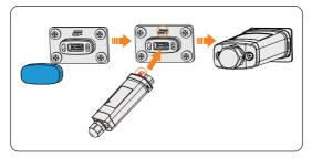
Figure 8-57 Connecting to the inverter
