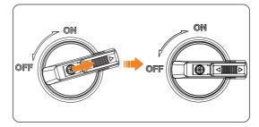
Figure 9-9 Unlocking the DC switch
