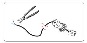
Figure 15-28 Stripping communication cable for meter
