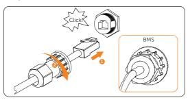
Figure 8-37 Connecting to BMS terminal
