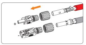
Figure 8-19 Threading the PV cable
