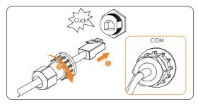
Figure 8-33 Connecting to COM terminal
