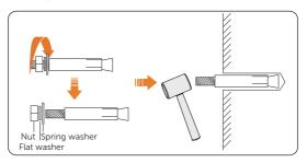
Figure 7-7 Disassembling the expansion set
