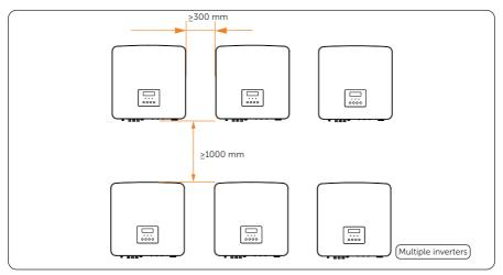
Figure 5-5 Clearance requirement for multiple inverters
