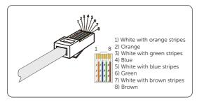
Figure 8-32 Crimping the network cable
