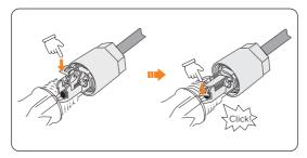
Figure 8-27 Pressing down the spring
