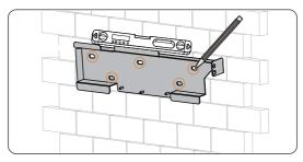
Figure 7-5 Marking the holes
