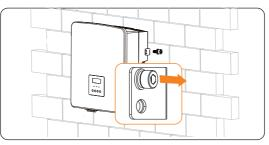
Figure 13-7 Unscrewing the M5 screws
