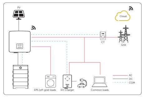
Figure 15-7 EV-Charger wiring diagram
