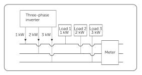
Figure 10-8 Phase Unbalanced enabled
