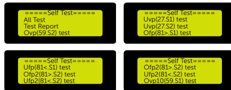
Figure 9-52 Setting to do tests
