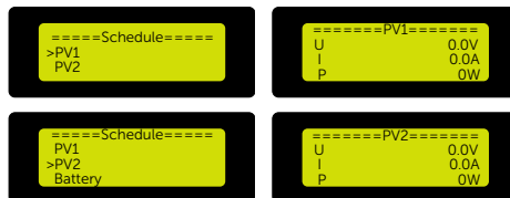
Figure 9-14 Displaying PV1 and PV2 status
