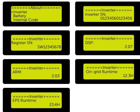
Figure 9-103 Displaying the inverter information
