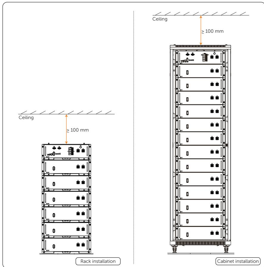
\*Note: It is recommended to install the device against the wall.
