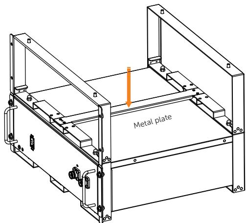
Gently place the battery into the rack, and tighten 4 M6 screws
