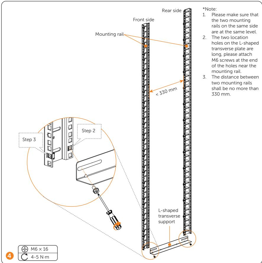
After all L-shaped transverse plate are secured, attach the assembled mounting rails into the cabinet, and tighten screws to fasten mounting rail and fix rail.
