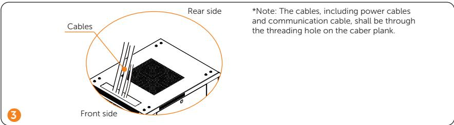
\*Note: The cables, including power cables and communication cable, shall be through the threading hole on the caber plank.
