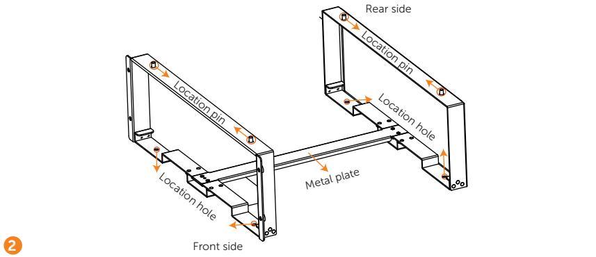
Gently place the battery into the rack, and tighten 4 M6 screws
