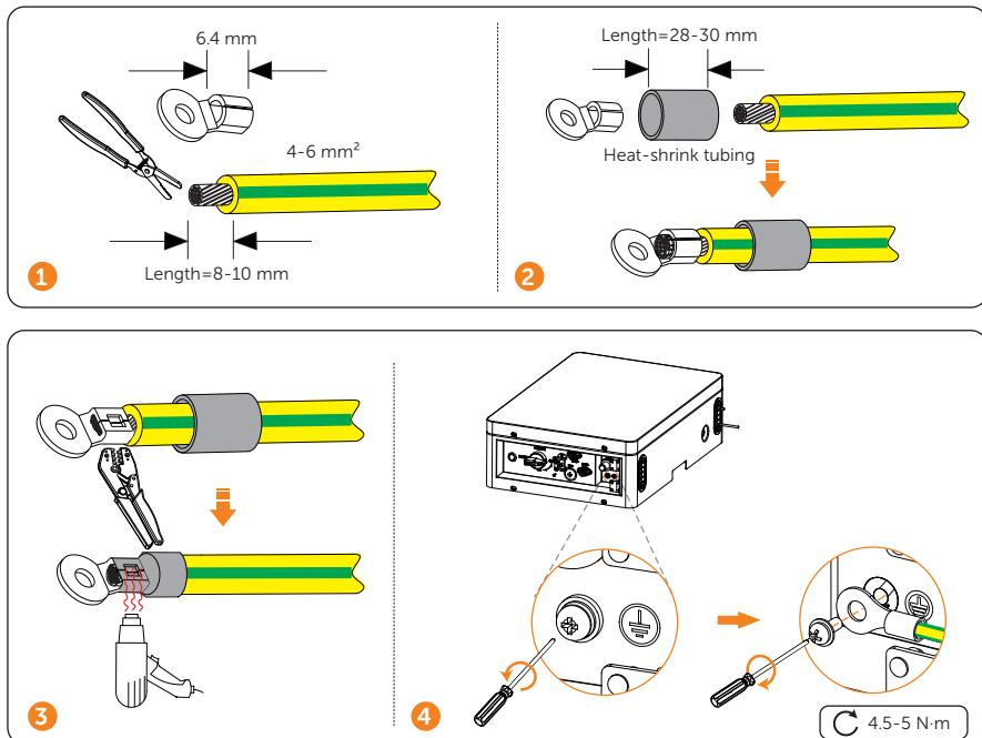
In case of a rated current of 30 A, the wire size of 5.5-6.5 mm<sup>2</sup> for cables (including grounding cable) is recommended; in case of a rated current of 45 A, the wire size of 8.5-9.5 mm<sup>2</sup> for cables (grounding cable) is recommended.
