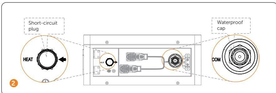
\*Note: In case of one tower, a waterproof cap shall be put on the unconnected "COM" port, as well as a short-circuit plug on the unconnected "HEAT" port.
