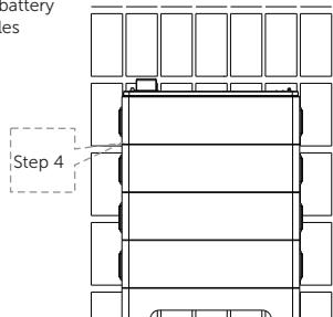
Attach M6 Flange nut but not tighten
