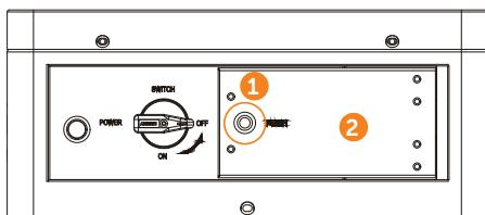
1. Remove the screws on both covers of the BMS.
