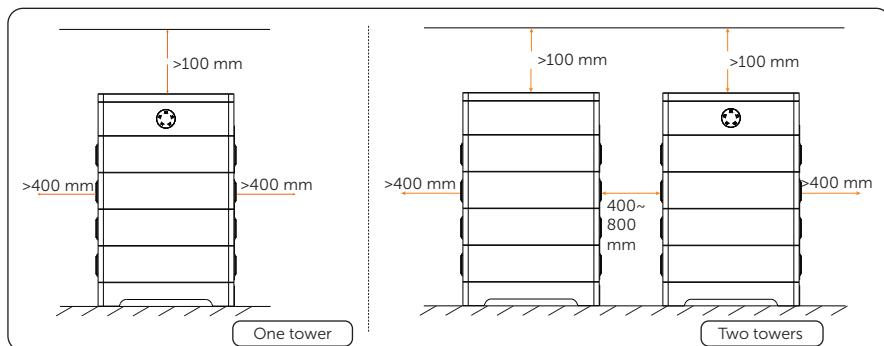
\*Note: The above figure shows an example of installation space of "One Tower" and "Two Towers".
