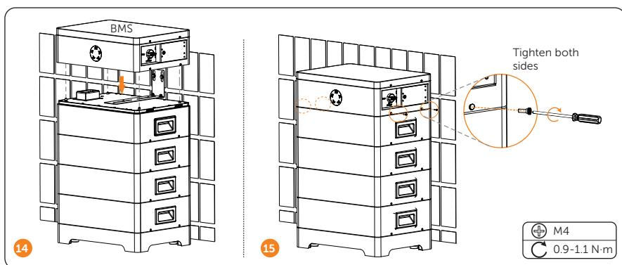
\*Note: Regarding the cover plate on both sides of the BMS, they should be installed after finishing wiring.
